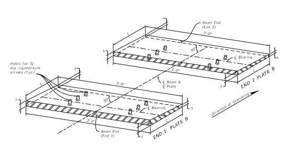
ISOMETRIC VIEW OF BEVELED BEARING PLATES (TYPE 2) FOR FLORIDA I-BEAMS
