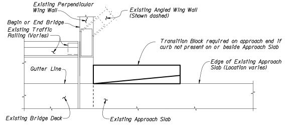
PARTIAL PLAN VIEW OF EXISTING BRIDGE WITH PERPENDICULAR OR ANGLED WING WALLS
