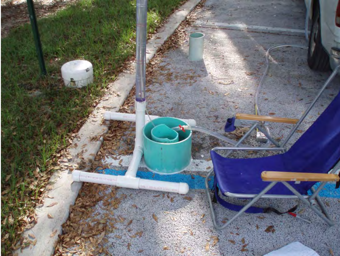
Figure 4 - Embedded Ring Infiltrometer Kit Showing On-Site Measurement
