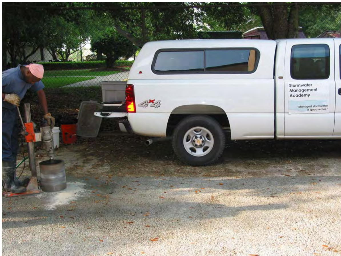
Figure 22: FDEP Parking Lot Core Test
