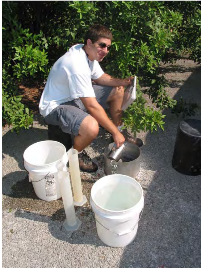
Figure 9: Pervious Concrete Pavement Core Test
