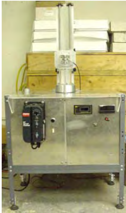
Figure 1. Photograph of Rotating Erosion Test Apparatus (RETA).
