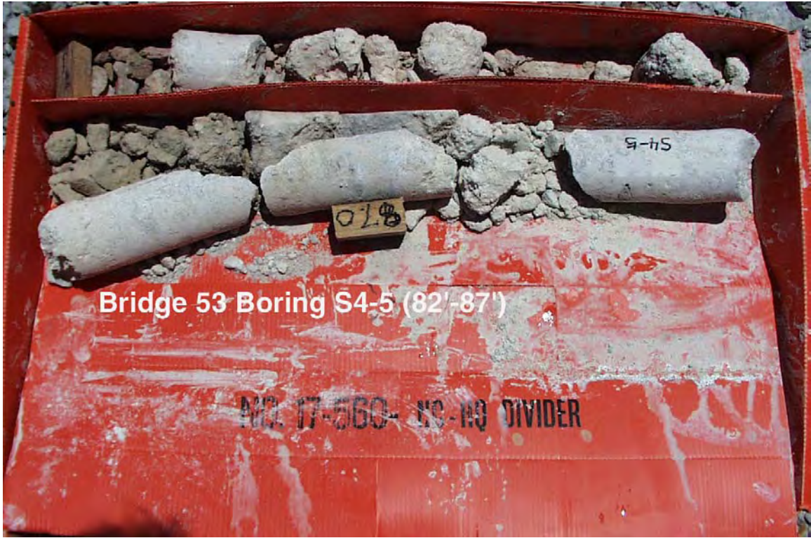
Figure B17. Photograph of core samples from Borehole S4-5.
