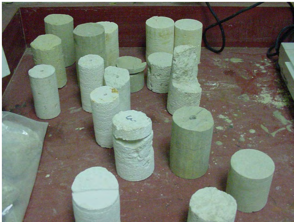
Above: Picture of trial test samples using the new cutting and drilling procedures
