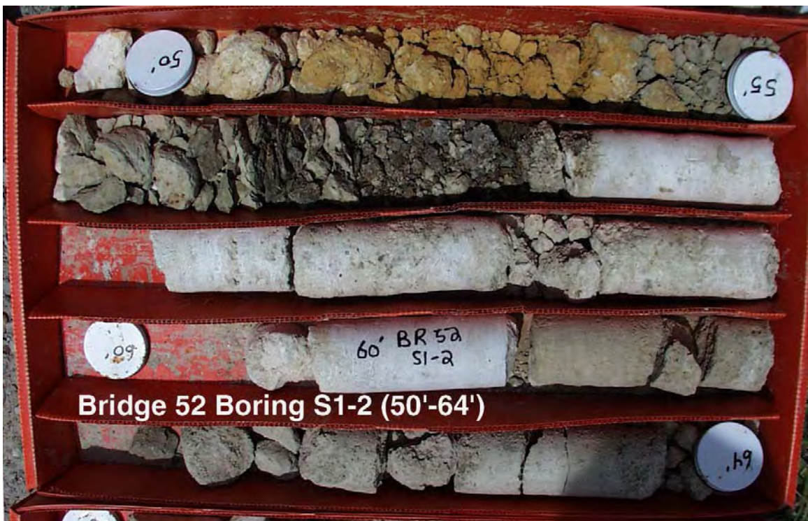
Figure B2. Photograph of core samples from Borehole S1-2.
