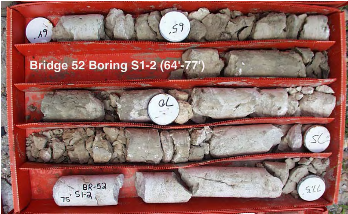
Figure B3. Photograph of core samples from Borehole S1-2.
