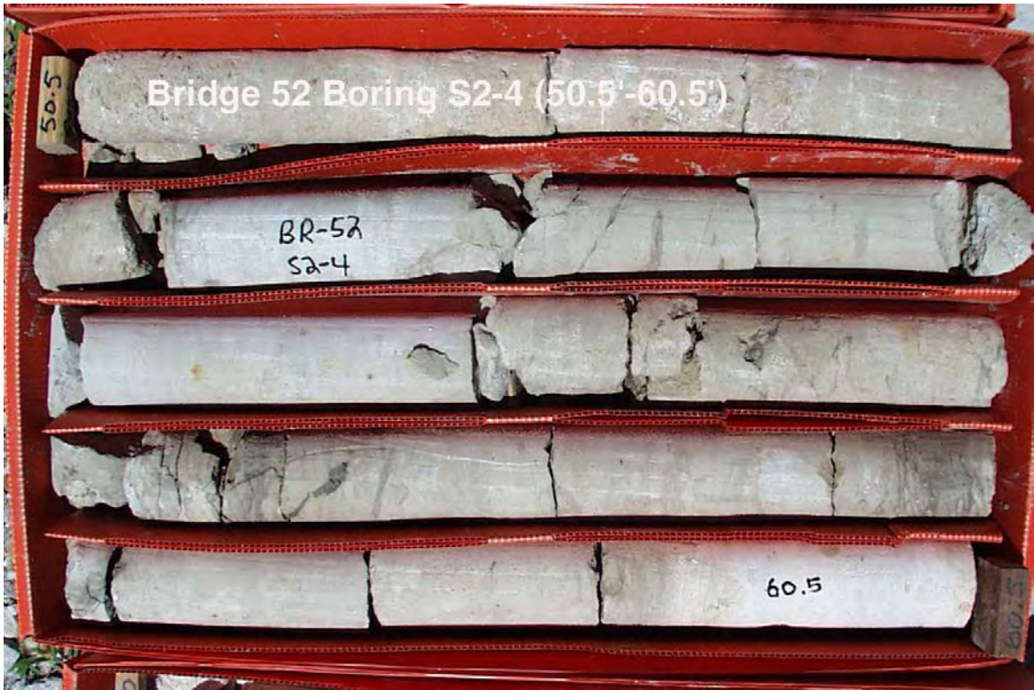
Figure B7. Photograph of core samples from Borehole S2-4.
