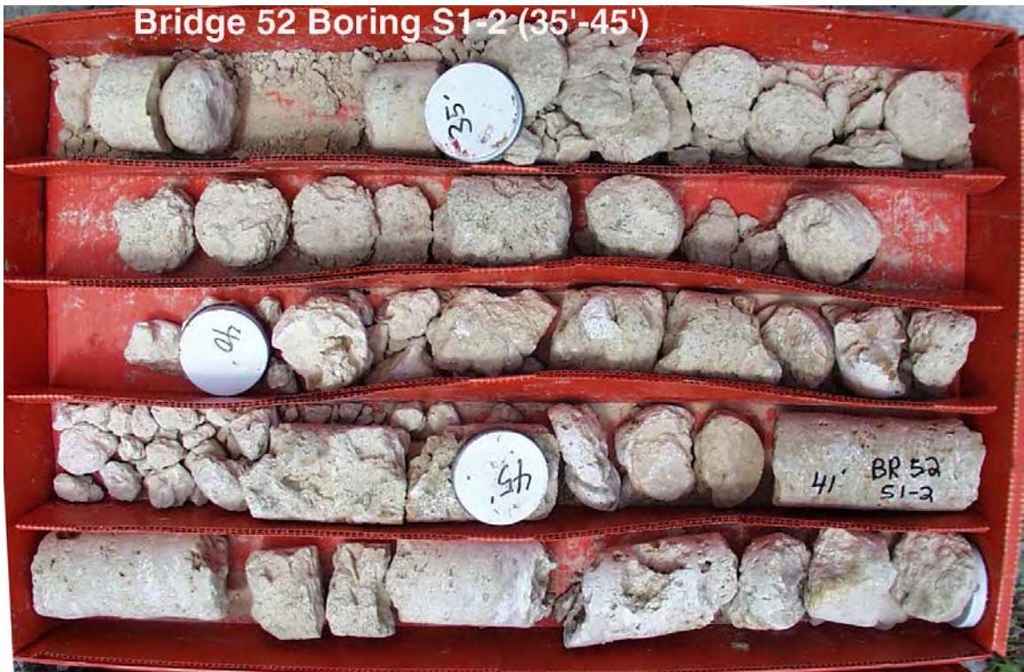
Figure B1. Photograph of core samples from Borehole S1-2.
