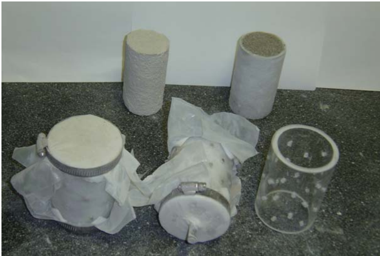
Figure A-10 From front left to right: cemented sand molds for the SERF, the RETA, and an empty mold. Extracted samples are seen at the back.
