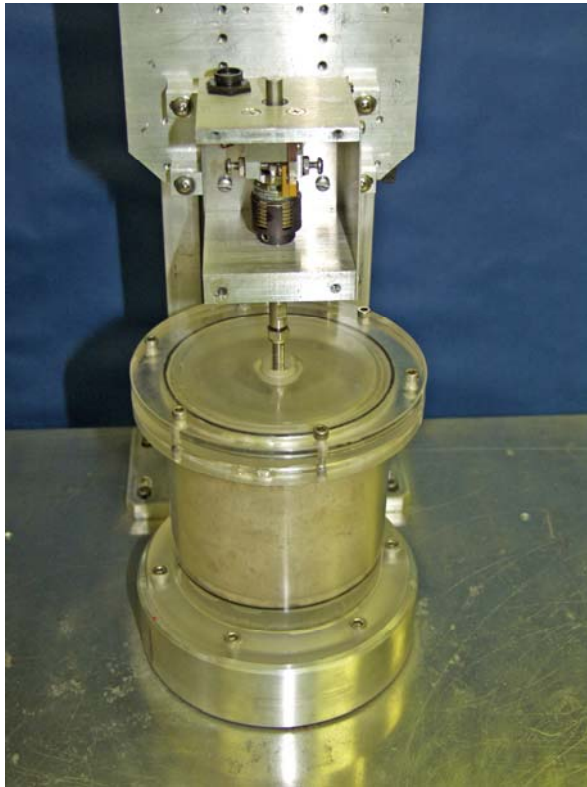
Figure A-6 Front View of the RETA Cylinder with Sample and Torque-Measuring Load Cell.
