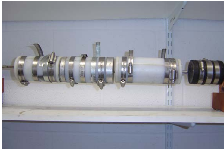
Figure A-7 Gatorock molds secured to the rotating shaft device.
