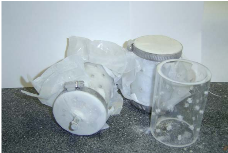
Figure A-9 From left to right: cemented sand molds for the RETA, the SERF, and an empty mold.
