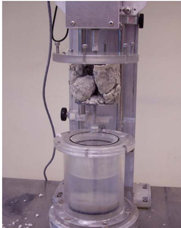
Figure A-11 Cemented sand sample failure in the RETA
