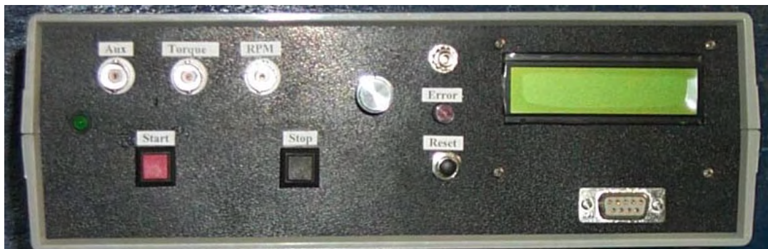
Figure IB - 2. RETA Control Box Front Panel Showing the Location of Various Switches.
