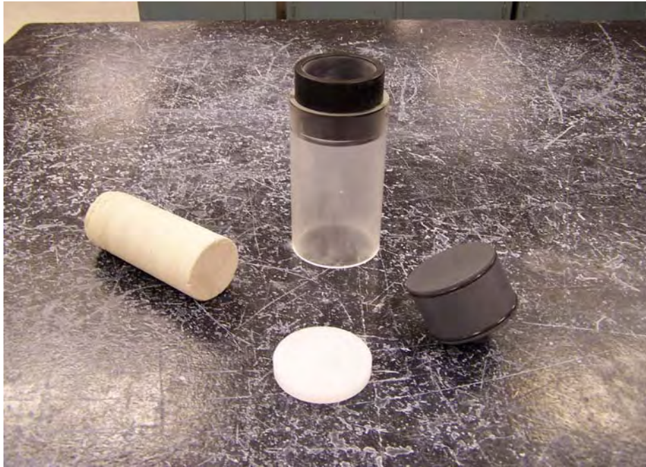
Figure IID - 8. Rock Core Test Cylinder with Separate Components, Cylinder, Rock Core Seat, Plunger, and Rock Sample.
