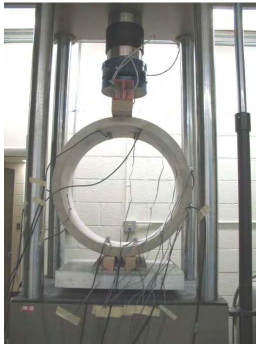
Figure B-3 The three-edge-bearing test on FRCP.
