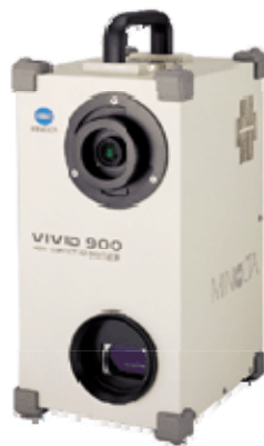
Figure A-4.7 Minolta VIVID 900 non-contact 3-D digitizer.
