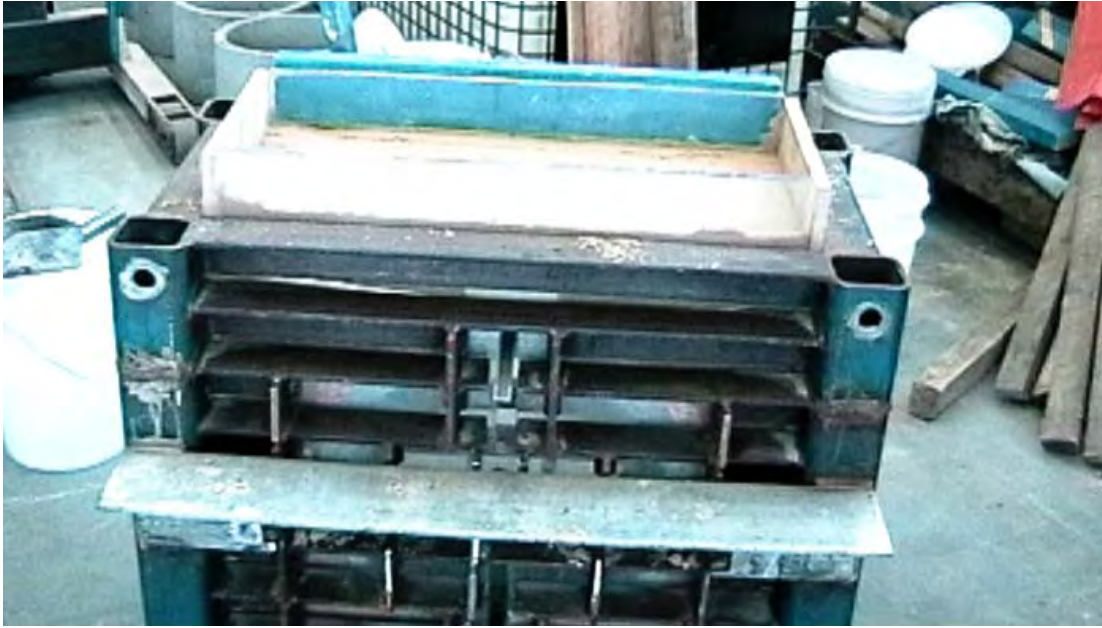
Figure A-2.5 Hardie Pipe's rigid soil box front view (Courtesy of Hardie Pipe Inc.).
