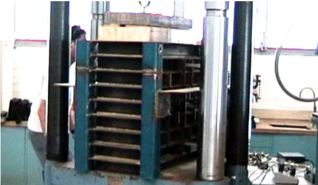
Figure A-2.6 Hardie Pipe's rigid soil box full image view (Courtesy of Hardie Pipe).
