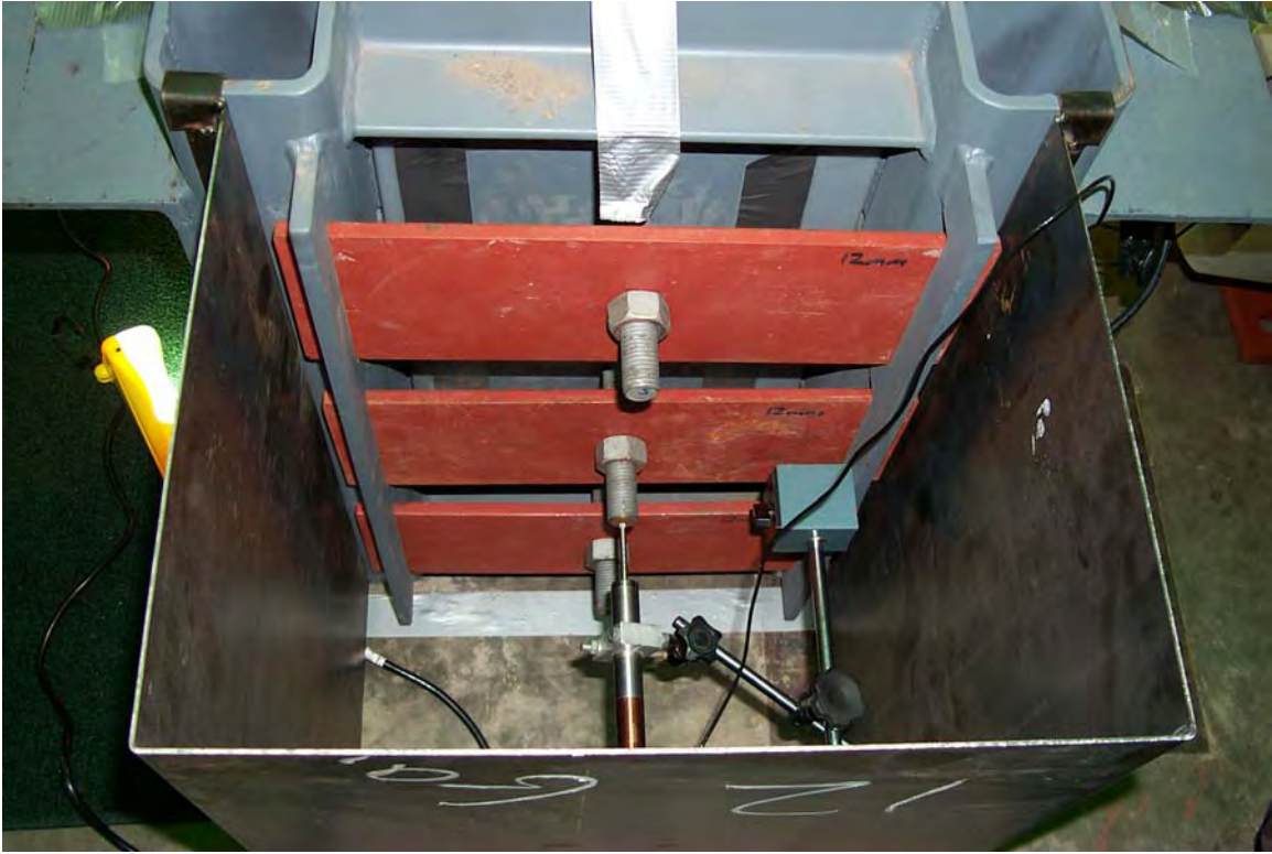
Figure A-2.9 LVDT's shown to measure deflection of sidewalls.
