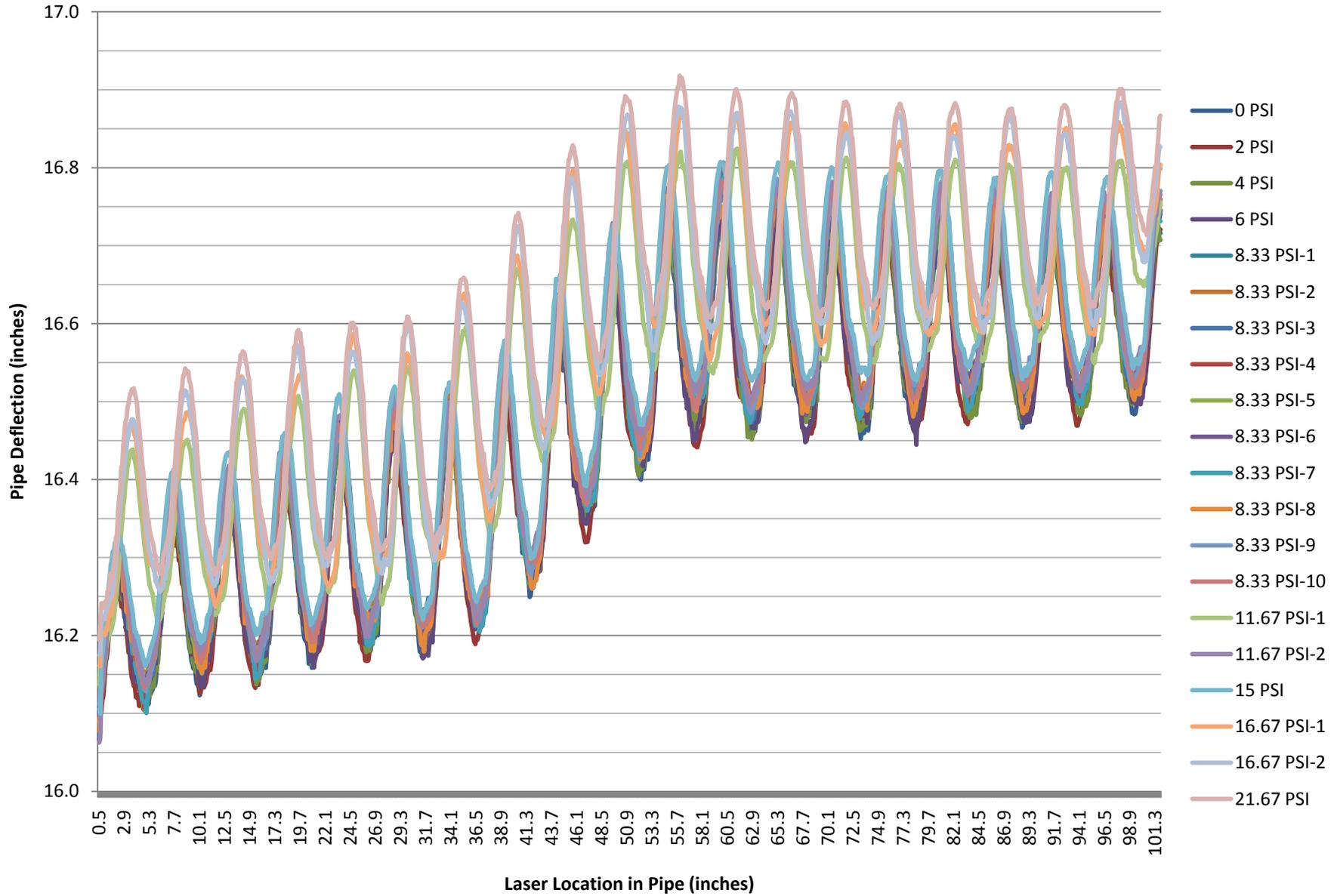
Figure L: HDPE 36" North End Quadrant 2 Profile
