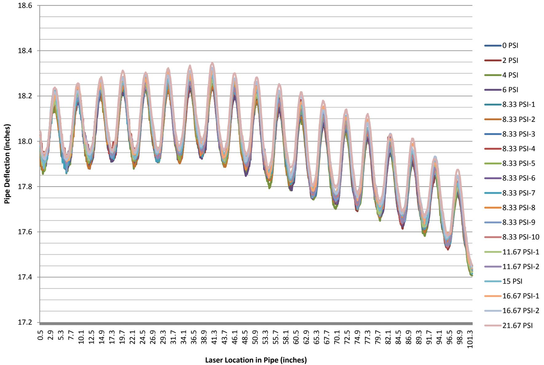
Figure N: HDPE 36" South End Quadrant 1 Profile
