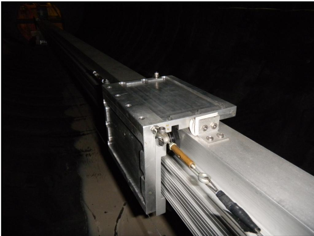
Figure 13: The cart on which the displacement laser mounts.
