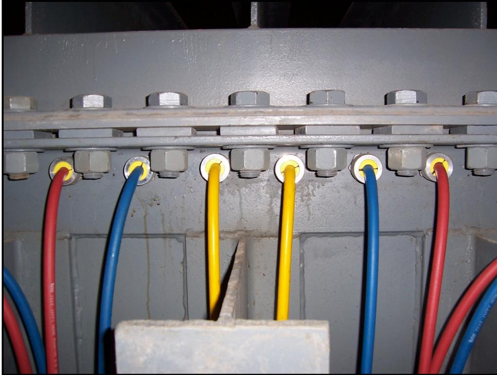
Figure 6: Close-up of air hoses being routed through Soil Box East wall.
