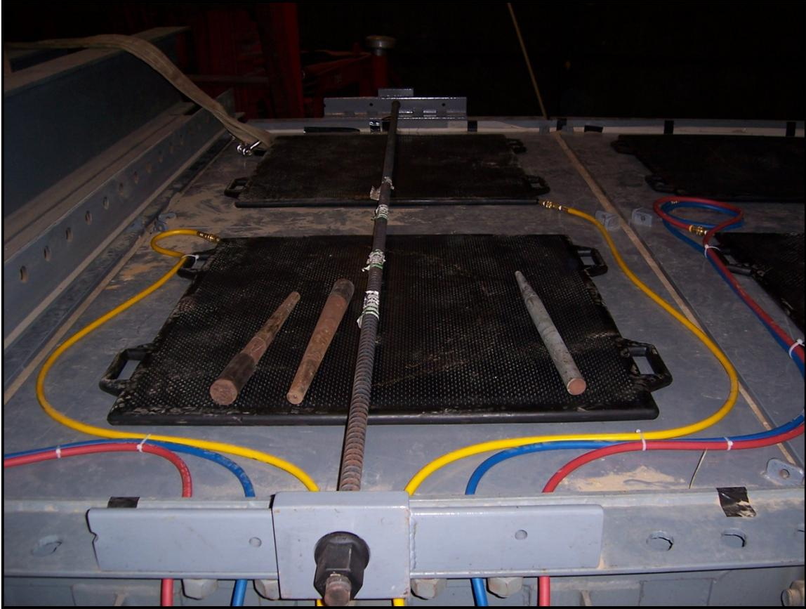
Figure 9: Partial installation of the Soil Box top.
