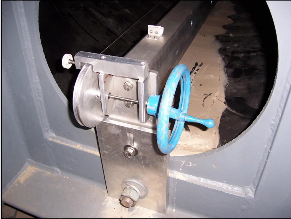
Figure 12: Hand-crank and reel on West end of Soil Box.
