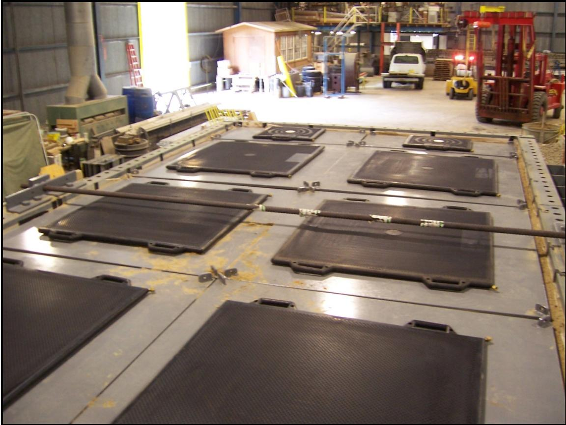
Figure 3: Lift bags after placement directly over center of the load plates.
