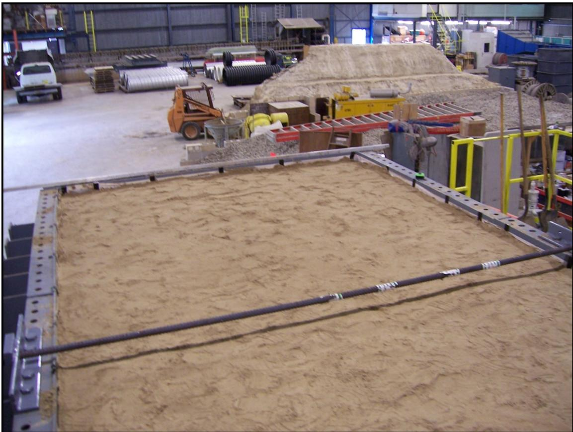
Figure 1: Final soil level in Soil Box.
