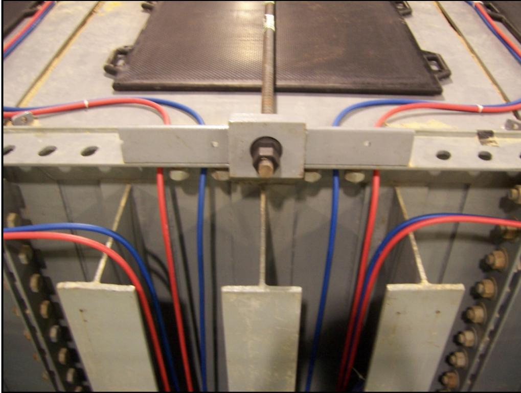
Figure 4: Air hoses routed through and down Soil Box East wall.
