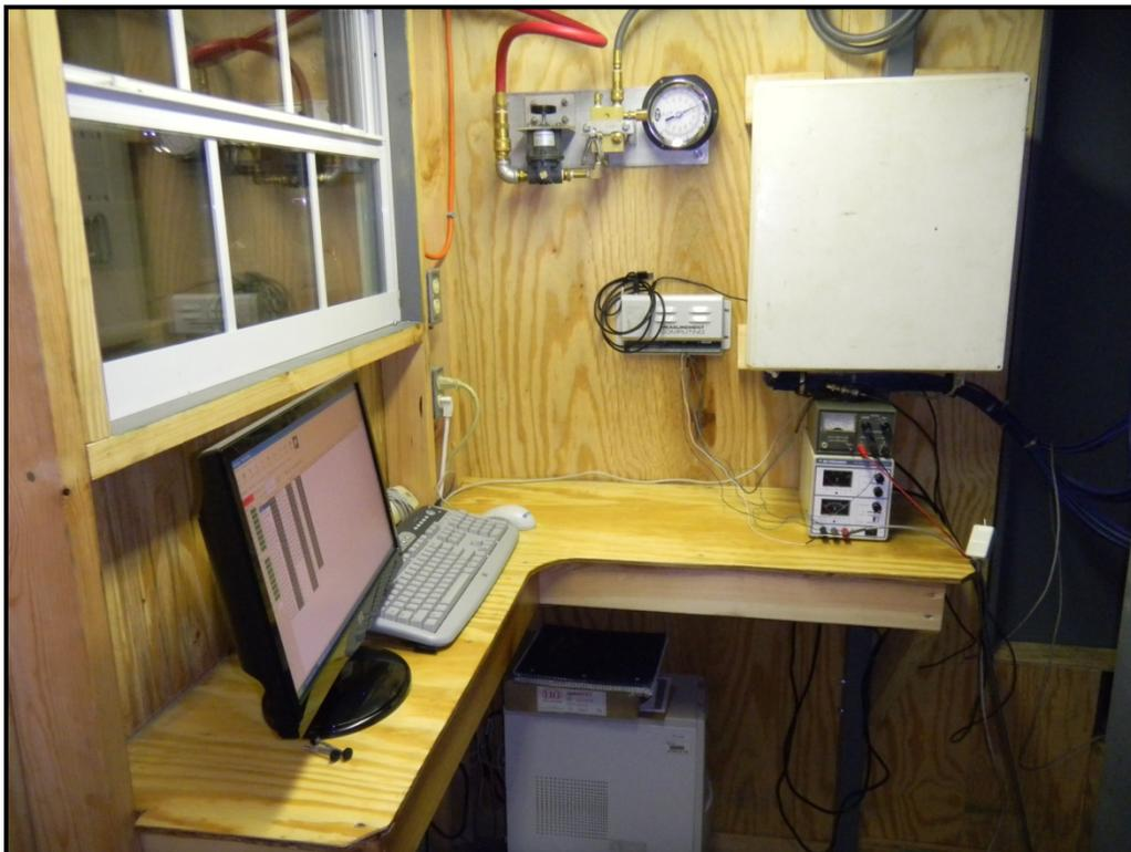
Figure 18: Simplified instrumentation wiring, decreasing the amount of electrical noise.
