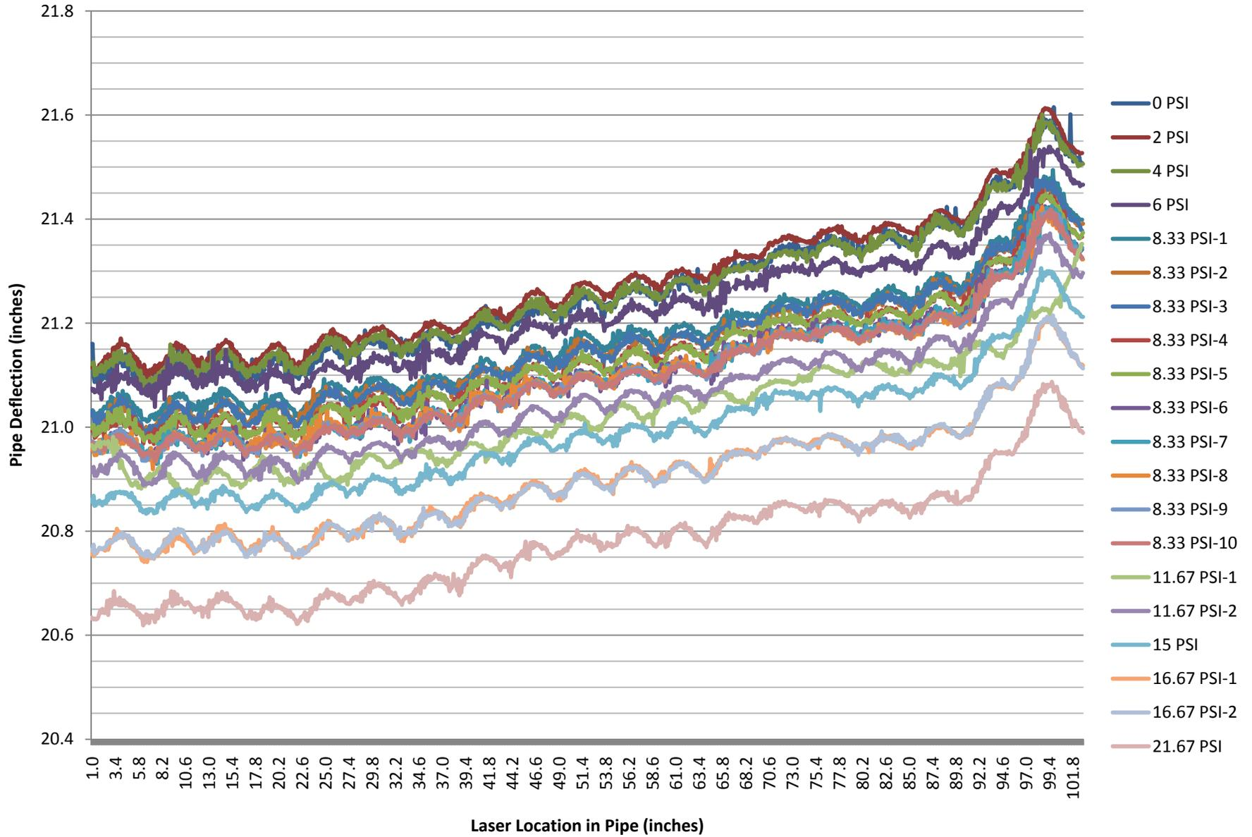
Figure P: HDPE 36" South End Quadrant 3 Profile
