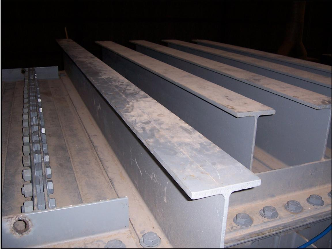
Figure 11: Completed installation of Soil Box top.
