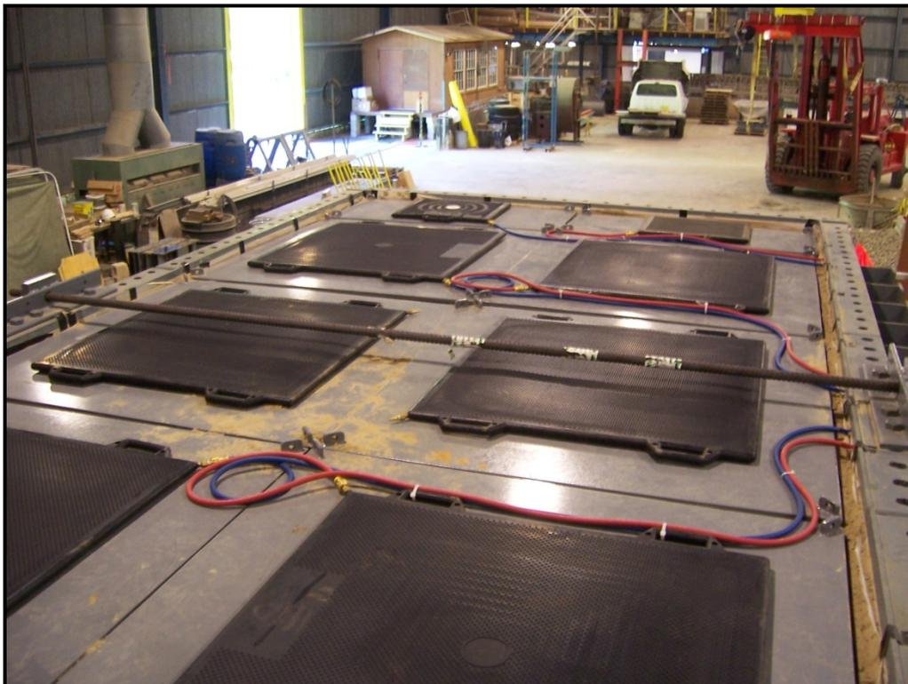
Figure 5: Air hoses connected to lift bags.
