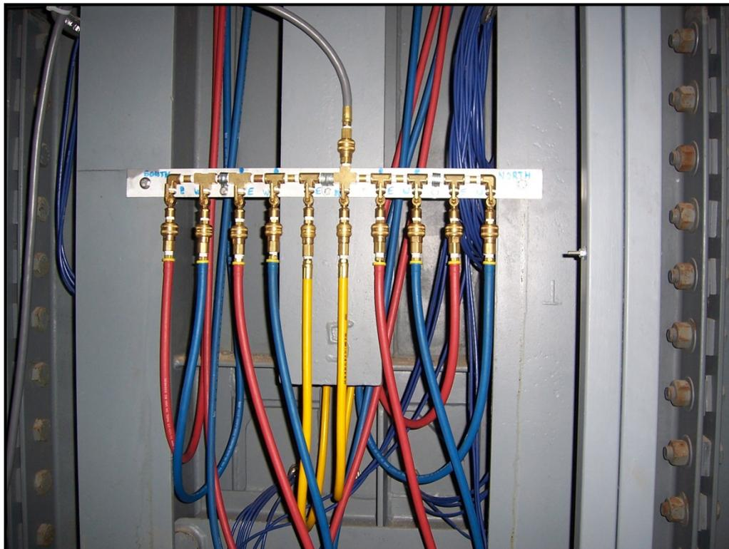
Figure 7: Air hoses connected to pressure source.
