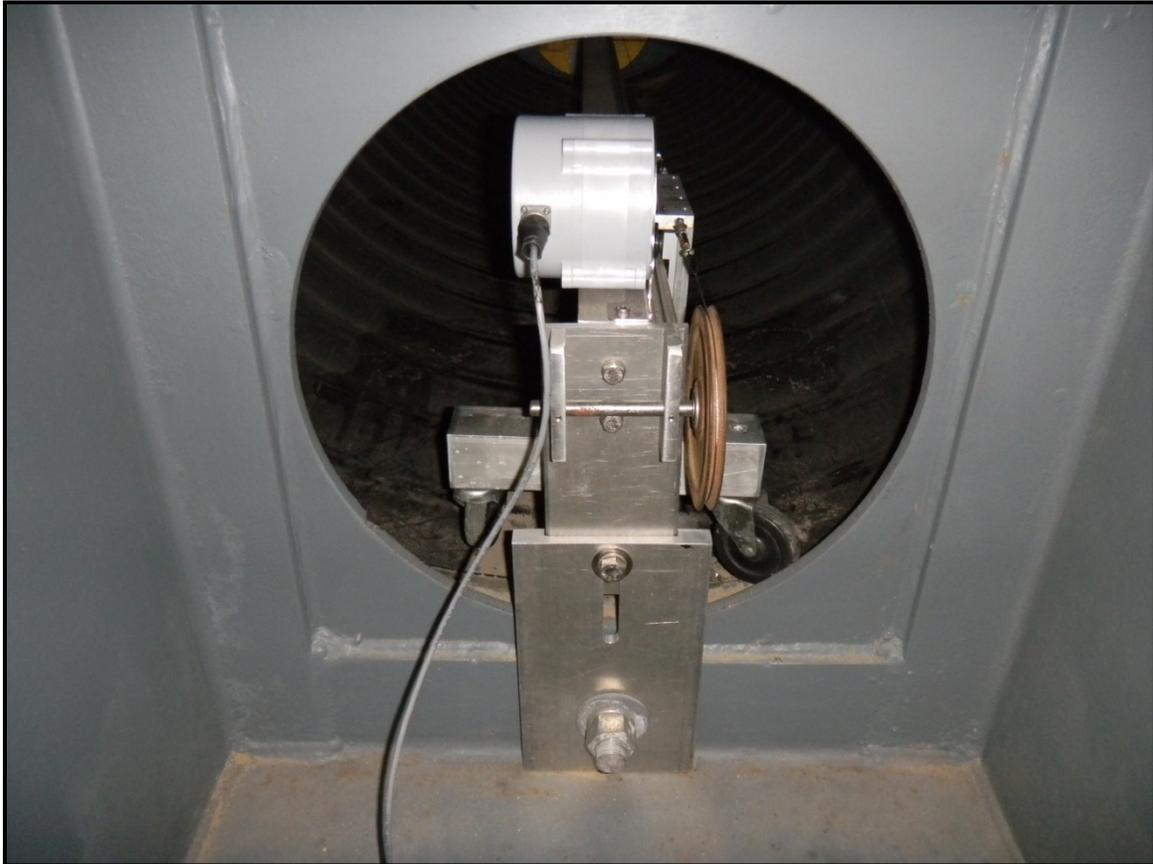
Figure 14: String potentiometer attached on the East end of the track.
