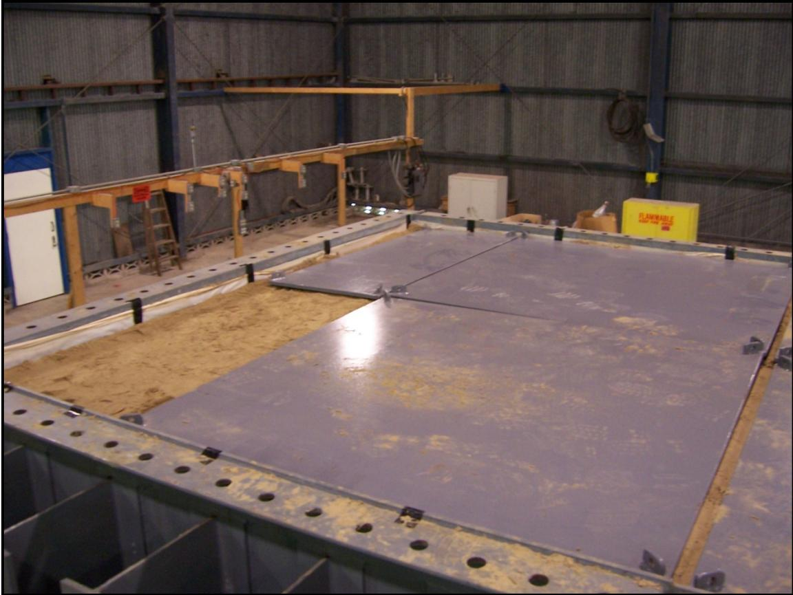
Figure 2: Load plates in the process of installation.
