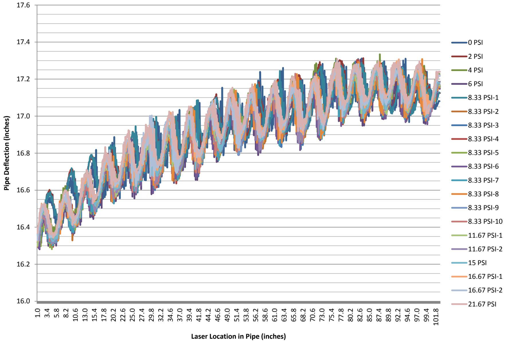
**Figure O: HDPE 36" South End Quadrant 2 Profile**
