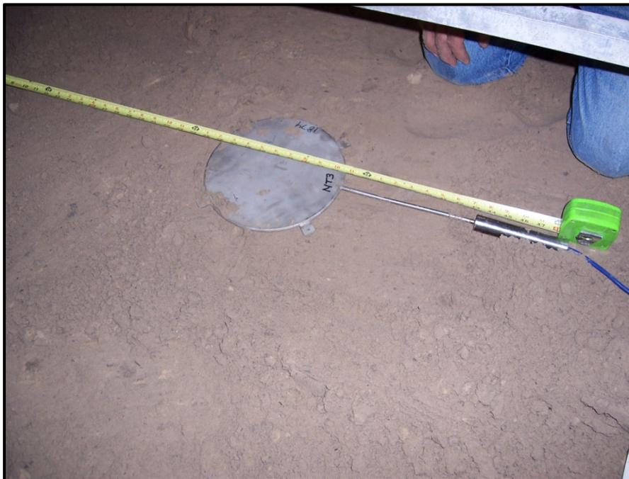
Figure 15: Placement of NT3 pressure cell.
