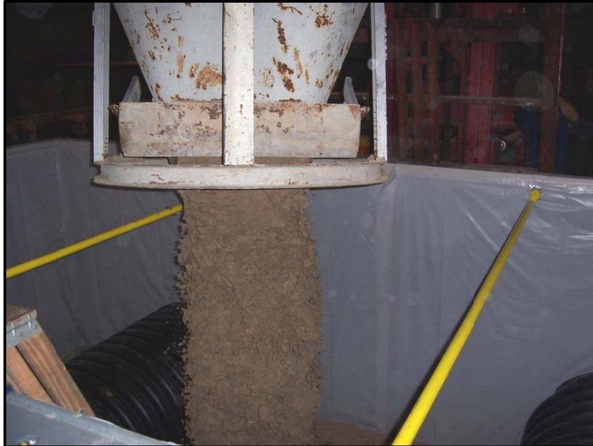
Figure 12: Concrete bucket emptied over Soil Box.
