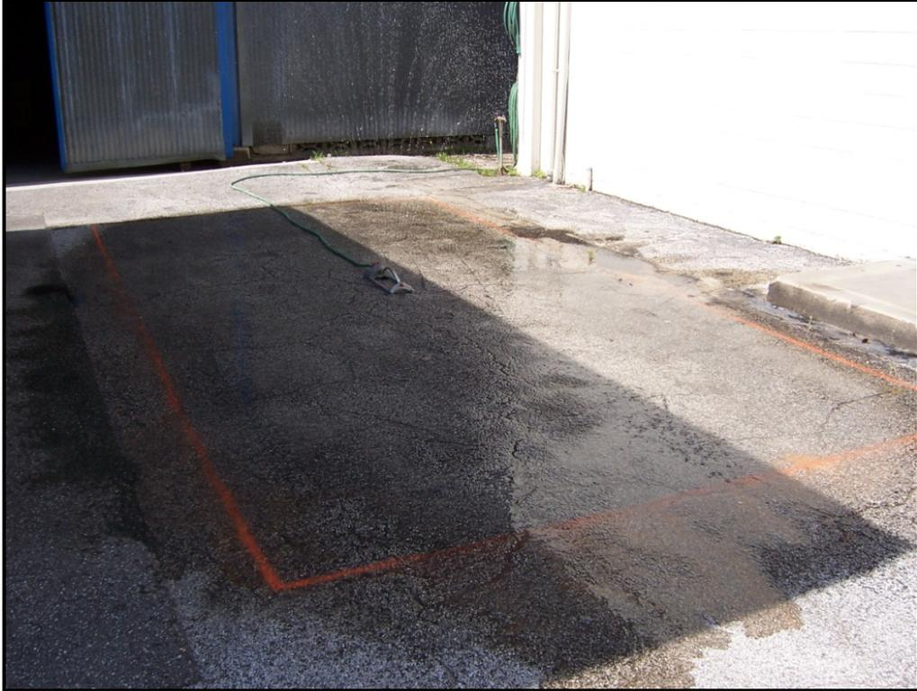
Figure 18: Water pressure being regulated for water to stay within the footprint.
