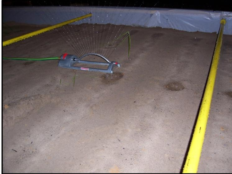
Figure 21: Sprinkler setup inside Soil Box with water beginning to form puddles.
