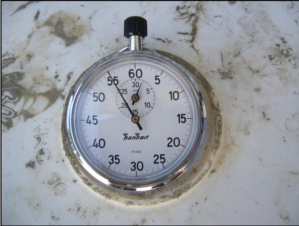
Figure 20: Stopwatch used to record the amount of time needed to fill the bucket.
