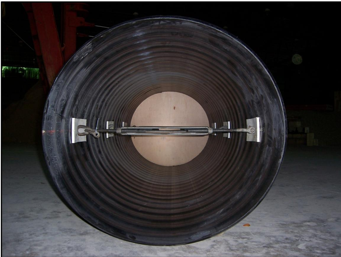
Figure 4: Pre-deflected M294 HDPE pipe with turnbuckles.
