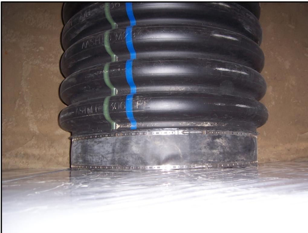
Figure 3: Sealing system between pipe end and Soil Box wall.
