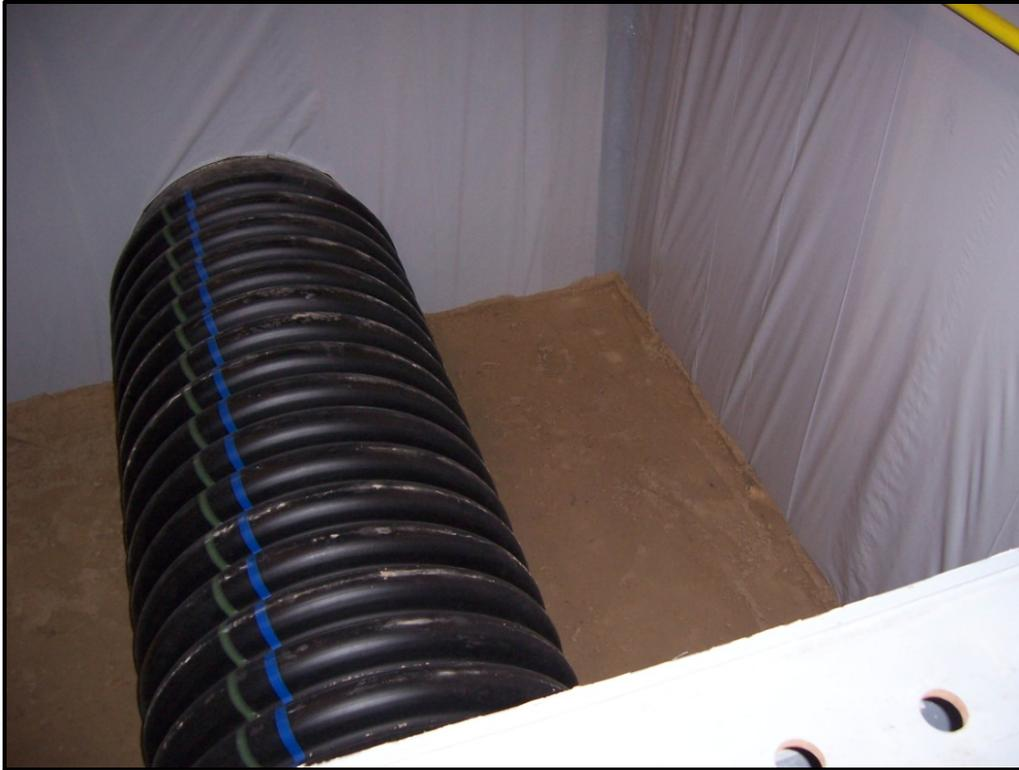
Figure 2: M294 HDPE pipe installed in North end of Soil Box.
