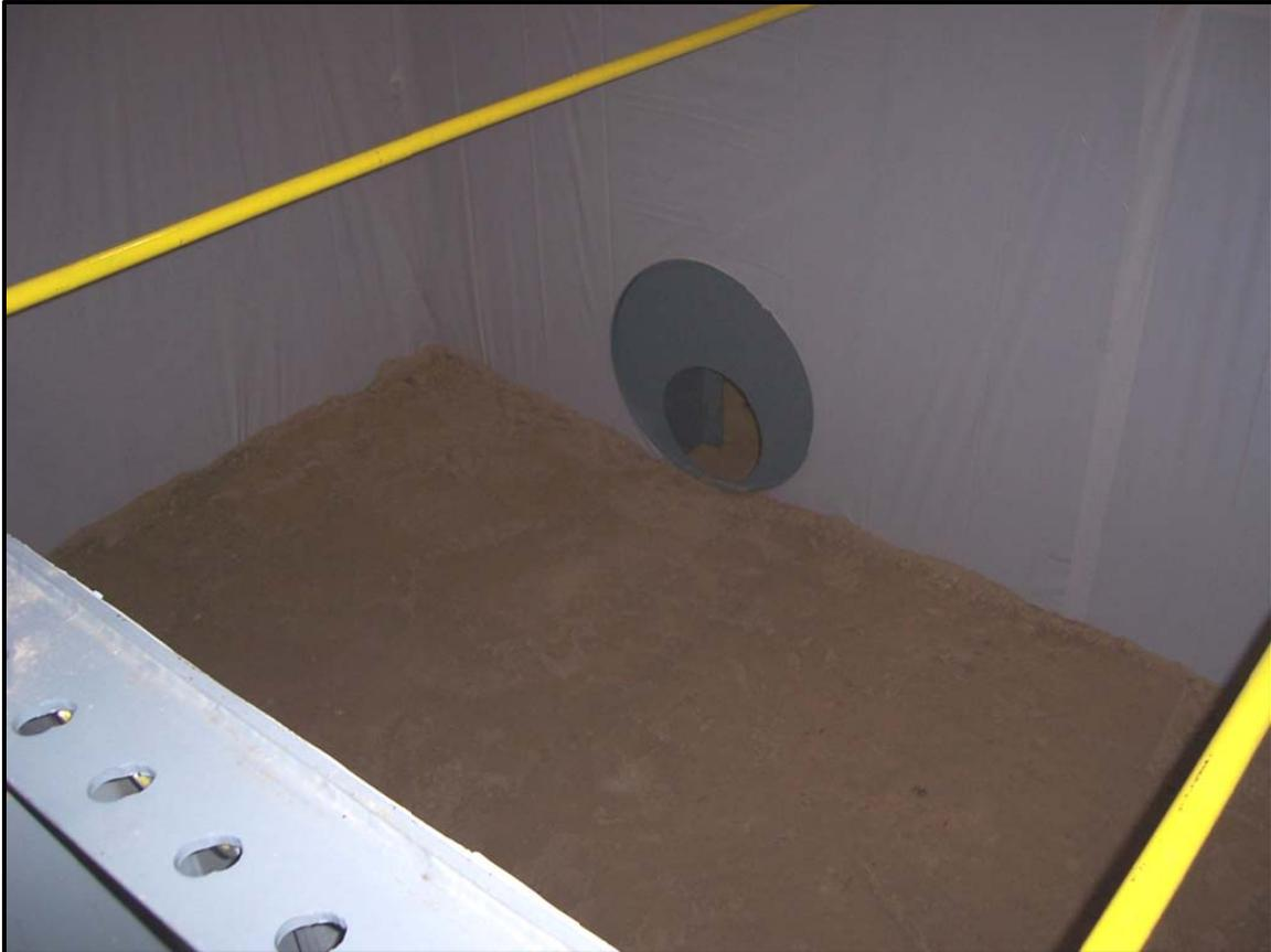
Figure 1: 12 inch thick layer of soil at bottom of Soil Box.
