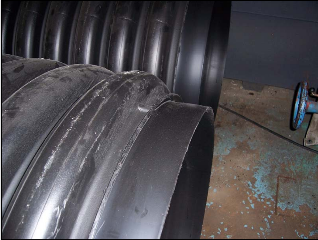
Figure 13: Filed back corrugation on M294 HDPE pipe.
