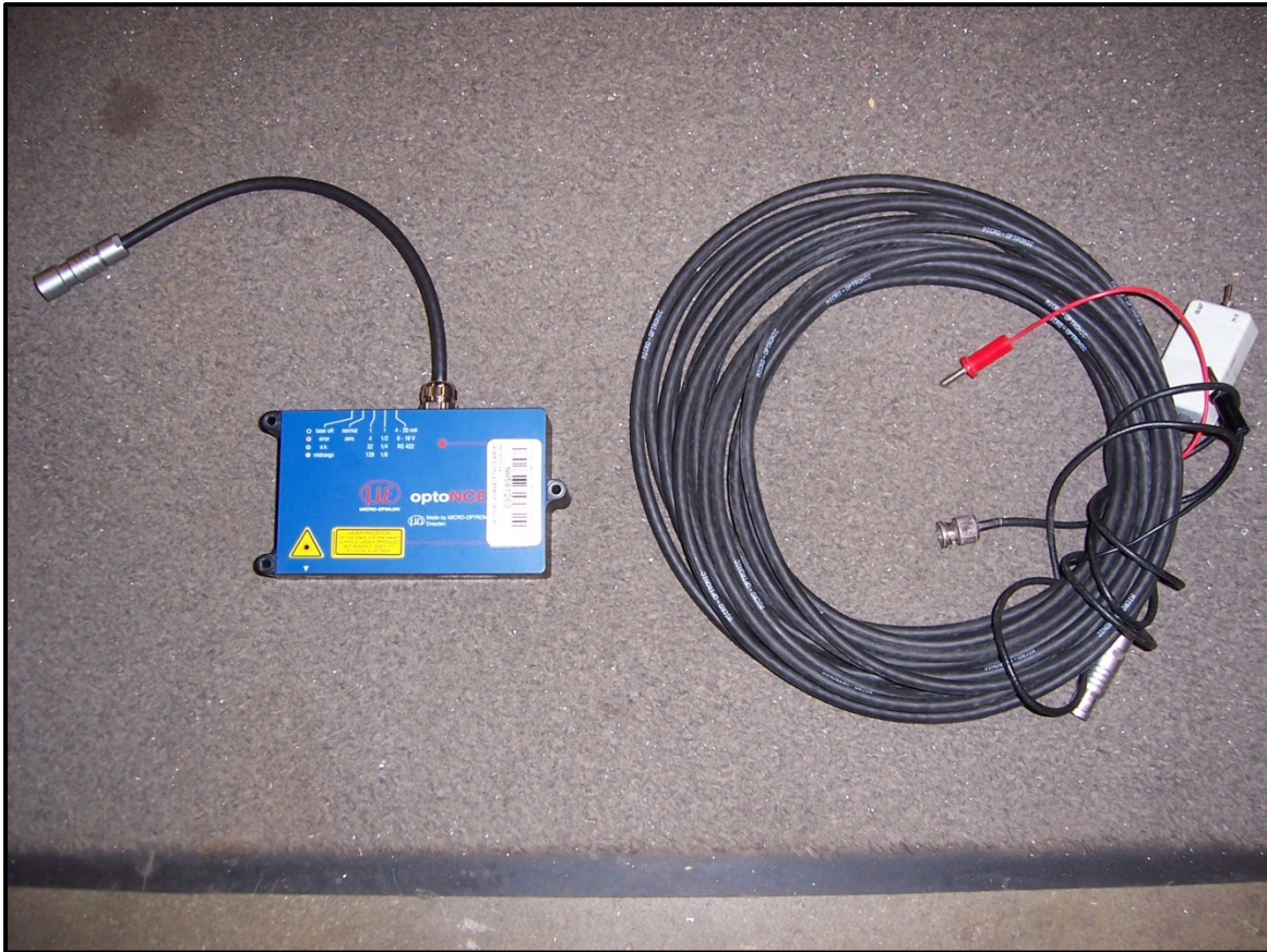
Figure 2: Micro-Epsilon Laser Displacement Sensor and cabling.
