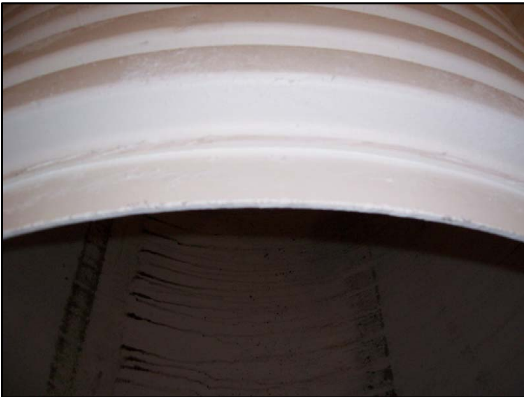
Figure 14: Filed back corrugation on F949 PVC pipe.
