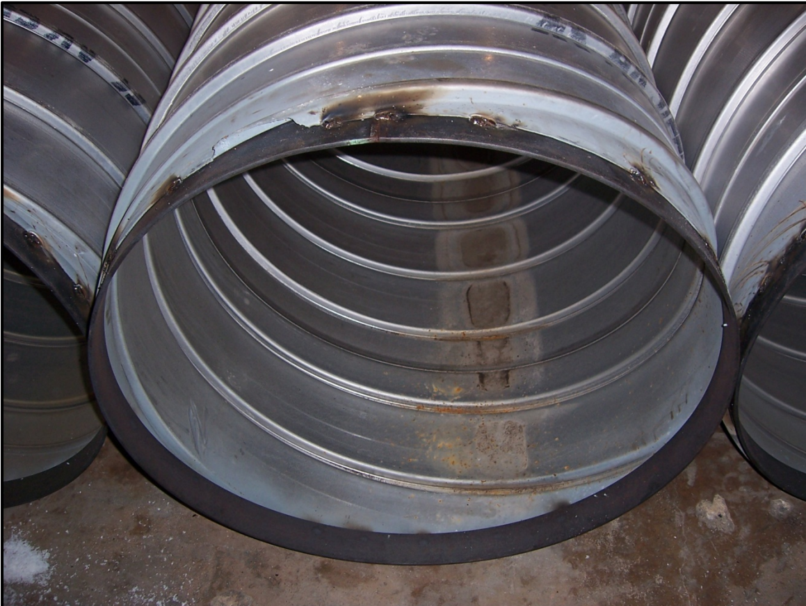
Figure 12: Metal strip welded onto spirally corrugated pipes.
