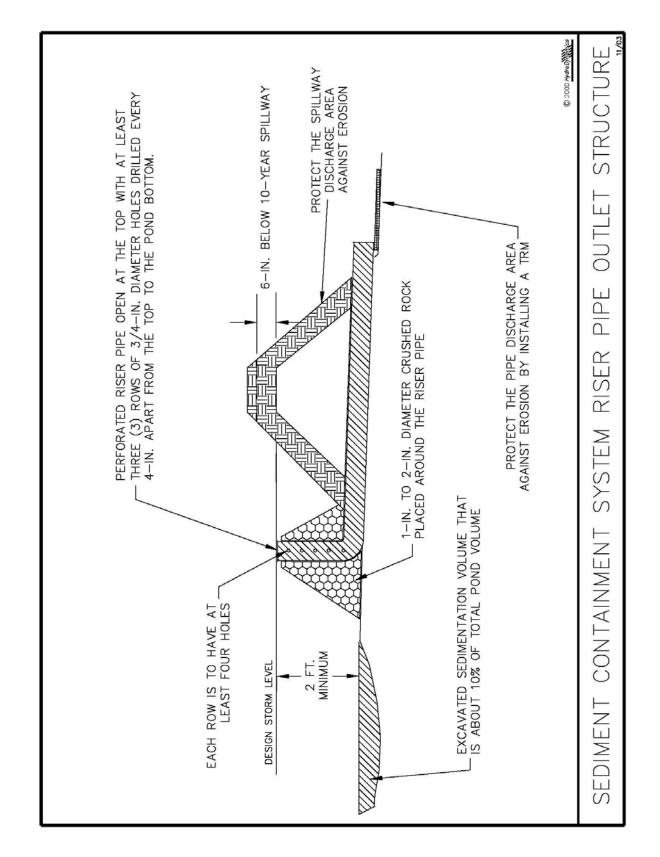
Figure IV-6: Illustration of a SCS Riser Pipe Outlet Structure
