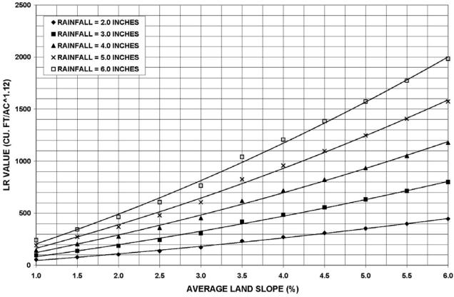
Figure IV-11: Hydrologic Type D Soils Loading Ratio Graph
