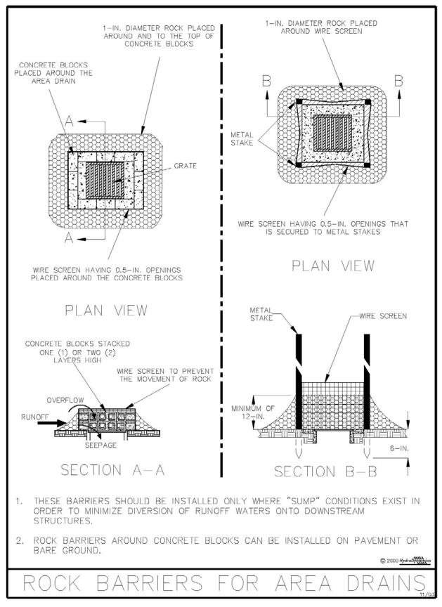
Figure V-13: Illustration of Rock Barriers around Area Drains
