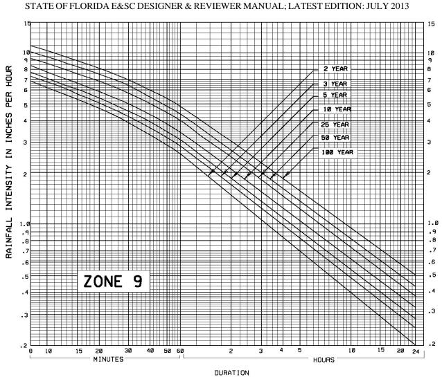
Figure III-21. Rainfall Intensity Duration Frequency Curve for Zone 9 (FDOT, 2001)
