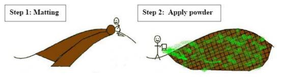
Figure AIII-6: Polymer-enhanced Armoring with Matting.
