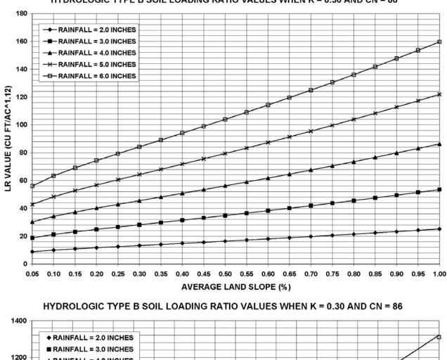
HYDROLOGIC TYPE B SOIL LOADING RATIO VALUES WHEN K = 0.30 AND CN = 86
