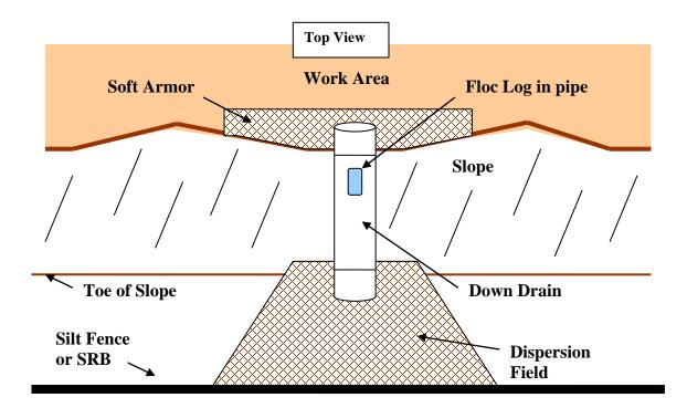
*Limitations*: High flow velocities will occur at the discharge end of the slope drain. Unless there is a great distance between the slope drain discharge end and the silt fence, and a pond is created, the silt fence barrier may be destroyed if the inflow values are greater than outflow.
