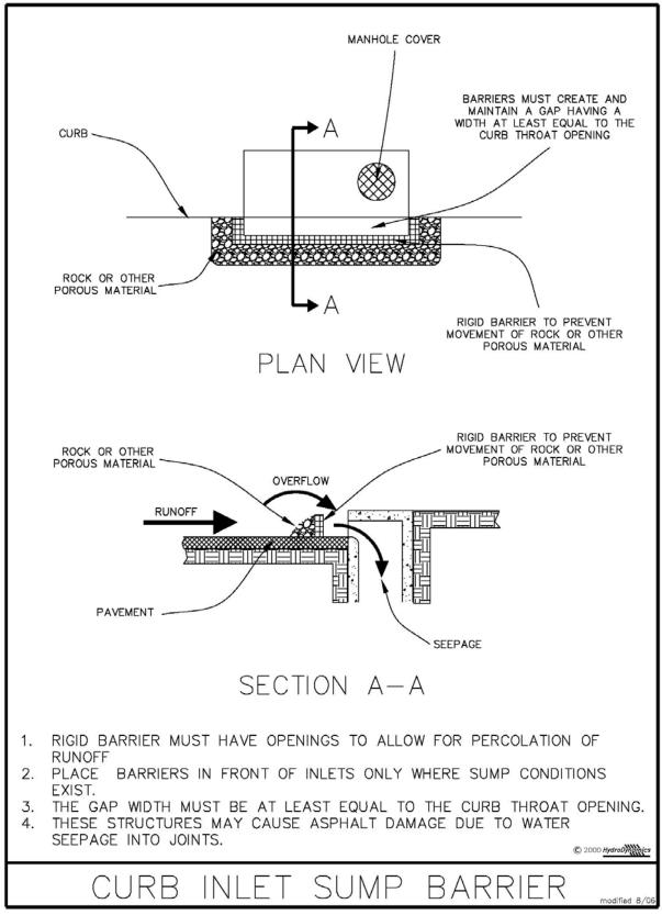
Figure V-15: Illustration of a Curb Inlet "Sump" Barrier
