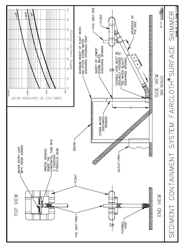
Figure IV-4: Illustration of a SCS Faircloth® Surface Skimmer
