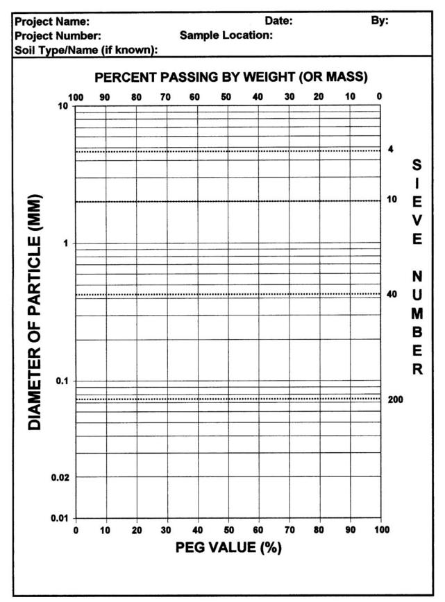
Figure IV-2: PEG Chart for Sediment Containment Systems (Fifield, 2004)
