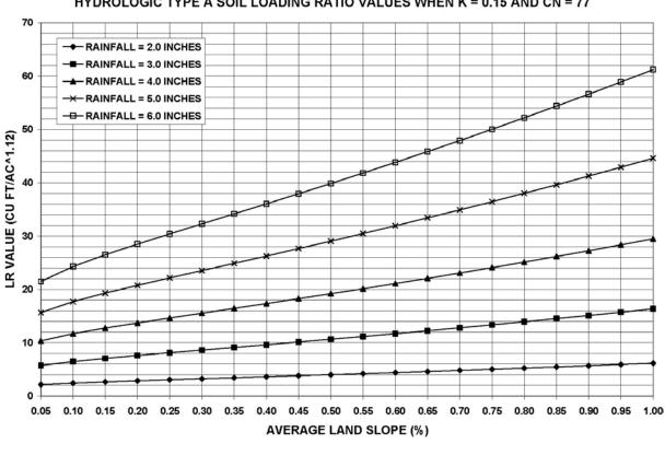
HYDROLOGIC TYPE A SOIL LOADING RATIO VALUES WHEN K = 0.15 AND CN = 77
