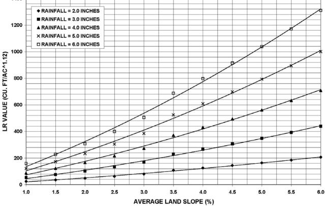
Figure IV-9: Hydrologic Type B Soils Loading Ratio Graph
