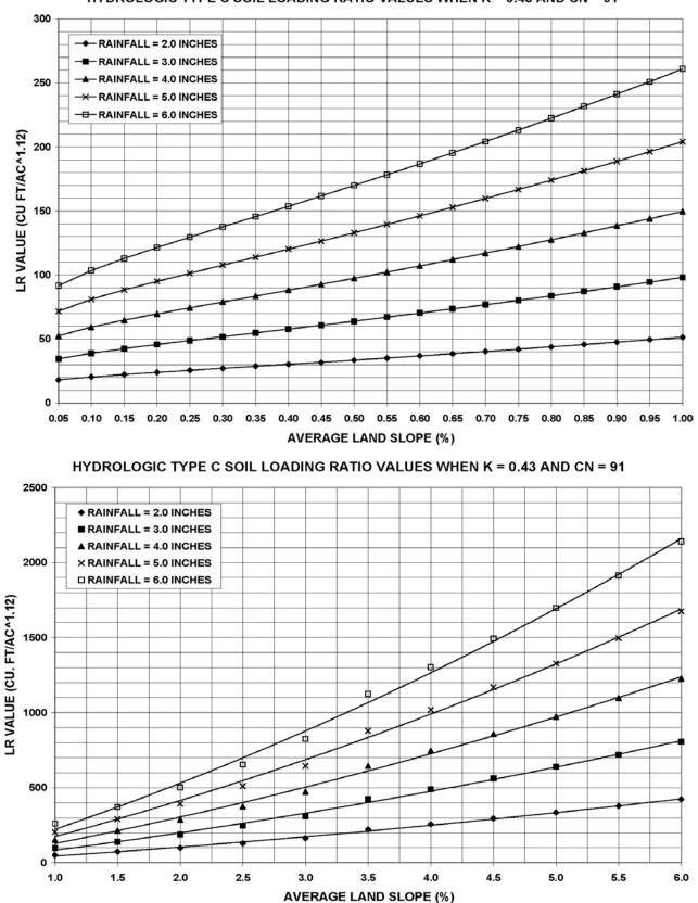
HYDROLOGIC TYPE C SOIL LOADING RATIO VALUES WHEN K = 0.43 AND CN = 91
