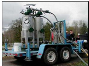
Sand Media Particulate Filter (Source: http://www.spillcontainment.com)
