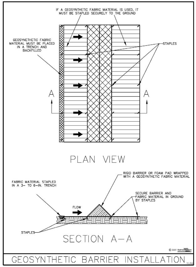
Figure V-8: Illustration of a Geosynthetic Barrier
