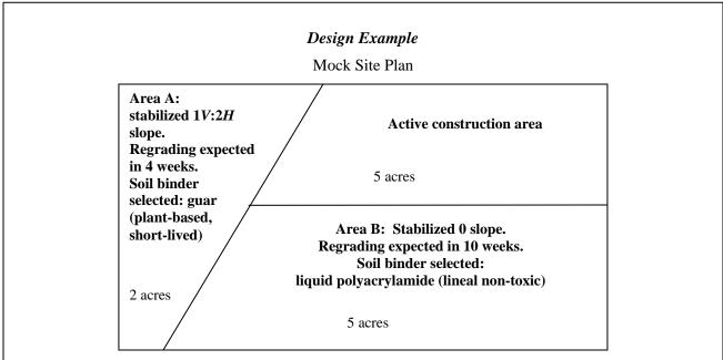
A designer on a 12-acre coastal construction project selects two soil binders for temporary soil stabilization as construction activities are phased across the site. The amount of binder needed is calculated as follows:
