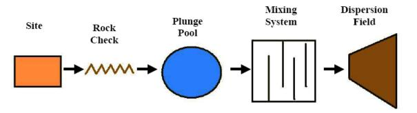
Figure AIII-22: Polymer-enhanced Particle Collection.
