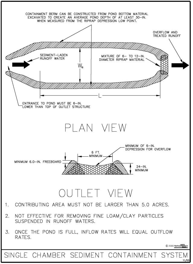
Figure IV-13: Illustration of a Single Chamber SCS Permission is given by HydroDynamics Incorporated to copy and reproduce this detail
