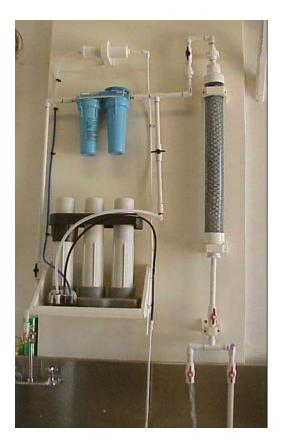
Figure AIII-1: Polymer Log dosage sampling device.
