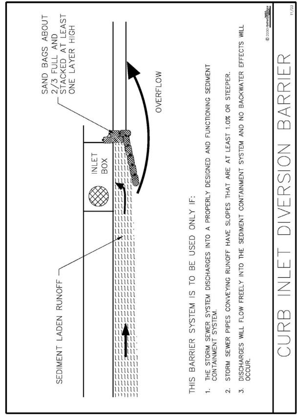
Figure V-16: Illustration of a Curb Inlet Diversion Berm
