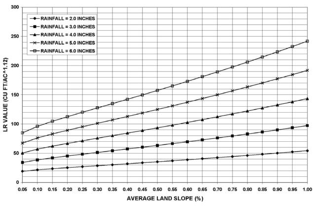
HYDROLOGIC TYPE D SOIL LOADING RATIO VALUES WHEN K = 0.37 AND CN = 94
