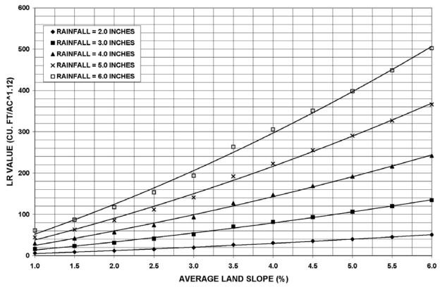
Figure IV-8: Hydrologic Type A Soils Loading Ratio Graph
