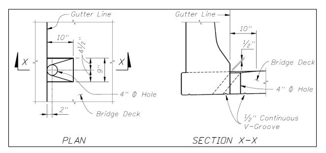
Figure 5.6-2: Standard FDOT Scupper Detail
