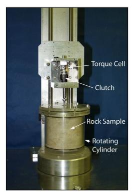
Figure 5.5-9: Rotating Erosion Test Apparatus (RETA, above)
