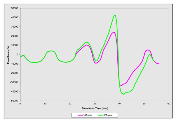
Figure 5.7-10: Flow Rate Time Series during the Design and Check Event at the SR-A1A Bridge over the Loxahatchee River
