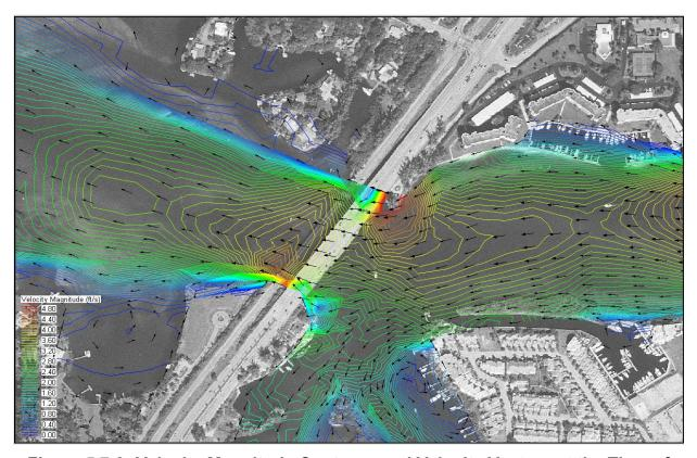
Figure 5.7-9: Velocity Magnitude Contours and Velocity Vectors at the Time of Maximum Velocity during the 100-Year Storm Surge Event at the SR-A1A Bridge over the Loxahatchee River
