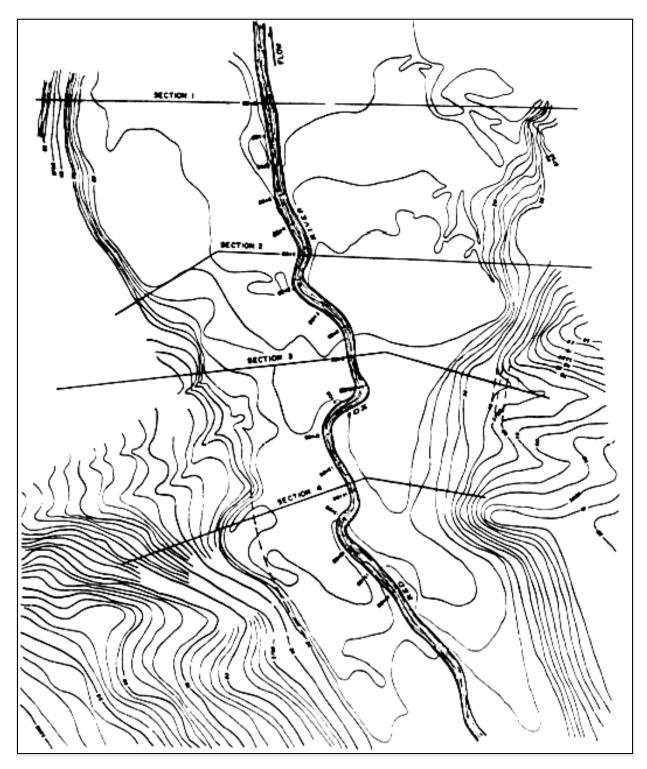
Figure 5.2-5: "Dog Legging" Cross Section
