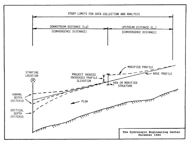
Figure 5.2-3: Open Channel Depth Profiles
