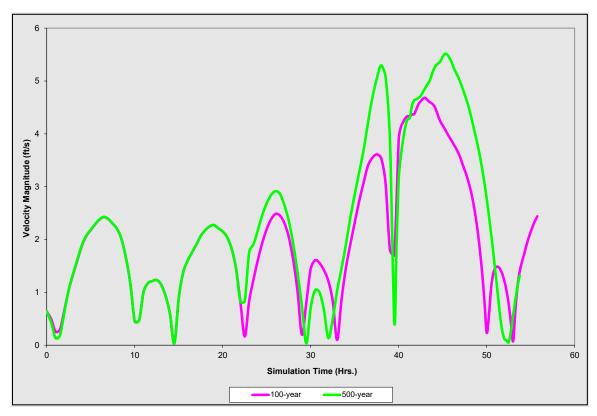
Figure 5.7-12: Velocity Magnitude Time Series during the Design and Check Event at the SR-A1A Bridge over the Loxahatchee River
