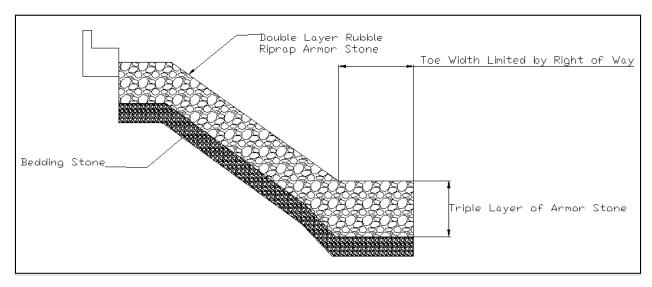
Figure 5.5-12: Example of Increased Toe Thickness to Offset Decrease in Toe Width
