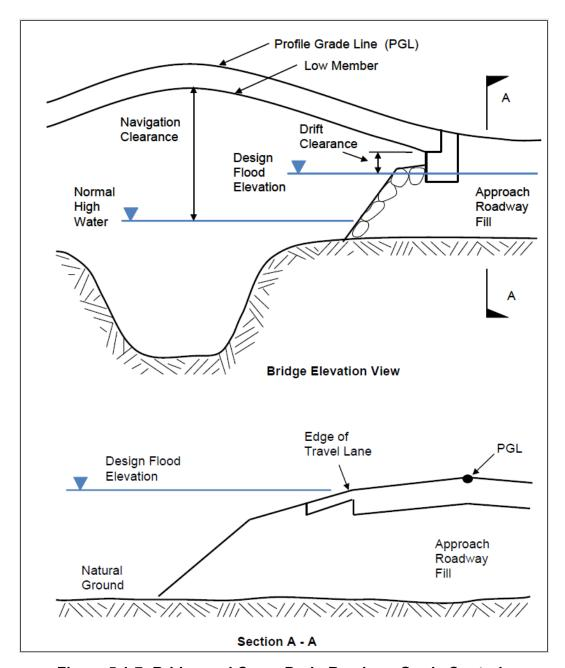
Figure 5.1-7: Bridge and Cross Drain Roadway Grade Controls
