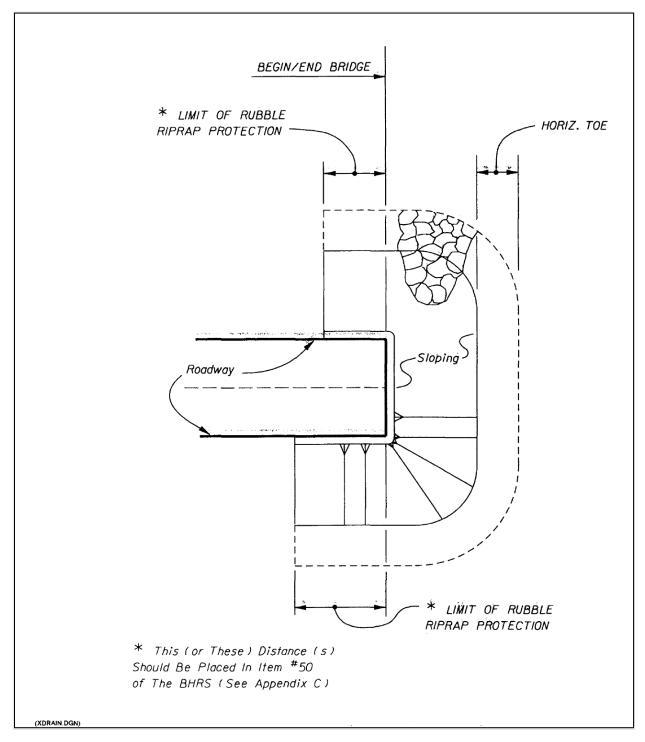
Figure 5.1-8: Limits of Rubble Riprap Protection
