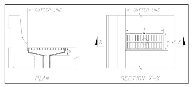
Figure 5.6-5: Grated Free-Draining Scupper
