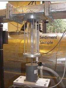
Figure 5.5-10: Sediment Erosion Recirculating Flume (SERF)
