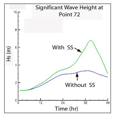
Figure 5.3-12: Wave Height Simulation during Hurricane Katrina with No Coupling (Without SS Curve) and with One-Way Coupling (With SS Curve) (Source: Sheppard et al., 2006)
