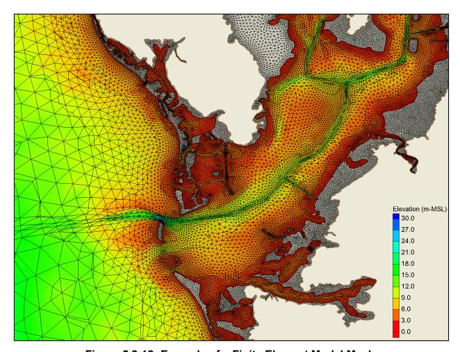
Figure 5.2-12: Example of a Finite Element Model Mesh
