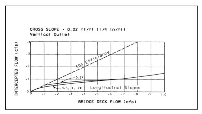
Figure 5.6-4 Intercepted Flow for 4-inch Bridge Scuppers Cross Slope = 0.02 ft/ft
