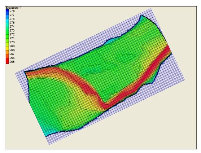
Figure 5.2-11: Example of a Finite Difference Model Mesh
