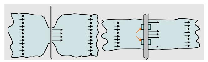
Figure 5.5-1: Examples of Contractions at Bridge Crossings
