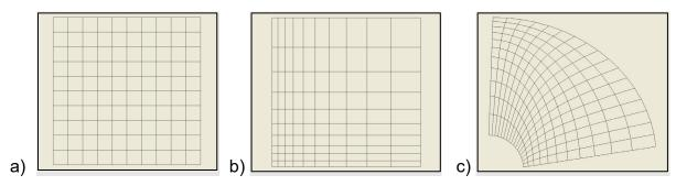
Figure 5.2-10: Example of (a) Cartesian, (b) Rectilinear, and (c) Curvilinear Grids
