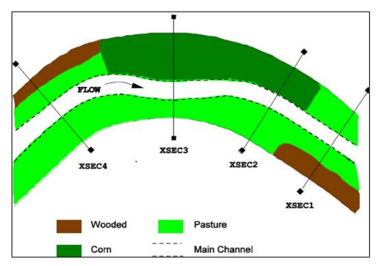
Figure 5.2-4: Example Cross Section Spacing
