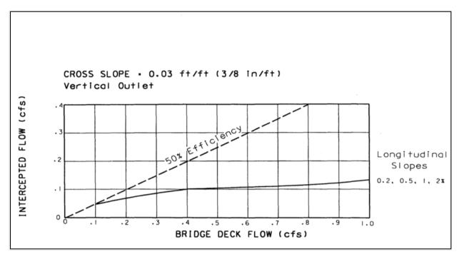
Figure 5.6-3: Intercepted Flow for 4-inch Bridge Scuppers
