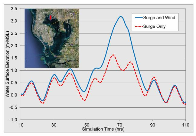
Figure 5.3-14: Surge Elevations at the Courtney Campbell Bridge Location during the 1852 Unnamed Hurricane both with and without Local Wind Effects
