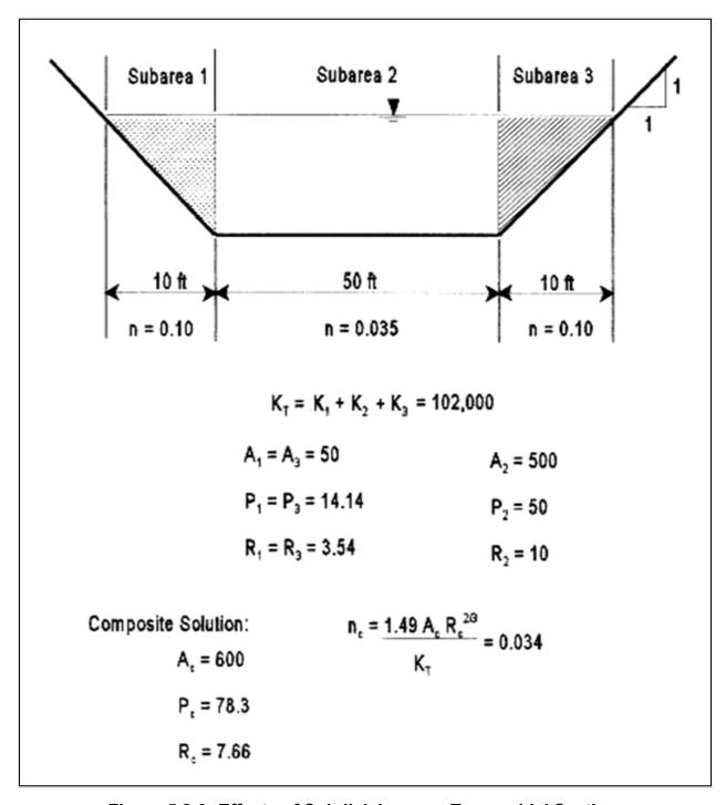
Figure 5.2-9: Effects of Subdivision on a Trapezoidal Section
