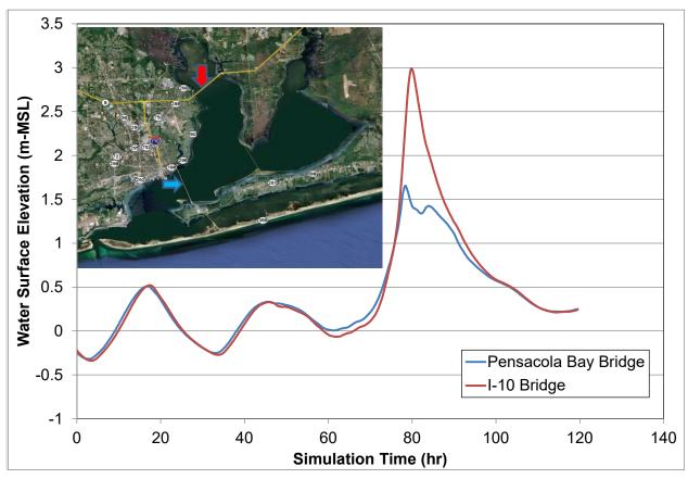
Figure 5.3-15: Hindcasted Surge Elevations at the I-10 over Escambia Bay Bridge and Pensacola Bay Bridge during Hurricane Ivan 2004.
