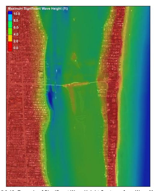
Figure 5.3-18: Example of Significant Wave Height Contours from Wave Modeling
