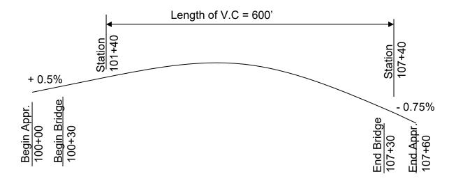
The ground beneath the bridge is less than 25 feet below the bottom of the bridge deck for a distance of 50 feet from each bridge end. Determine the required deck drainage features.
