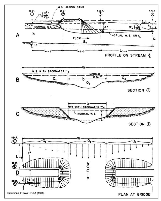
Figure 5.2-15: Normal Crossings: Spill-through Abutments
