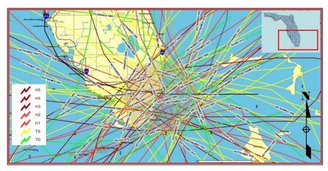
Figure 5.3-6: Hurricane and Tropical Storm Tracks Passing within 50 Nautical Miles (nmi) of Miami (Source: NHC)
