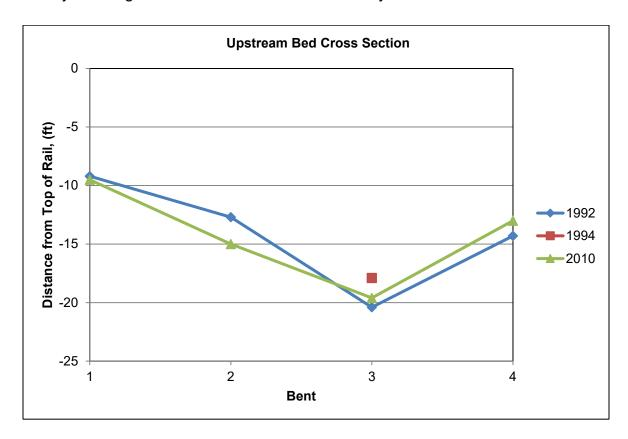
Figure 5.5-7: Example of Normal, Everyday Scour Holes from Bridge Inspection Data
