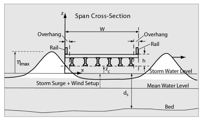
Figure 5.3-20: Definition Sketch for Wave Forces
