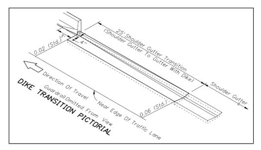
Figure 5.6-1: Shoulder Gutter Transition at Bridge End
