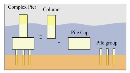
Figure 5.5-4: Complex Pier Components
