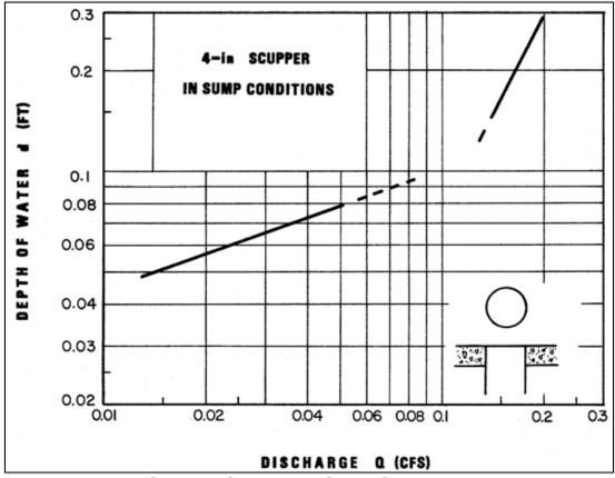
**Scupper Capacity in Sump Conditions**
