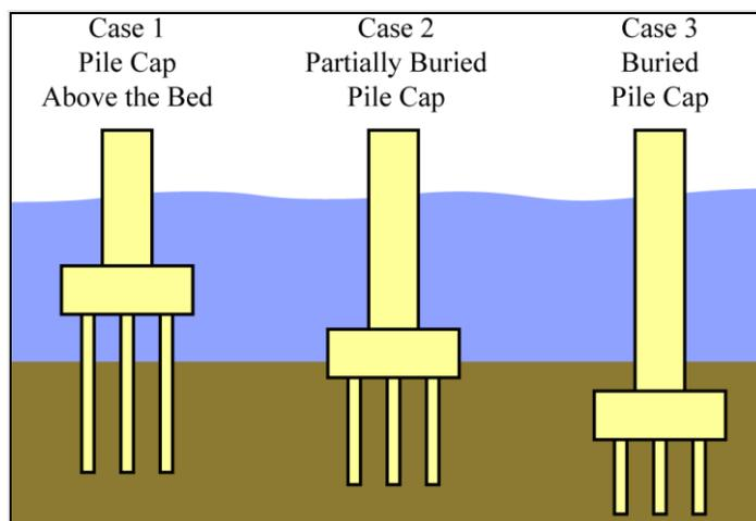
**Figure 5.5-5: Three Cases of Local Scour Depth for Complex Pier Computations**
