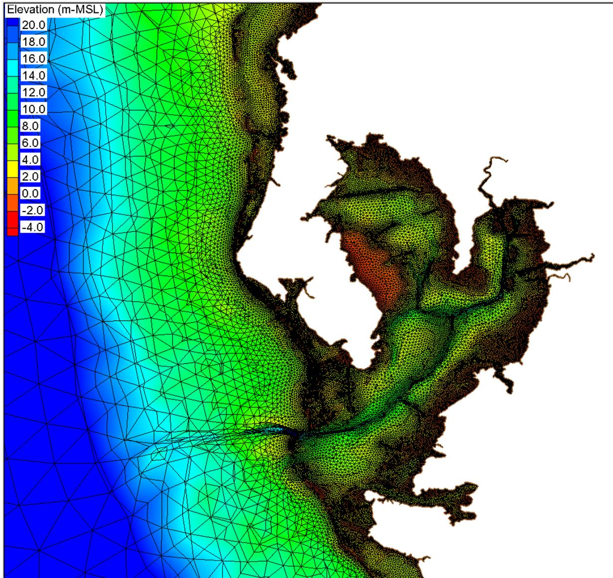
Figure 5.7-5: Model Mesh at Tampa Bay
