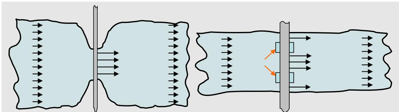
**Figure 5.5-1: Examples of Contractions at Bridge Crossings**
