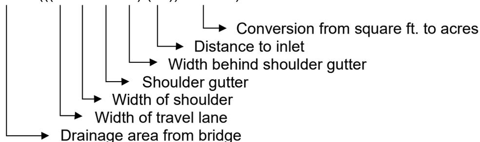
Assume that the location of the bridge and the NOAA Atlas 14 Point Precipitation Frequency Estimates webpage are used to provide the 10-year, 10 minute rainfall intensity of 7.0 inches per hour. The flow to the inlet is:
