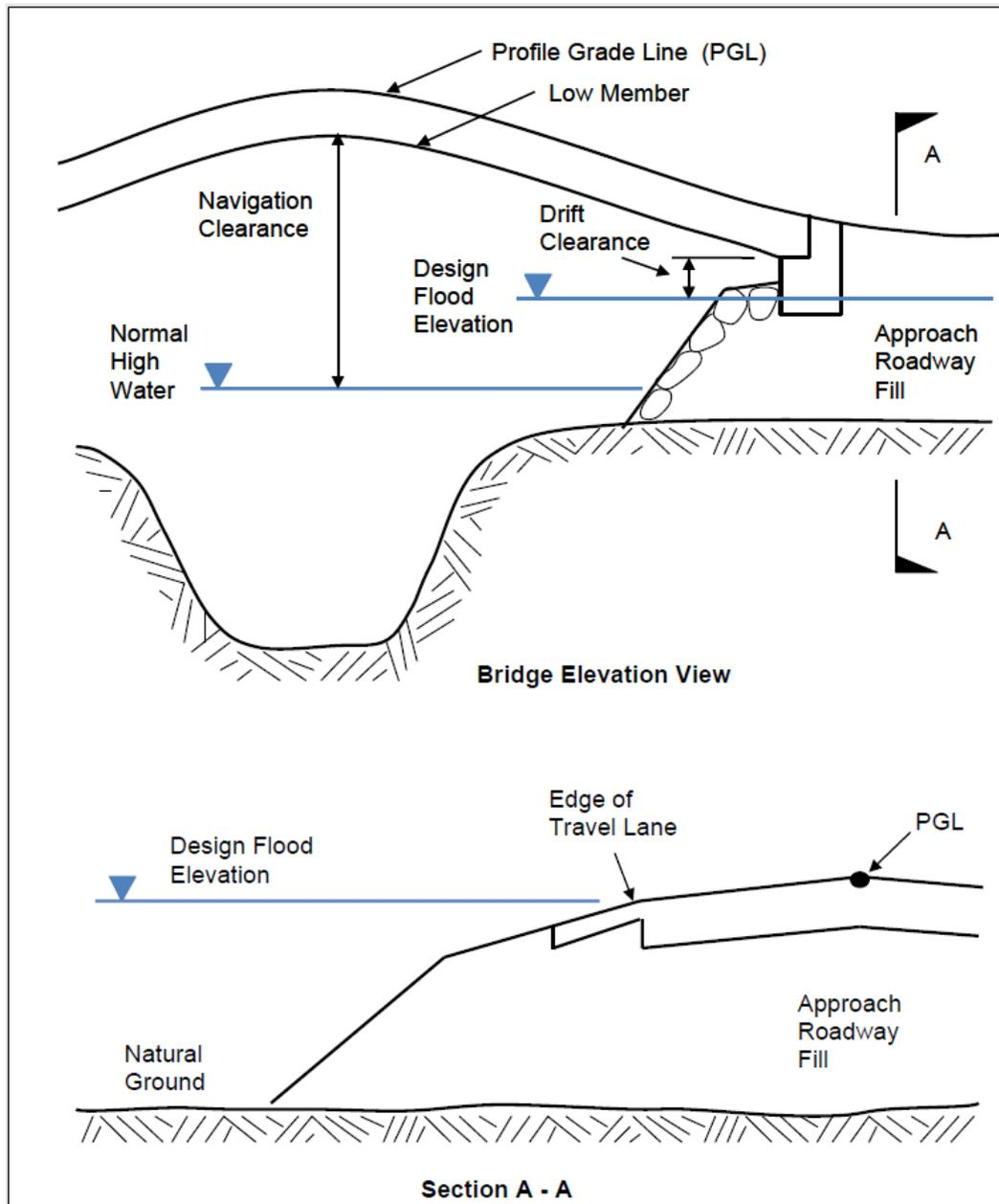
**Figure 5.1-7: Bridge and Cross Drain Roadway Grade Controls**
