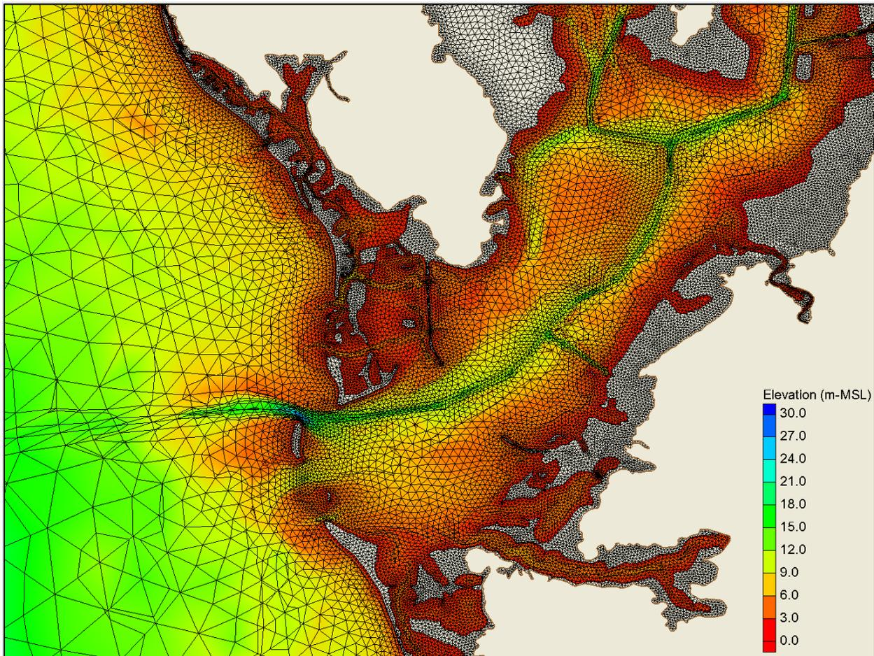
**Figure 5.2-12: Example of a Finite Element Model Mesh**
