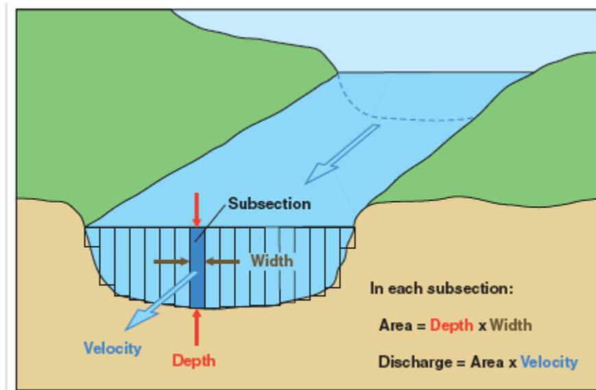
**Figure 5.2-19: Discharge Determination with a Velocity Meter**
