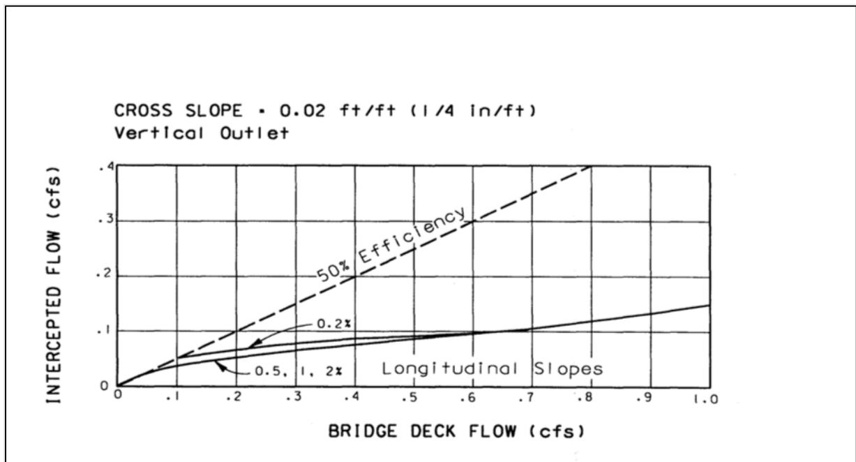
**Figure 5.6-4 Intercepted Flow for 4-inch Bridge Scuppers
