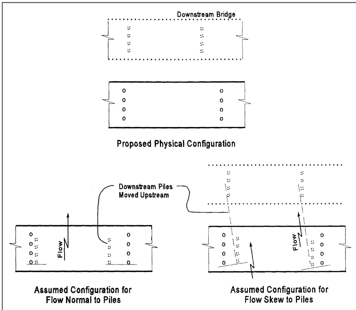
**Figure 5.1-9: Configurations for Computing Scour of Dual Bridges**
