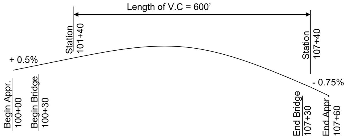
The ground beneath the bridge is less than 25 feet below the bottom of the bridge deck for a distance of 50 feet from each bridge end. Determine the required deck drainage features.
