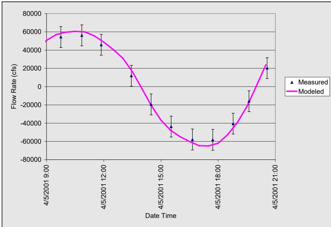
**Figure 5.7-8: Flow Rate Calibration at Lake Worth Inlet
