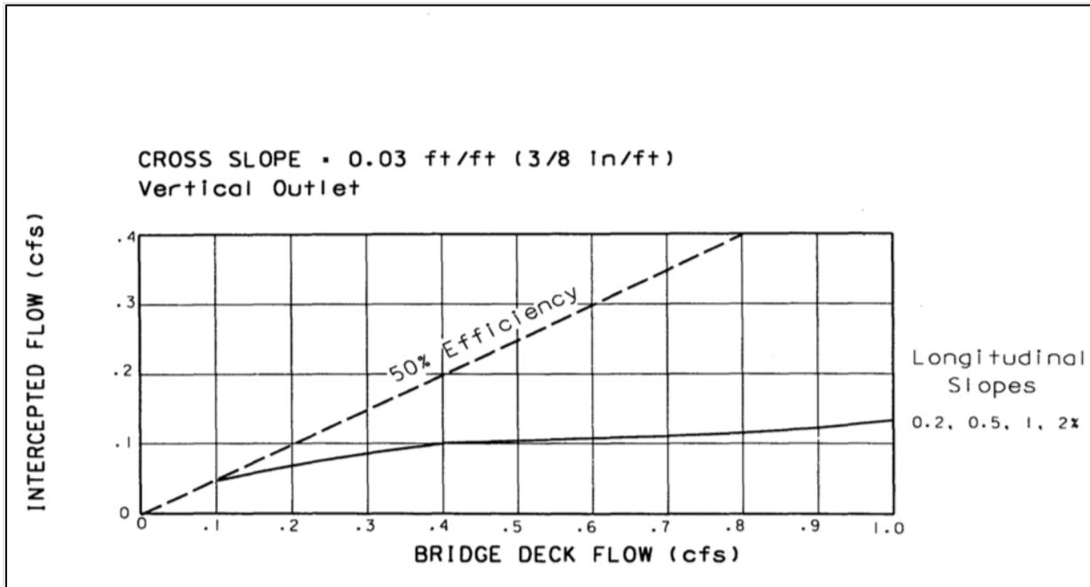
**Figure 5.6-3: Intercepted Flow for 4-inch Bridge Scuppers
