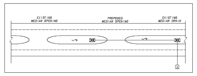
Figure 3.4-5: New Median Drainage System
