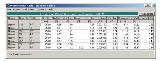
The new flow depth at Section 3 is 1.81 - 0.575 = 1.24 feet. The profile in the narrow section has essentially converged to normal depth (1.25 feet). The depth of the complete profile is shown below:
