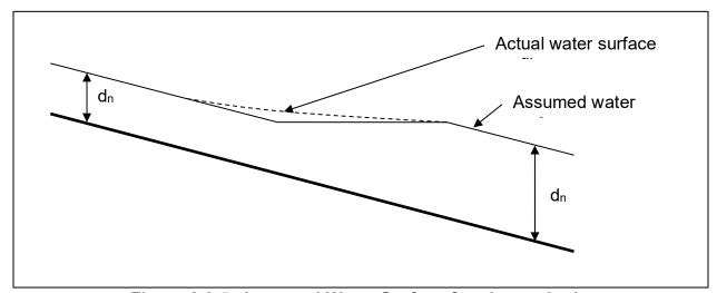
Figure 3.2-5: Assumed Water Surface for change in dn
