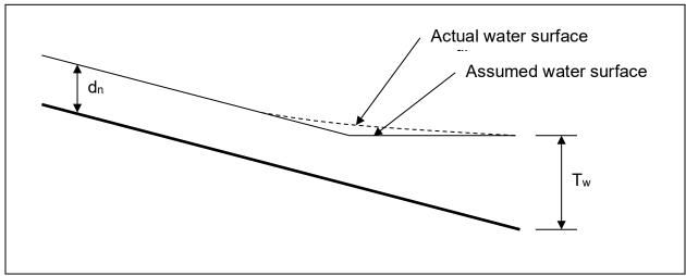
Figure 3.2-3: Assumed Water Surface for Tw > dn
