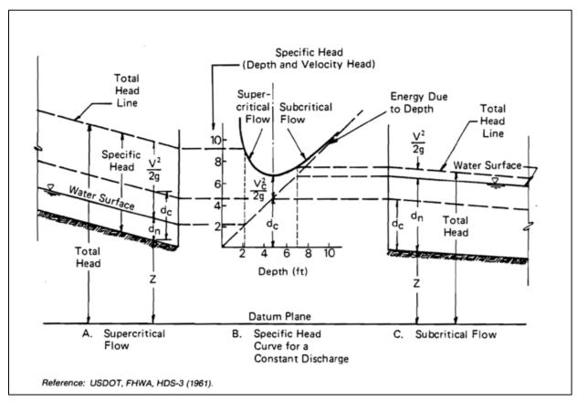
Figure 3.1-2: Definition Sketch for Specific Head and Sub-Critical and Super-Critical Flow
