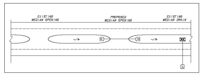
Figure 3.4-3: New Median Opening with Side Drain
