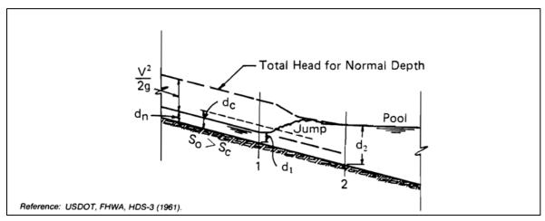
Figure 3.1-5: Non-Uniform Water Surface Profile Caused by a Hydraulic Jump
