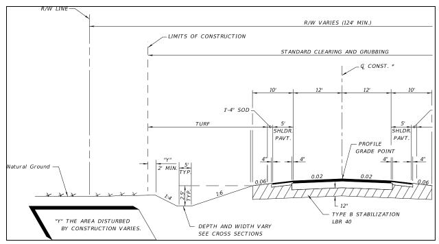
Figure 3.2-1: Typical Ditch for Two-Lane Rural Roadway
