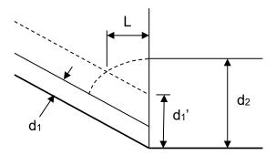
Assuming a more conservative approach, you can split the length of the hydraulic jump between the two regions and provide rubble riprap ditch protection for 20 feet downstream.
