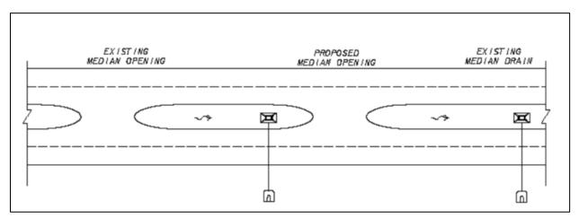
Figure 3.4-4: New Median Drain
