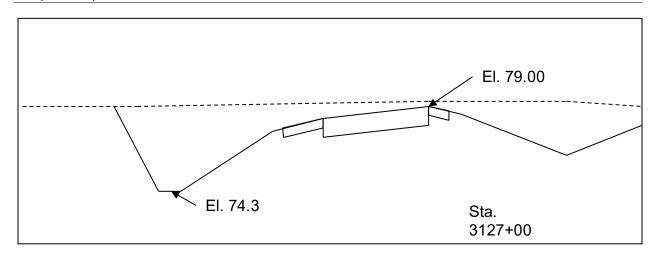
The PGL is flat (0.000 percent) between this cross section and the end section at Station 3126+50. The minimum slope of the ditch is 0.05 percent, and the ideal slope is at least 0.1 percent. Therefore, you will need a special ditch grade between these stations. If the flowline at the headwall (Station 3126+50) is set at 74.2 feet, the ditch grade between these stations will be 0.1/50 = 0.002, or 0.2 percent.
