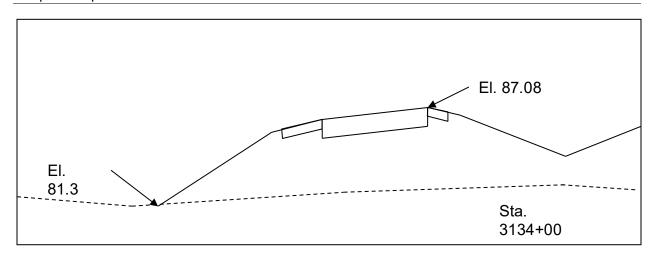
The standard ditch could be used if a berm was constructed. However, there are at least two reasons not to construct the berm. First, some offsite flow to the ditch would be blocked. Second, the cost of constructing the berm is unnecessary since you can use a special ditch profile to lower the ditch into the natural ground.
