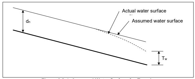
Figure 3.2-4: Assumed Water Surface for Tw < dn
