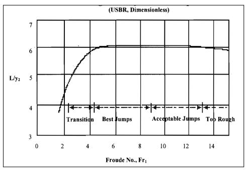
Figure 3.1-7: Lengths of Hydraulic Jumps
