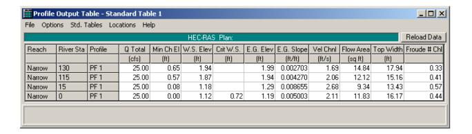
To compare the results with the spreadsheet solution, the depth of flow must be calculated from the water surface elevation.
