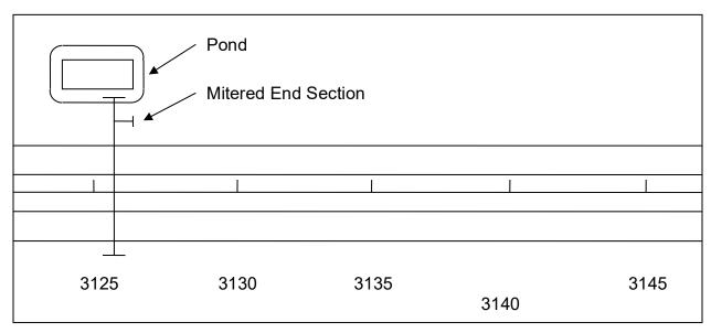
**Step 1—Drainage Plan.** On the left side of the roadway near Station 3125+00A, there is a stormwater pond to treat and attenuate the roadway runoff. Roadside ditches will collect the runoff from the roadway and convey it to the cross drain, which empties into the pond. The offsite drainage area is small; therefore, dual ditches are not needed to reduce the size of the pond.
