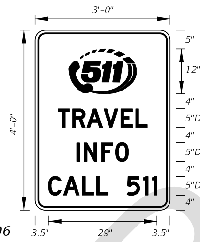
FTP-61-06 3' X 2' 3" Radii 3/4" Border 4" and 3" Series C Legend Yellow Background Black Legend and Border
