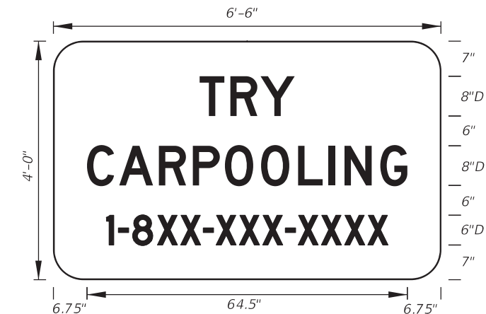
FTP-56-06 6'-6" X 4' 6" Radii 3/4" Border 8" and 6" Series D Legend Blue Background White Legend and Border Design Project Manager or Transit Administrator will supply correct 1-8XX number.
