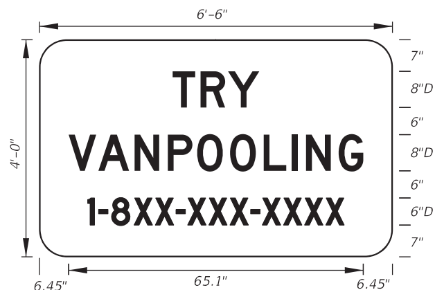
FTP-57-06 6'-6" X 4' 6" Radii 8" and 6" Series D Legend Blue Background White Legend and Border Design Project Manager or Transit Administrator will supply correct 1-8XX number.
