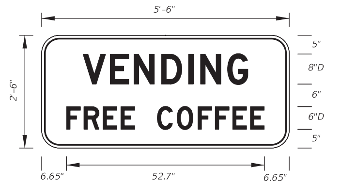
FTP-74-06 5'-6" X 2'-6" 4" Radii 3/4" Border 6" Series D Legend Blue Background White Legend and Border
