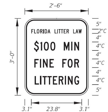
FTP-41-06 2'-6" X 3' 4" Radii 3/4" Border 2" and 4" Series C Legend White Background Black Legend and Border
