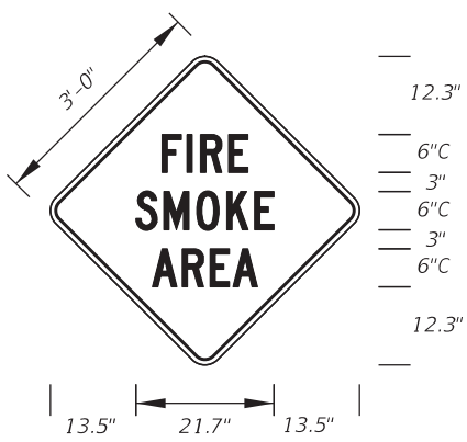
FTP-72-06 3' X 3' 2" Radii 3/4" Border 6" Series C Legend Yellow Background Black Legend and Border
