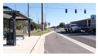
The two photos above are from the same roadway and illustrate an example of a high-volume roadway that balances the needs of freight traffic, transit, and pedestrians and bicyclists of varying abilities. The corridor includes a shared use path, bicycle lanes, bus pull-outs, bus shelters with benches, and other amenities. Location: US 98, Polk County, FL Source: KAI
