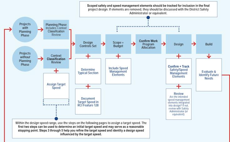
The target speed should be identified by a multidisciplinary group of engineers and planners. This group can work together to set the target speed and make sure the elements identified to achieve the target speed are carried through scoping, design, and implementation.
