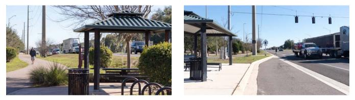
The two photos above are from the same roadway and illustrate an example of a high-volume roadway that balances the needs of freight traffic, transit, and pedestrians and bicyclists of varying abilities. The corridor includes a shared use path, bicycle lanes, bus pull-outs, bus shelters with benches, and other amenities. Location: US 98, Polk County, FL Source: KAI
