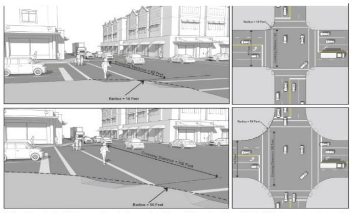
Curb radii has significant influence on the pedestrian crossing distance at intersections. Top and bottom illustrations compare the crossing distances between an intersection with 50 feet and 15 feet curb radius.
