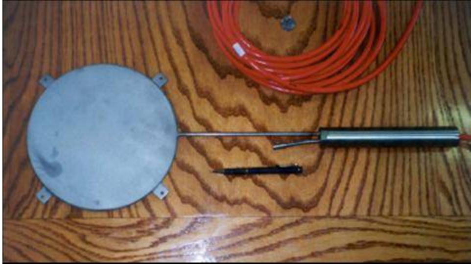
Figure 2-10. Typical soil pressure sensor.
