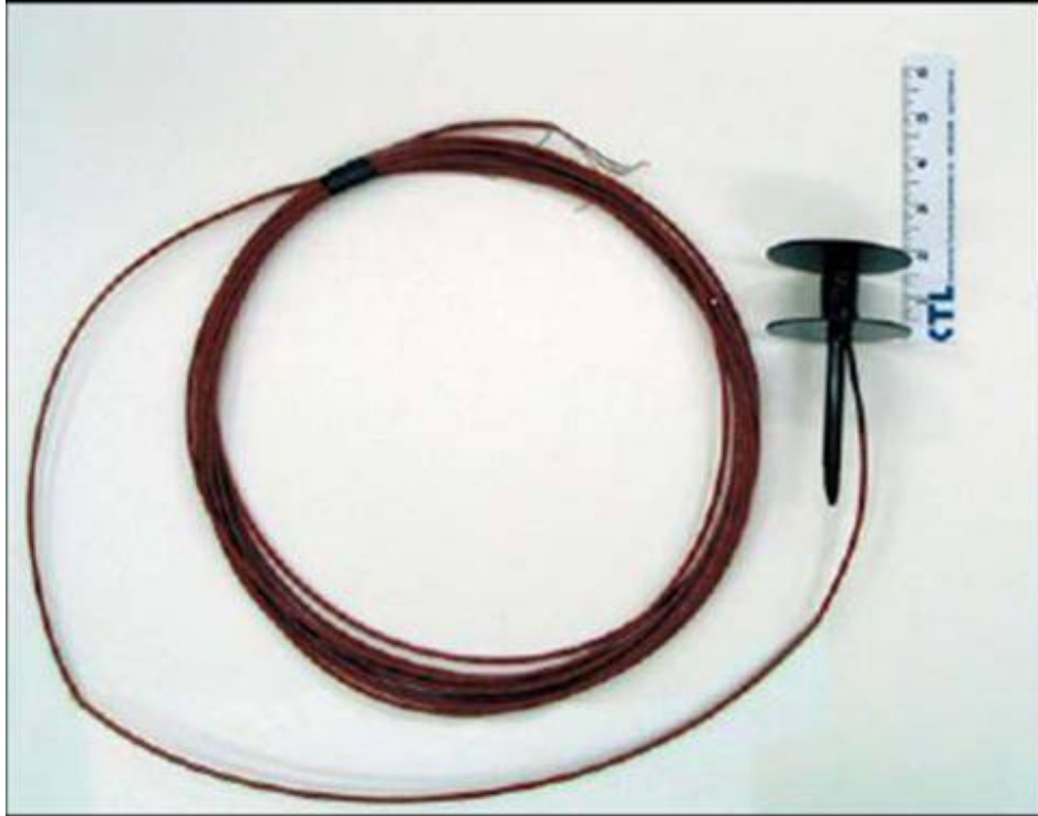
Figure 2-2. CTL asphalt vertical strain sensor.
