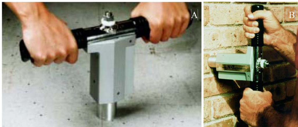
Figure 0-5 Windsor Pin System ® On: A) Smooth Surface; B) Mortar Joint (NDT James, 2006)
