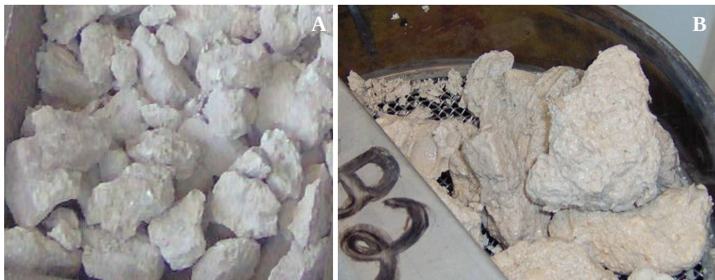
Figure 0-3 Sulfate Soundness Result for Limestone (TYP); A) Before; B) After
