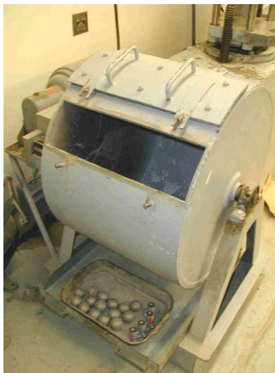
Figure 0-4 Typical L. A. Abrasion Tumbler (SuperPave)
