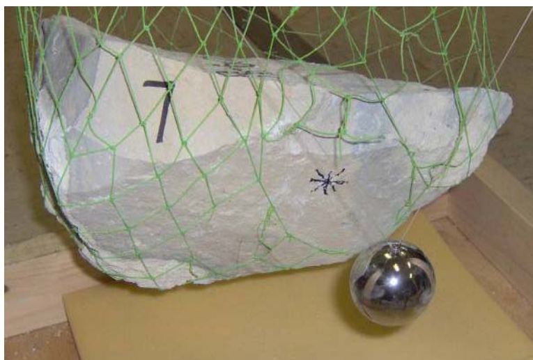
Figure 0-2 Example of Asterisk Denoting Impact Identification Point
