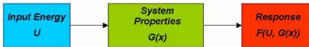
Figure 0-1 Simple Transfer Function Block Diagram
