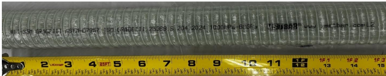
Figure 26. FRP straight bar #11 manufactured by MST-Bar.
