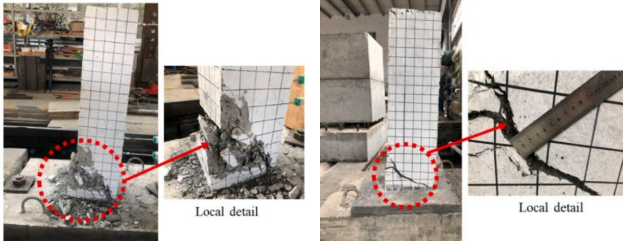
(a) Failure of RC column
