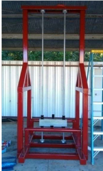
Figure 7- 2 Drop weight impact apparatus
