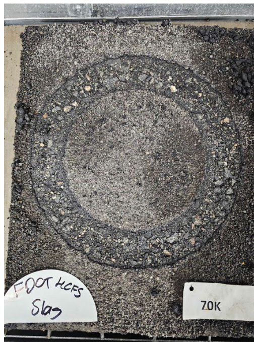
Figure 23: Failed HFCS Slab with Slag Aggregate
