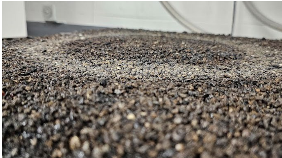
Figure 42: Roughness of the Bauxite HFCS Slab
