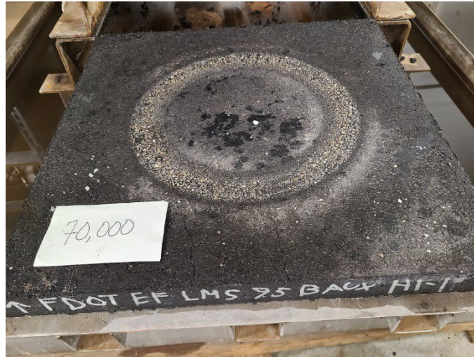
Figure 38: Raveling of LMS FC-9.5 Bauxite (High) Slab
