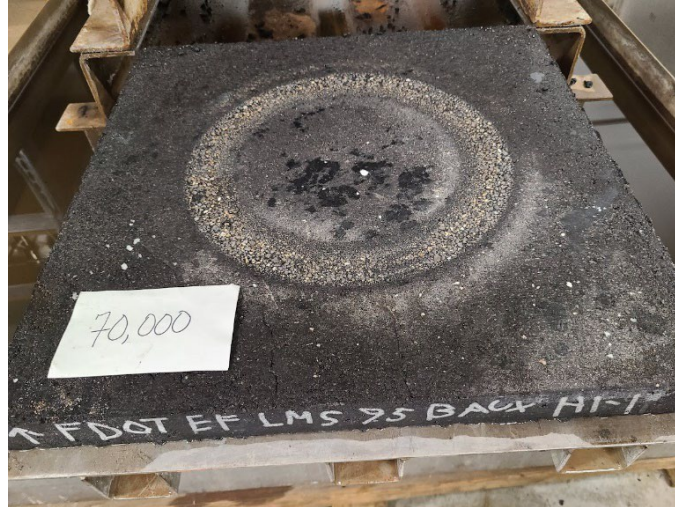
Figure 38: Raveling of LMS FC-9.5 Bauxite (High) Slab
