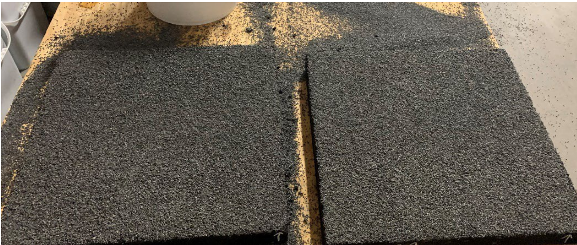
Figure 6: Stalite Lightweight Aggregate as HFST on a Slab (NCAT)
