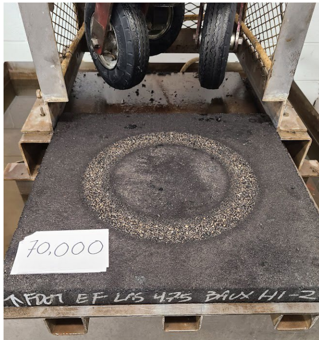
Figure 21: Slab after Polishing
