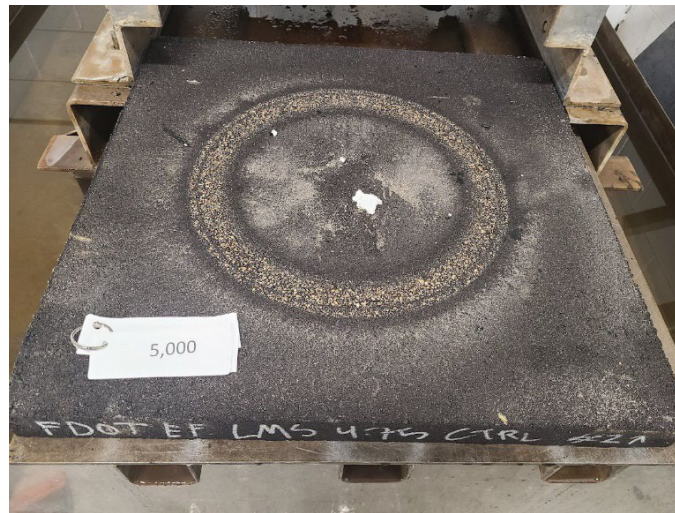
Figure 35: Initial Raveling of LMS FC-4.75 Slab at 5,000 TWPD Cycles
