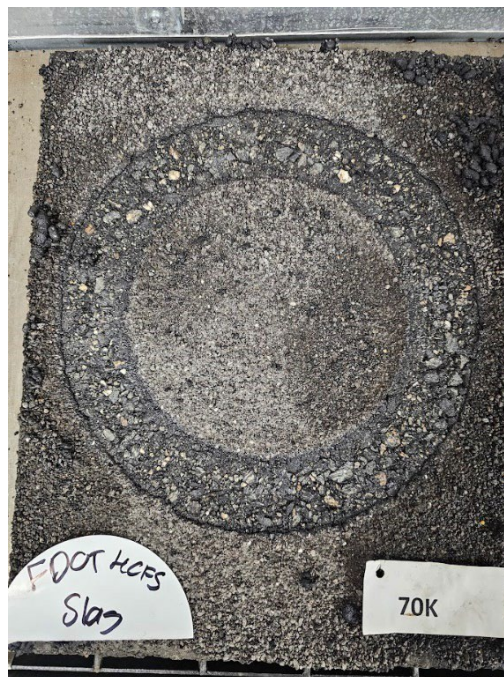
Figure 23: Failed HFCS Slab with Slag Aggregate
