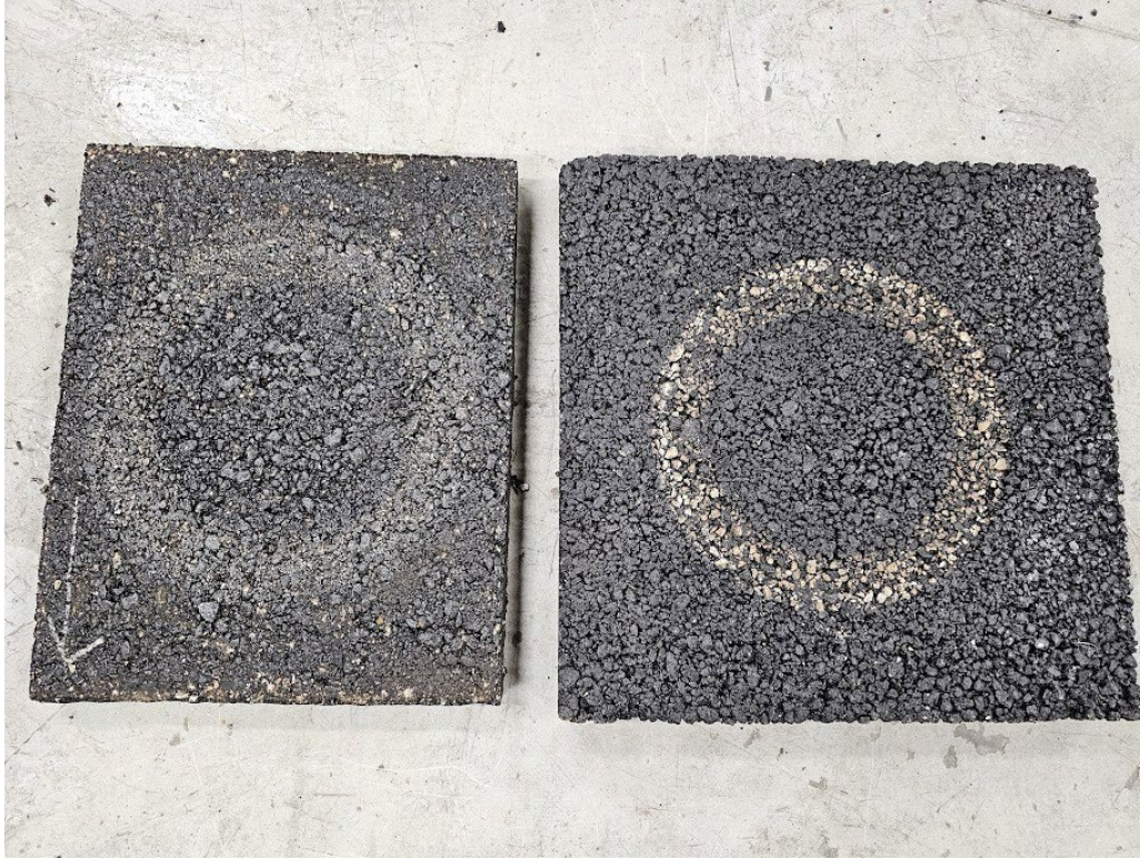
Figure 17: Comparison of Slab Sizes between Compactor Types – (Left: A.R.C; Right: NCAT)
