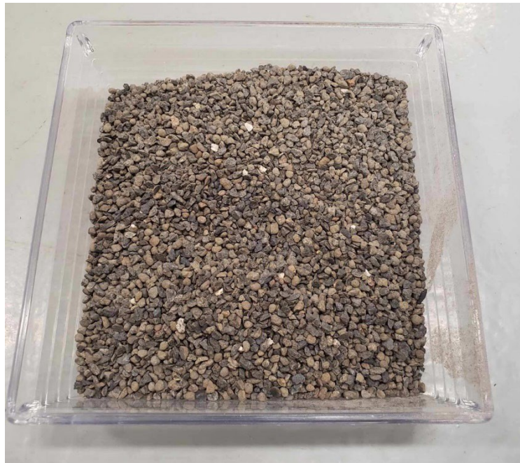
Figure 8: Sample of Calcined Bauxite from Eufala, Alabama
