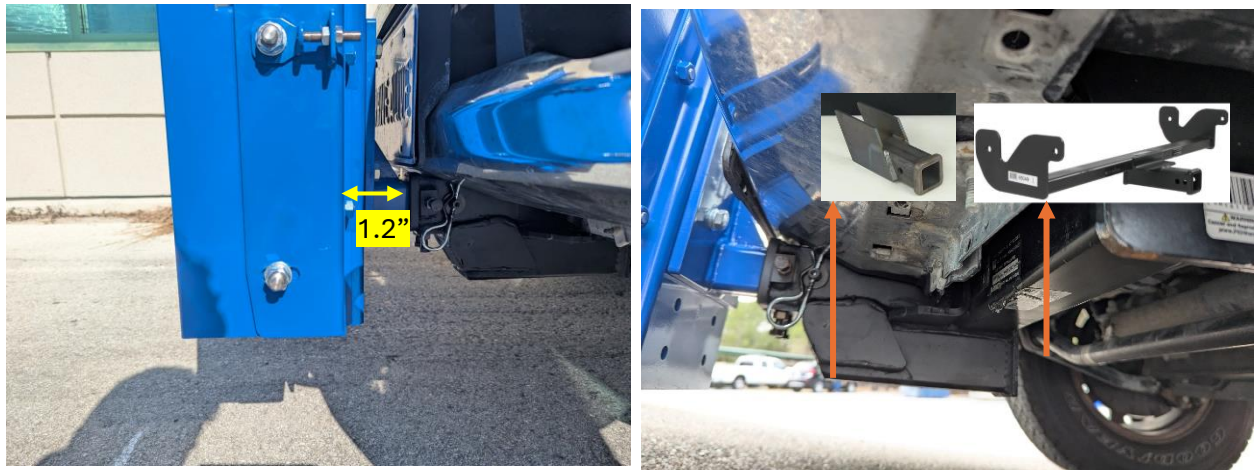
Figure 2.1 Modification made to the FDOT truck to install the mounting bracket for DRS
