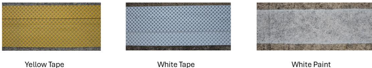
Figure 1.16 Different pavement marking samples used in the study by Pike et al. [10].
