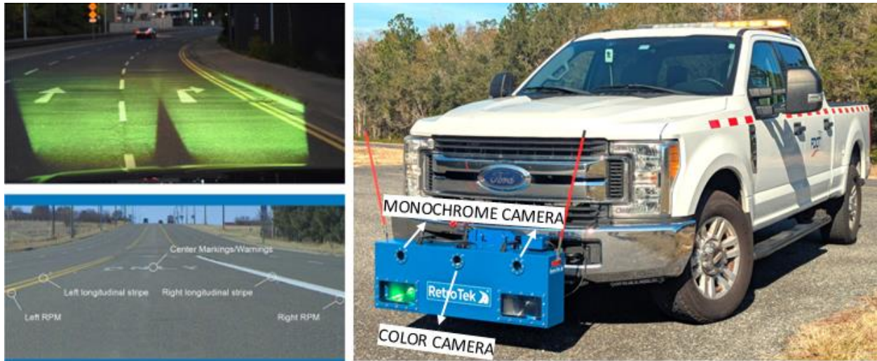
Figure 1.12 RetroTek DRS front-mounted on a vehicle capable of detecting pavement marking characteristics across the full lane width in a single pass.
