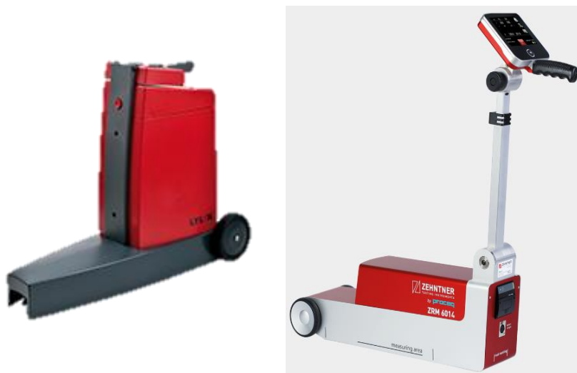
Figure 5.3 FDOT's handheld retroreflectometers (LTL-X on the left, Zehntner on the right)
