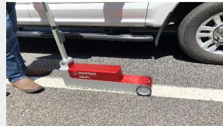
Figure 4.30 The testing details for the handheld measurements: (A) measurement points, (B) distance for skip lines, (C) Delta LTLX and Zehntner handhelds retroreflectometers
