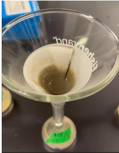
Figure 43. Rinsing residue from sides of filter paper
