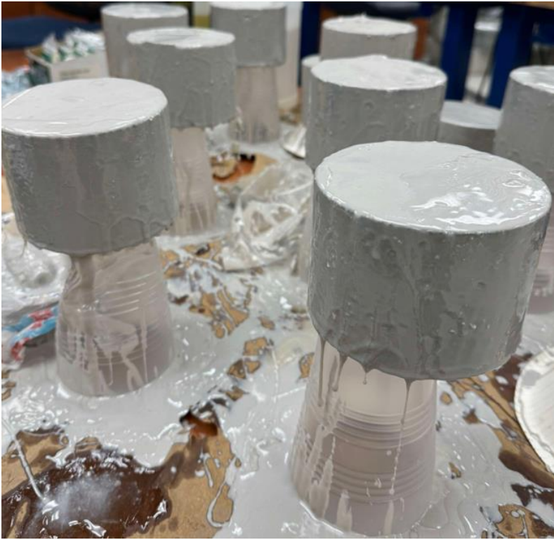
Figure 25. Samples coated with epoxy
