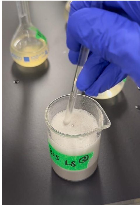
Figure 40. Dispensing 5% nitric acid and stirring until minimal frothing
