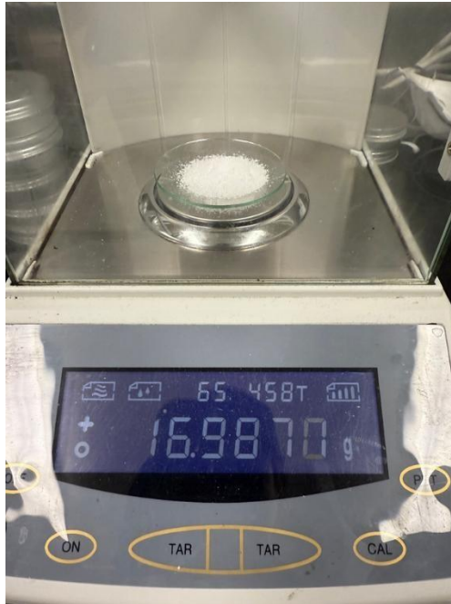
Figure 34. Silver nitrate particles weighed on analytical balance
