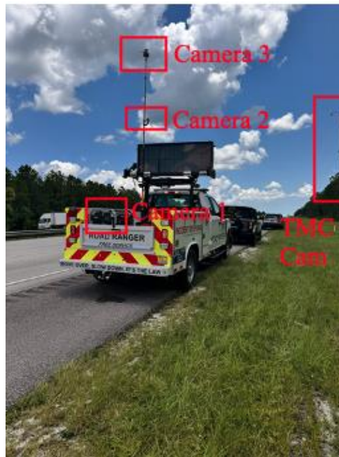
Figure 14: Roadside camera setup
