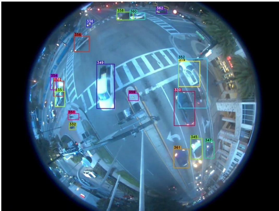
Figure 8-28 – False detection of the fisheye camera (ID 359)
