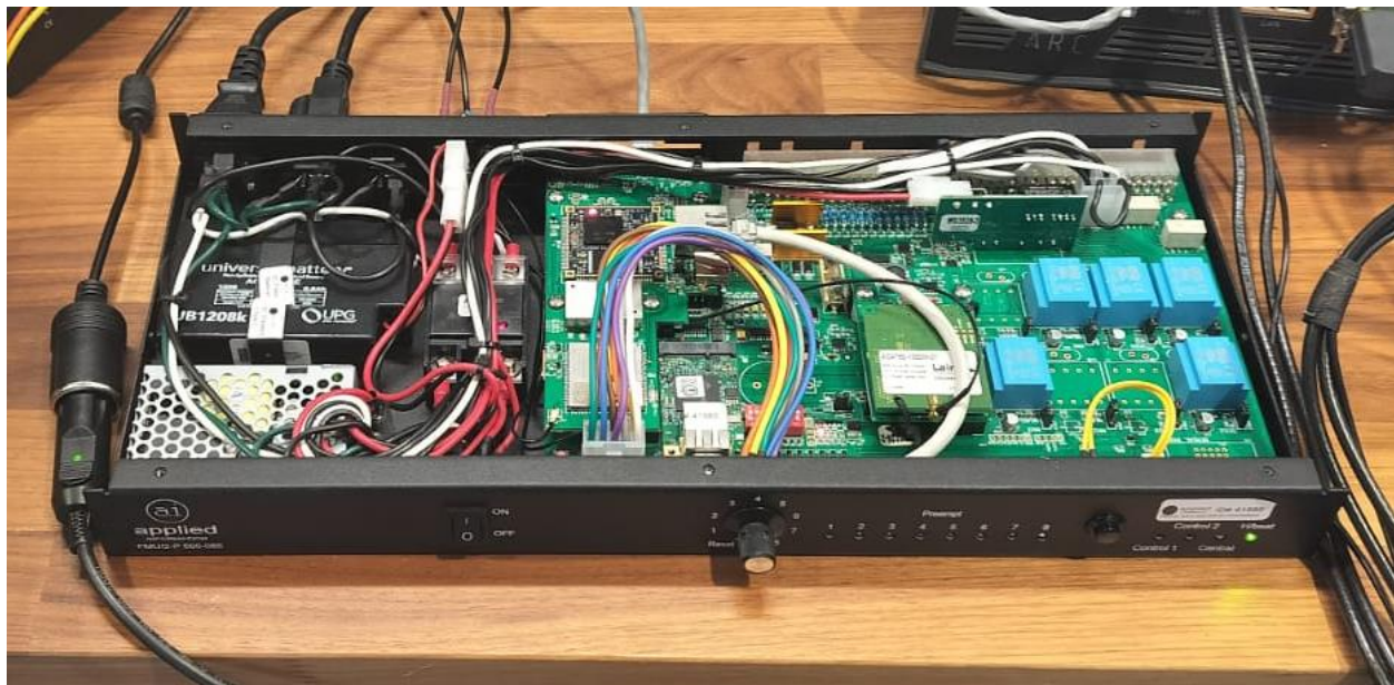
Figure 5-19 – A field-monitoring unit (FMU) used in the study area
