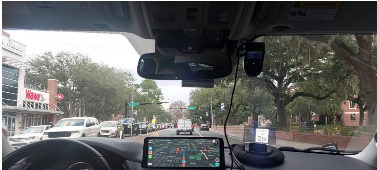
Figure 5-14 – Speed limit message received by OBU
