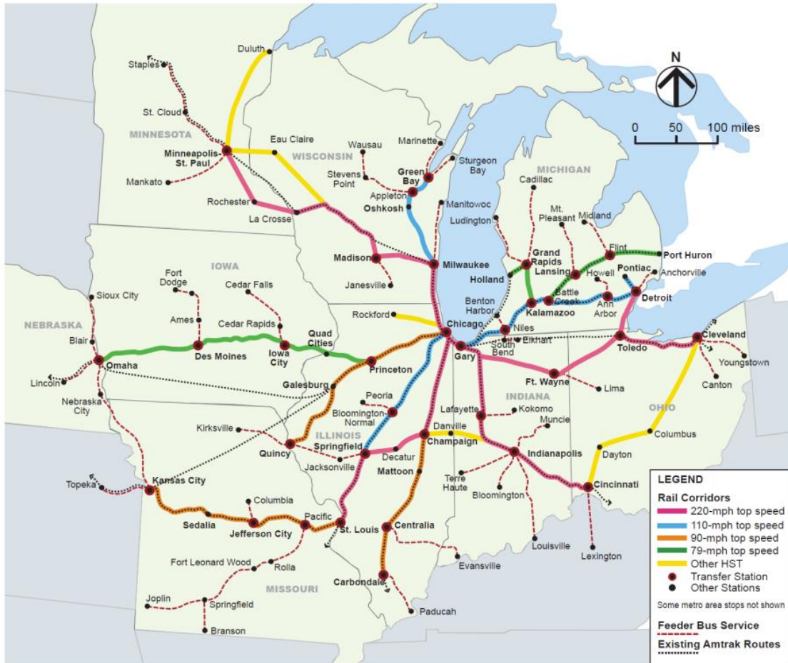
Figure 4-3. Concept plan for the Midwest region’s high speed rail network. Adapted from MHSRA (2011).
