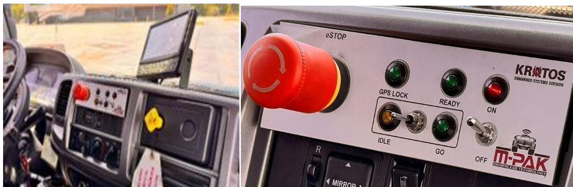
e) The RCTMA dash (left) showing OCU (detail, right)
