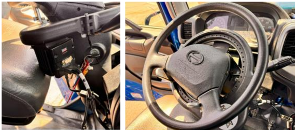
d) Left – Side view of steering actuator; right – mechanical coupling: steel “fingers” (arrows) and ring
