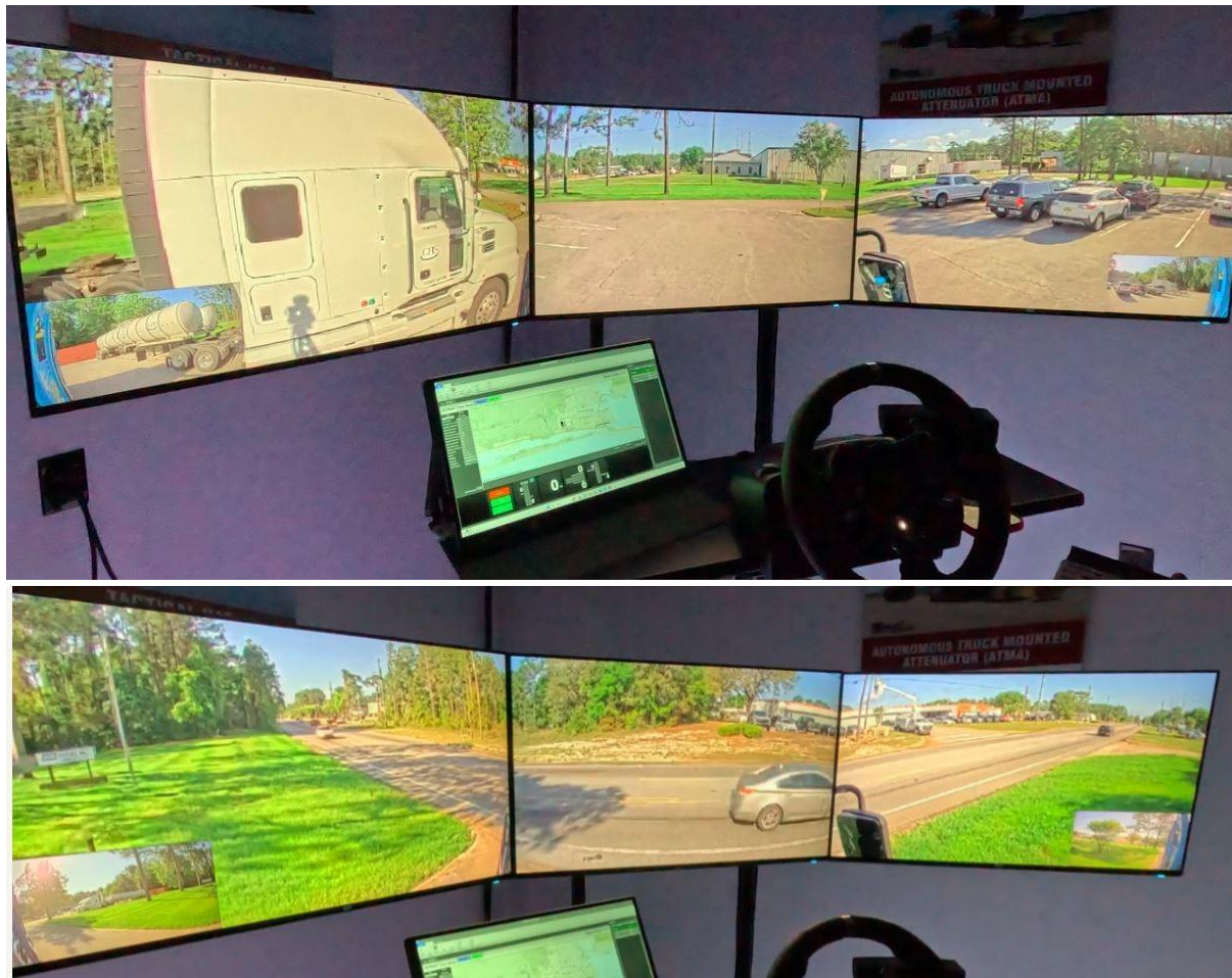
Figure 27. C2 monitors: three 27-inch monitors provide the C2 driver with a more than 180-degree forward view and rear views (PIP insets) along either side of the RCTMA.
