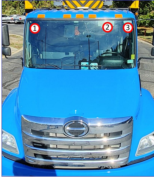
Figure 18. RCTMA Three Front-Facing Camera Locations
