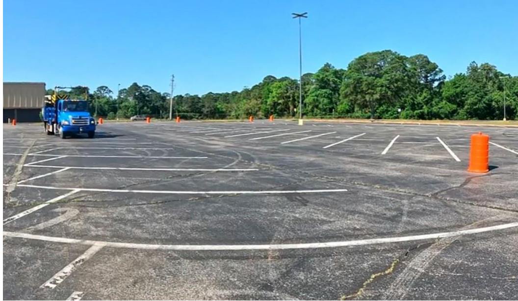
Figure 37. RCTMA positioned to begin the braking test in motion
