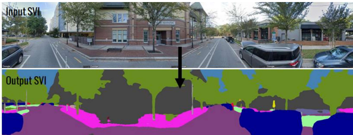
Figure 6-1 A showing of model input and output images of the pspnet101_cityscapes model
