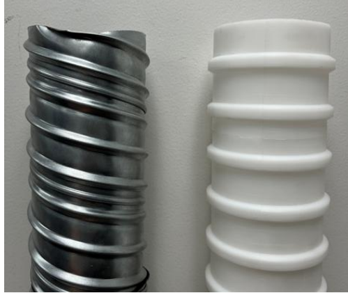
Figure 3.6. Corrugated ducts of different materials and ribs used for post-tensioning: corrugated metal duct on the left and corrugated plastic duct on the right.
