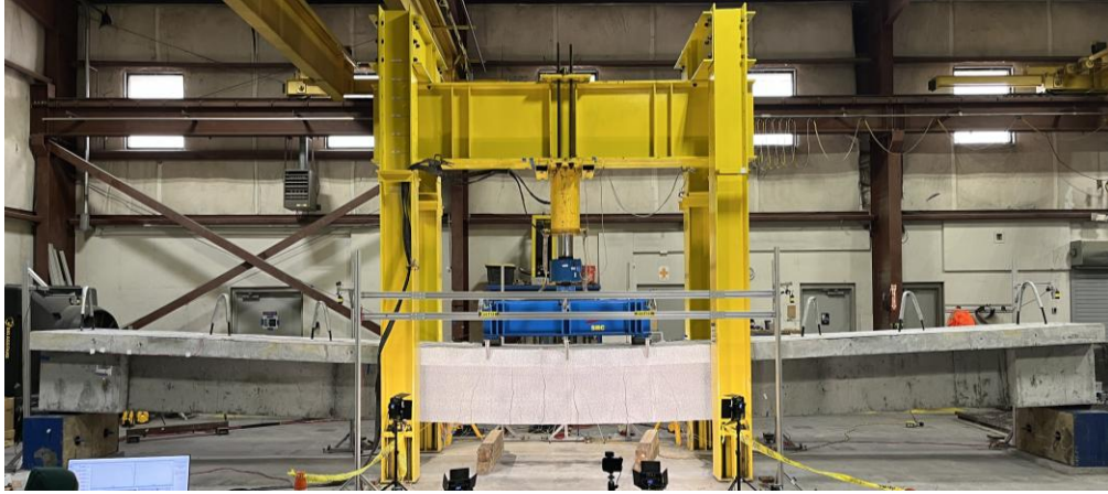
Figure 9.11. Flexural testing of S19-M-T test beam.
