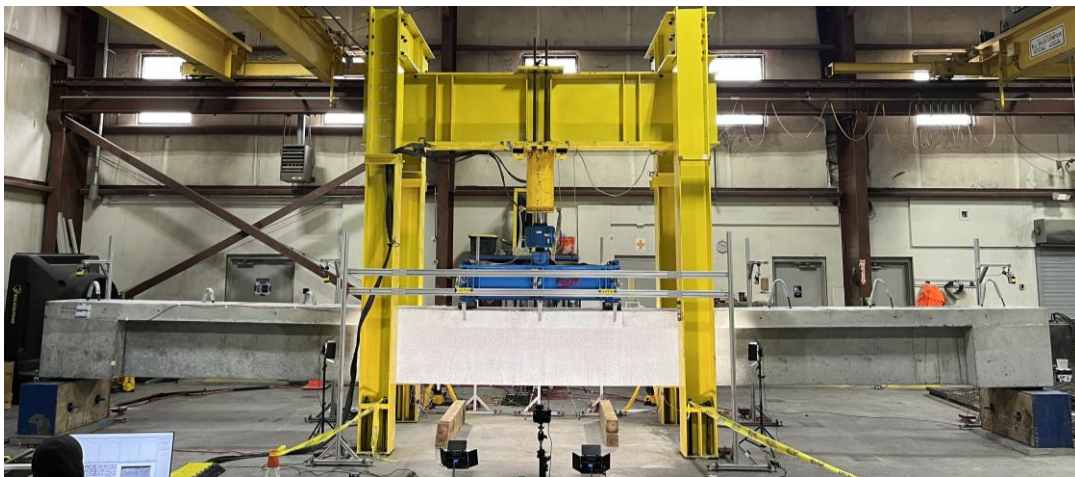
Figure 9.7. Flexural testing of S12-P-T beam
