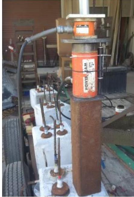
Figure 3.2. Pullout testing of grouted unstressed monostrand tendon (Silnutzer et al. 2020)
