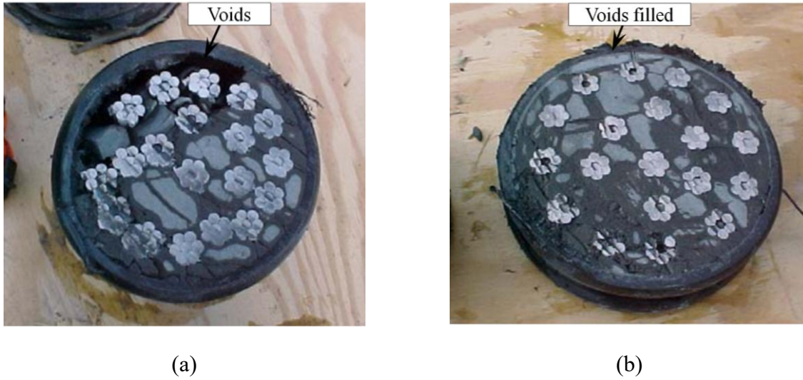
Figure 3.4. Dissected mock-up bonded tendon. Grout injected using: (a) pressure injection; and (b) vacuum injection (Corven 2001)
