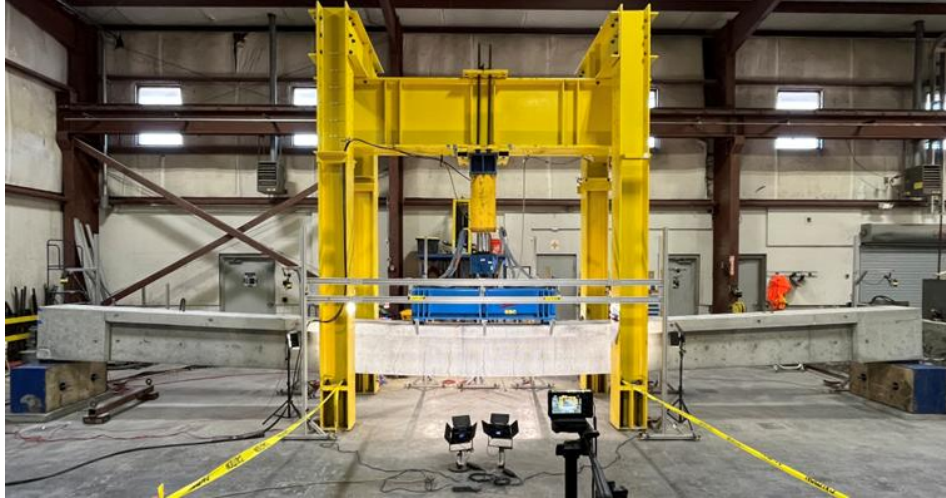
Figure 9.3 Flexural testing of S06-M-T beam
