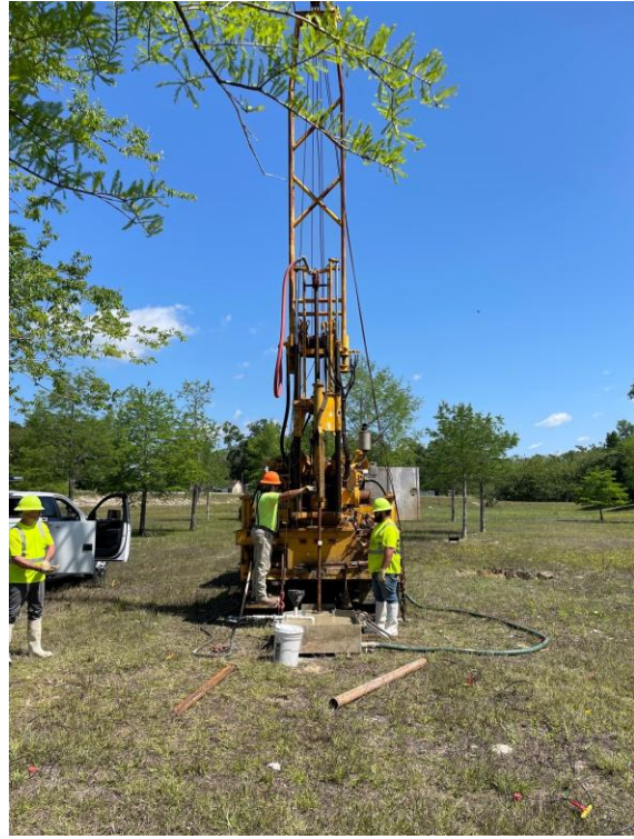
Figure 4.1. Field experiment at Newberry site: (a) two test zones with an SPT at the center of each zone; (b) site photo with the SPT rig
