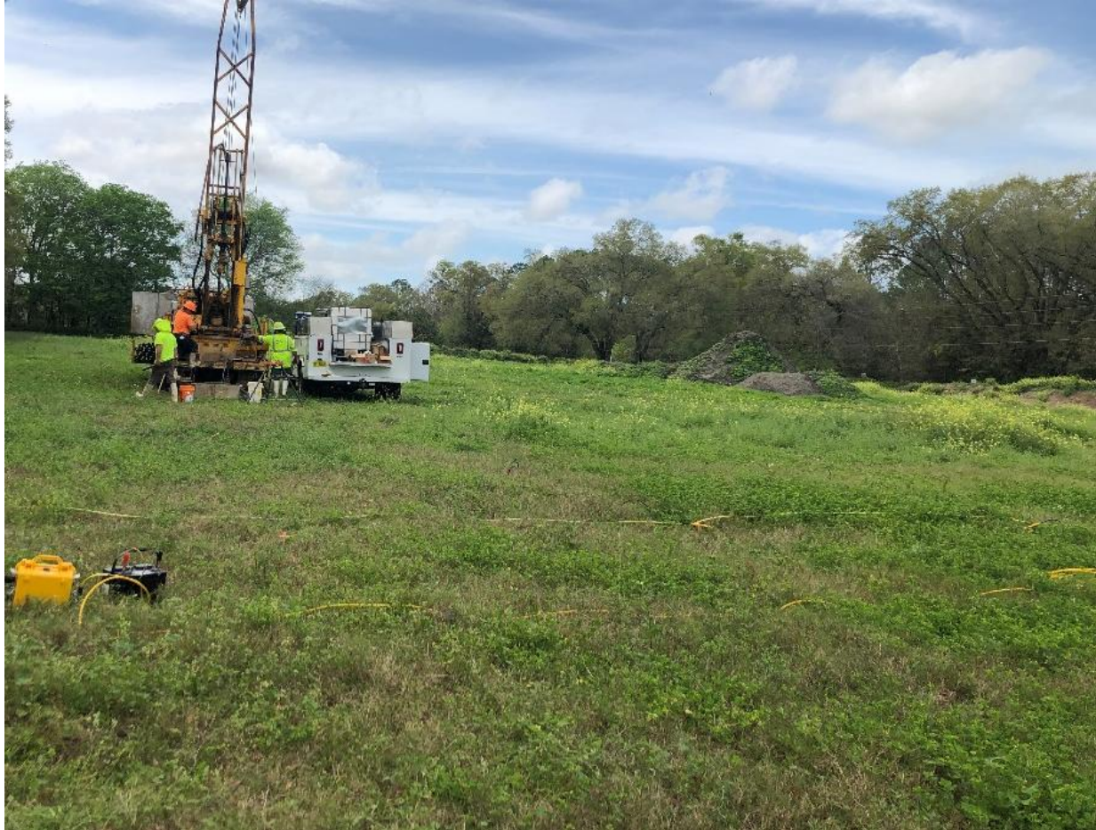
Figure 4.21. Field experiment at Kanapaha site: photo with the SPT rig. The 72 geophones ( 6 \times 12 grid) were placed over a test area of 60 \times 120 ft. The SPT location is at the center of the test area
