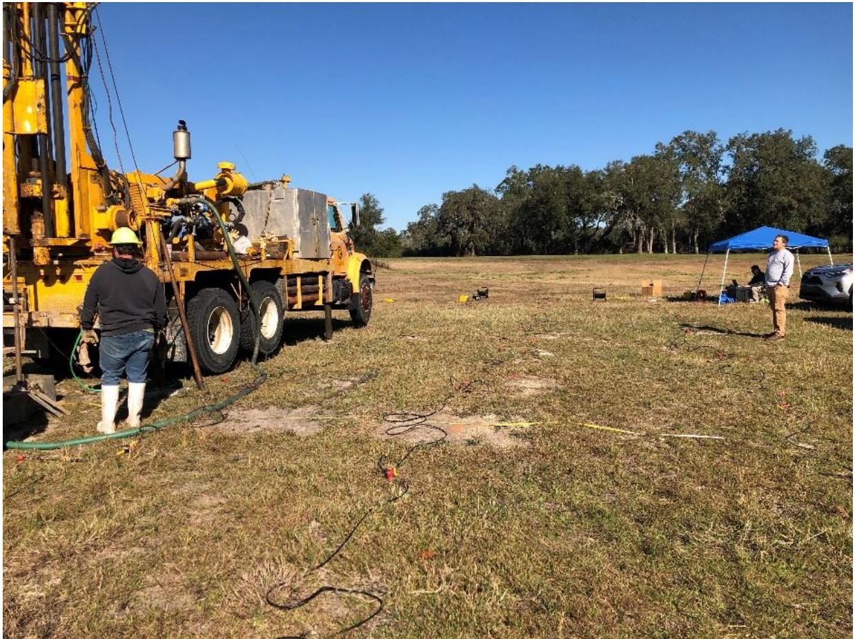
Figure 4.12. Field experiment at Bell site: test site photo with the SPT. The 72 geophones ( 6 \times 12 grid) were placed over a test area of 60 \times 120 ft. The SPT location is at the center of the test area
