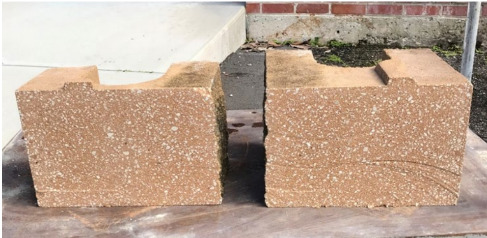
Figure 3-24. Vertical straight face blocks after being wet cut.
