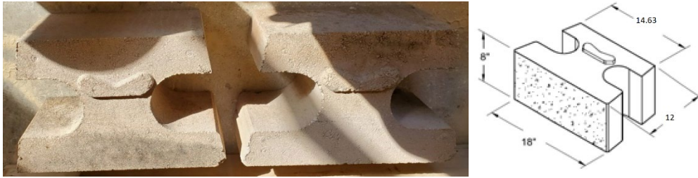
Figure 3-23. Details of the segmental block.
