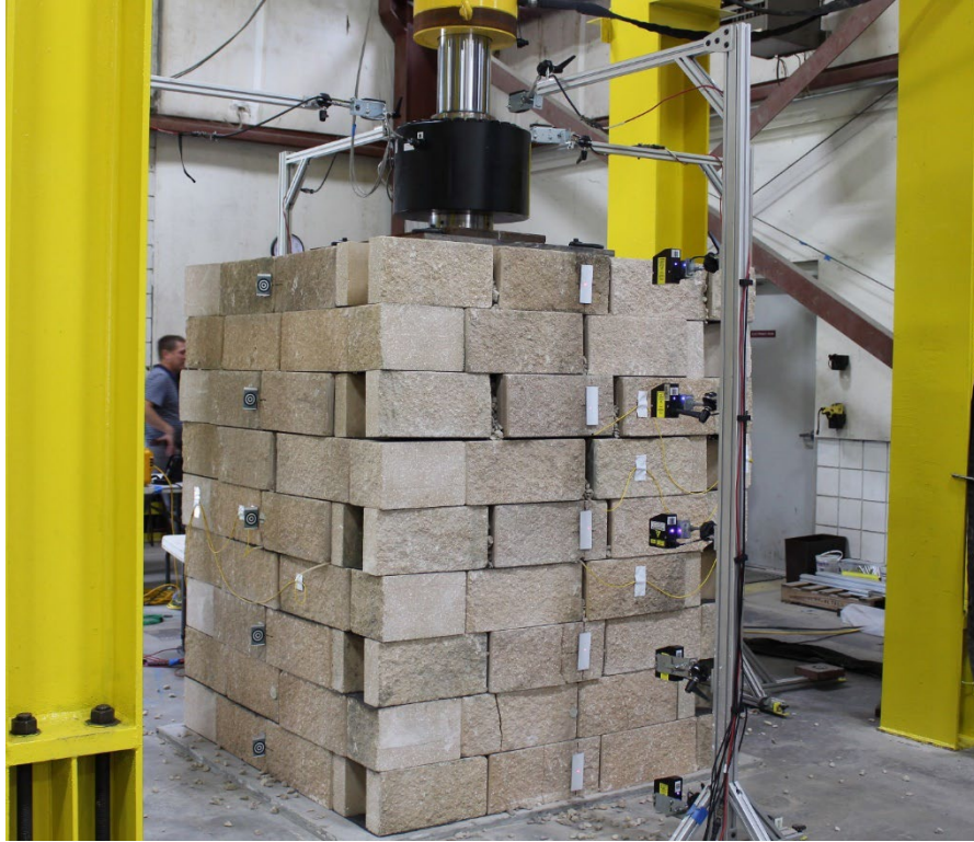
Figure 4-8. A photo of the failed pier after the PT-02 test.
