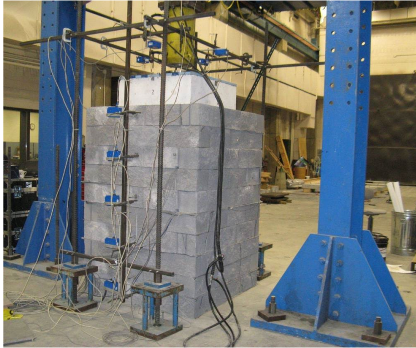
Figure 5-30. Photo of TF-6 PT setup with reaction frame. (Nicks et al., 2013).
