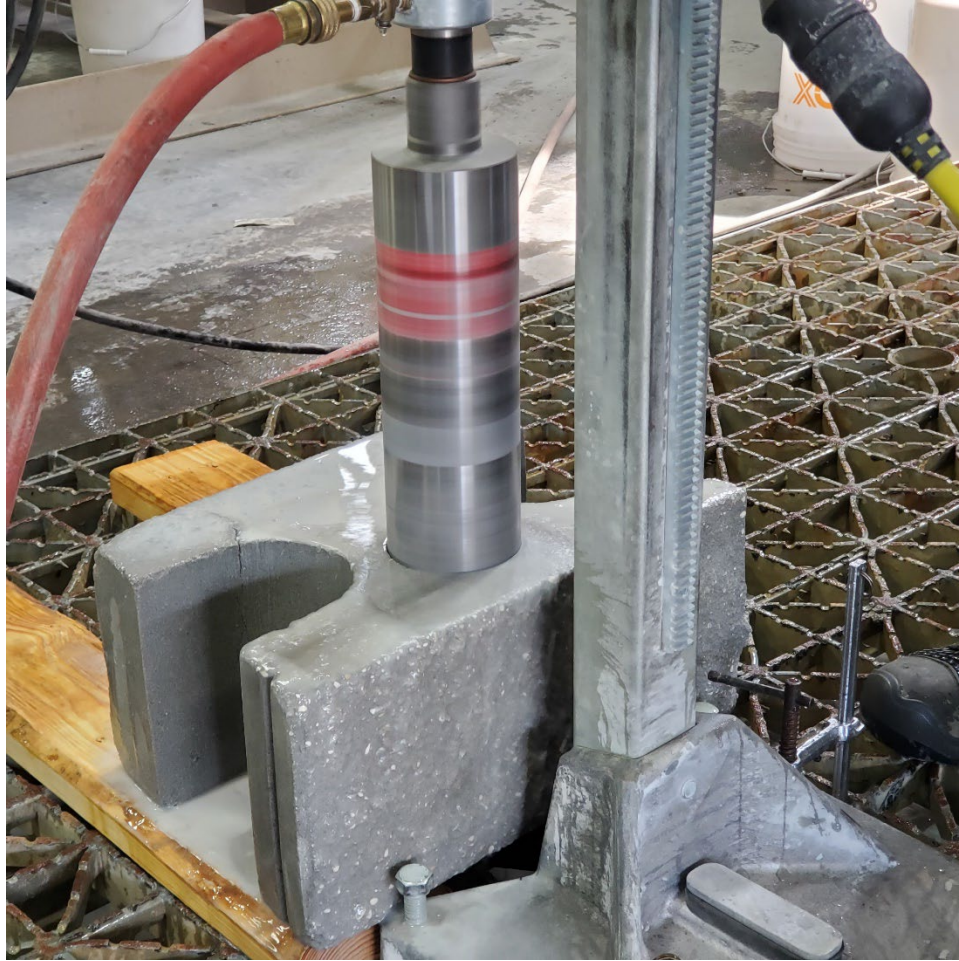
Figure 3-17. Drilling of the block cores.
