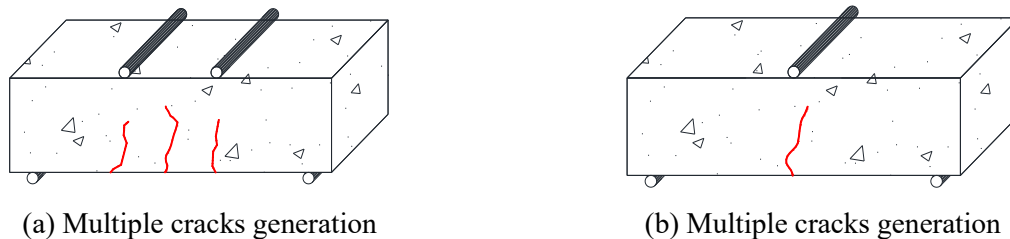
Figure 5-1 Illustration of crack generation by bending test
