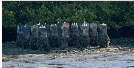
(b) Oyster growth on specimens after 6 months of exposure
