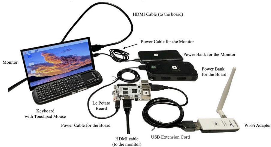
Figure 3-19 Sniffer device assembly diagram
