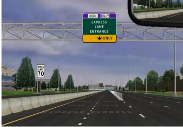
a) Managed Lane entrance with single solid line
