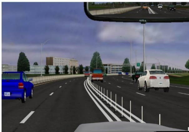
c) Curved section with 24" pylons and double solid lines
