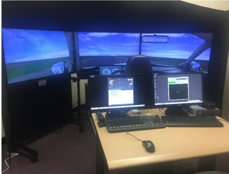
Figure 3.1: UCF miniSim™ Driving Simulator
