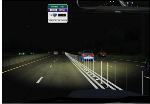
b) Nighttime scenario with 36" pylons and double solid lines
