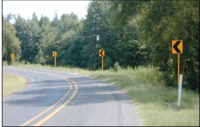
(b) Chevron signs with retroreflective strips on sign posts
