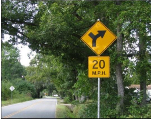
(a) Curve warning sign with advisory speed
