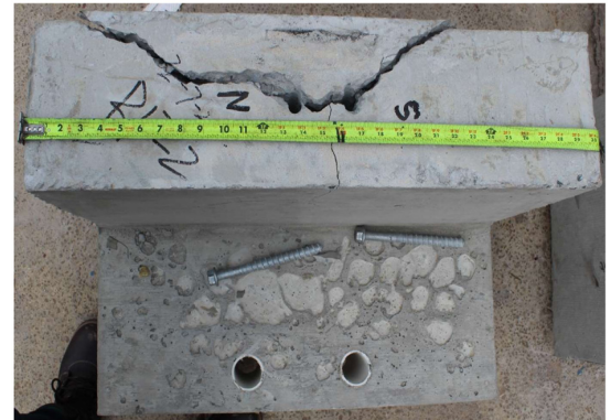
The concrete parapet mockup specimen after breakout of two 5/8-in dia. galvanized screw anchors.
