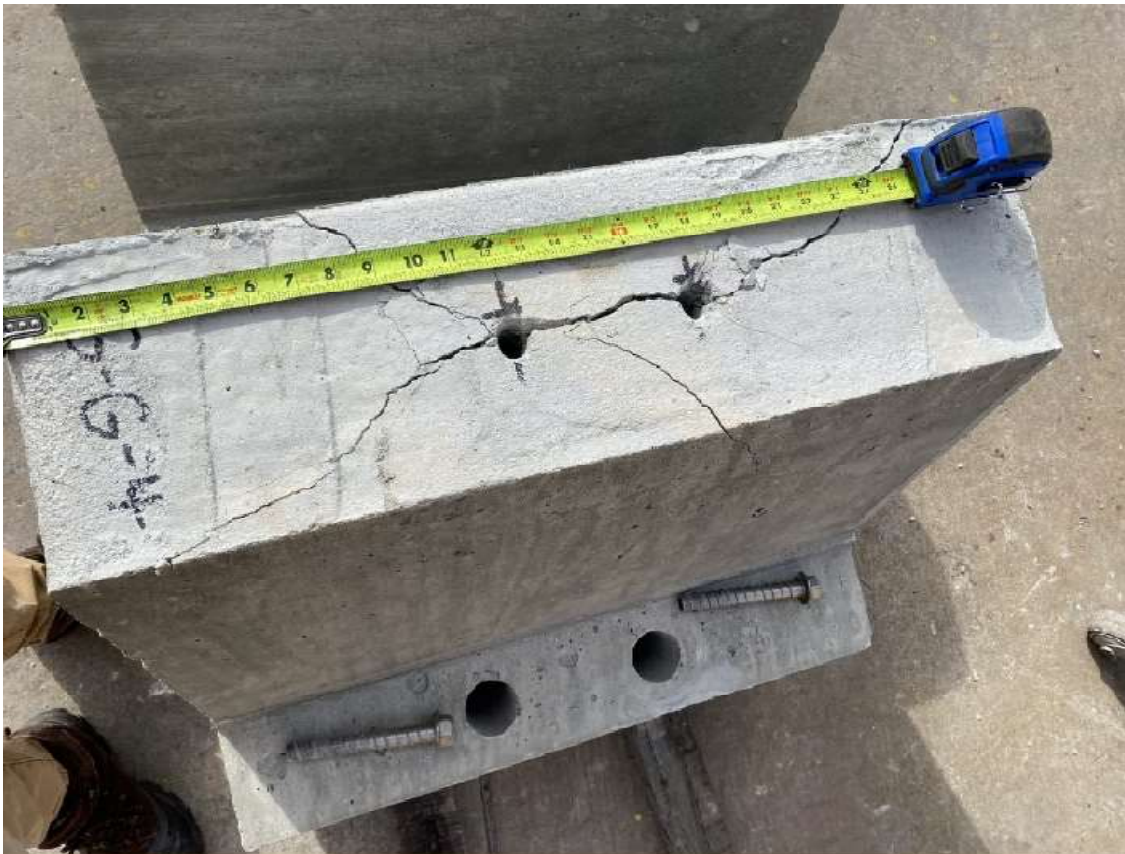
Figure A-85: G-G-4 specimen concrete after screw anchor breakout
