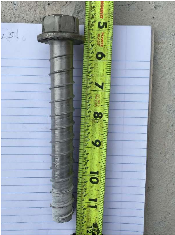
Figure A-57: G-SSc-1 specimen south screw after cyclic loading
