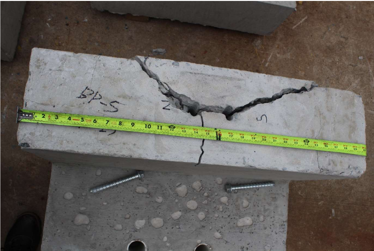
Figure A-105: B-P-5 specimen concrete after breakout
