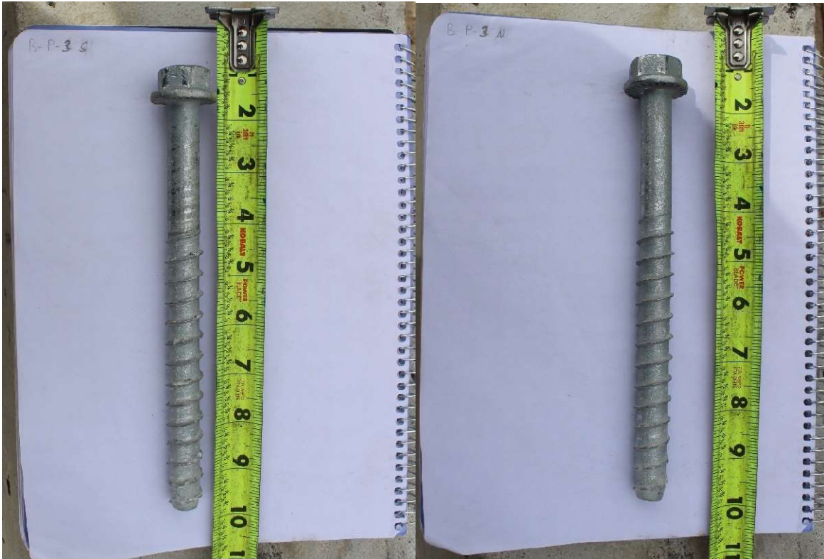
Figure A-100: B-P-3 specimen south and north screw anchor after breakout
