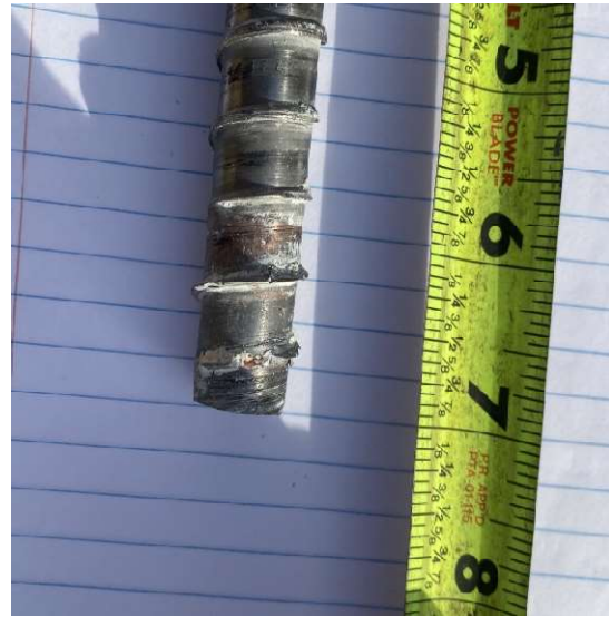
Figure A-75: G-G-1 specimen north screw after breakout
