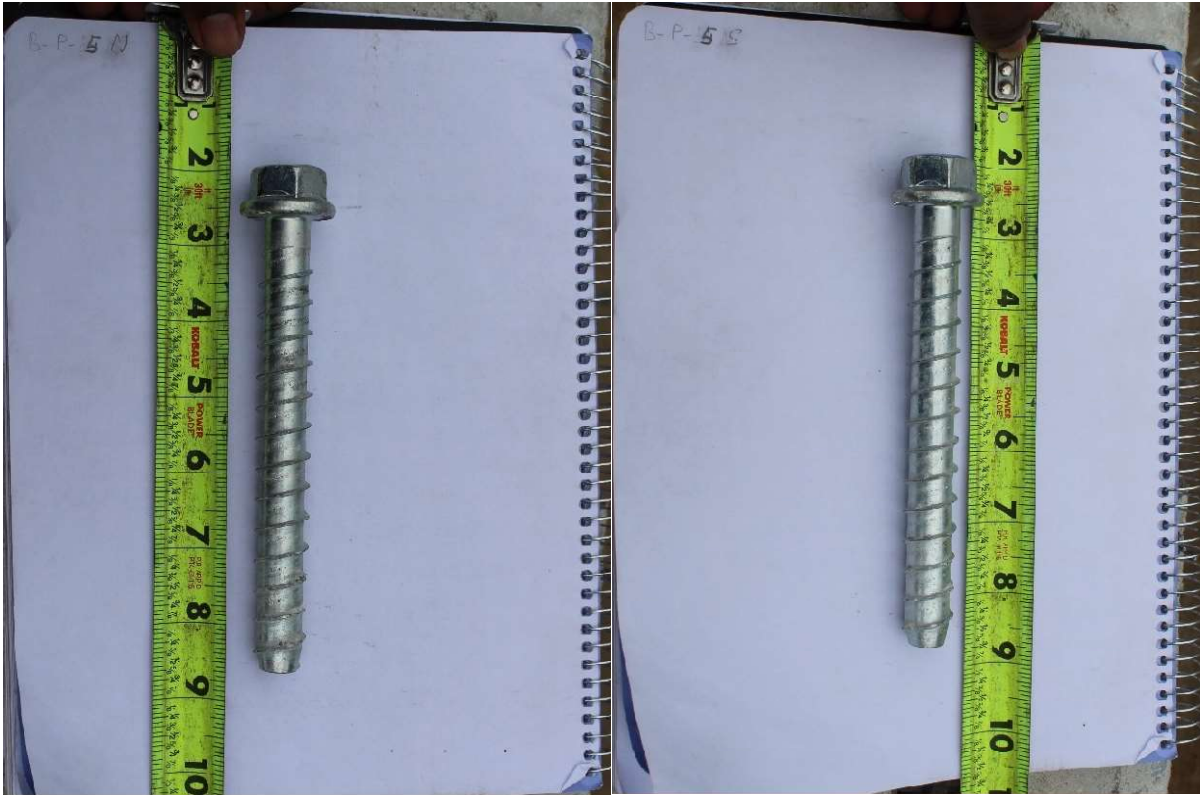
Figure A-104: B-P-5 specimen north and south screw anchor after breakout
