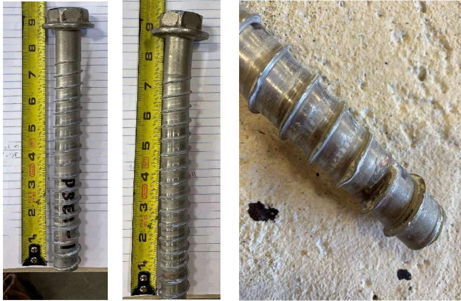
Figure A-5: P-SE1-1 specimen screw after loading
