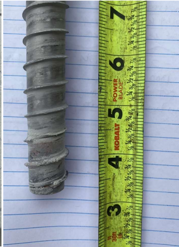
Figure A-65: G-SSc-4 specimen north screw after cyclic loading
