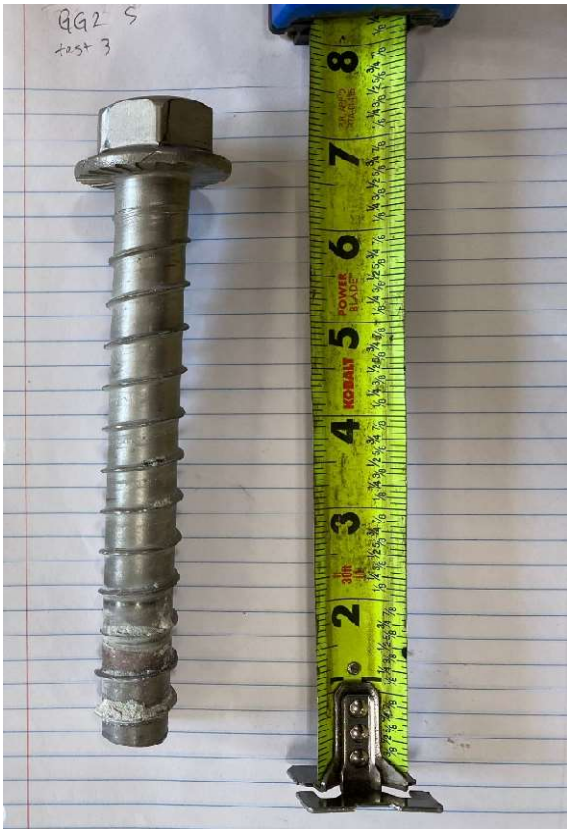
Figure A-79: G-G-2 specimen south screw after breakout
