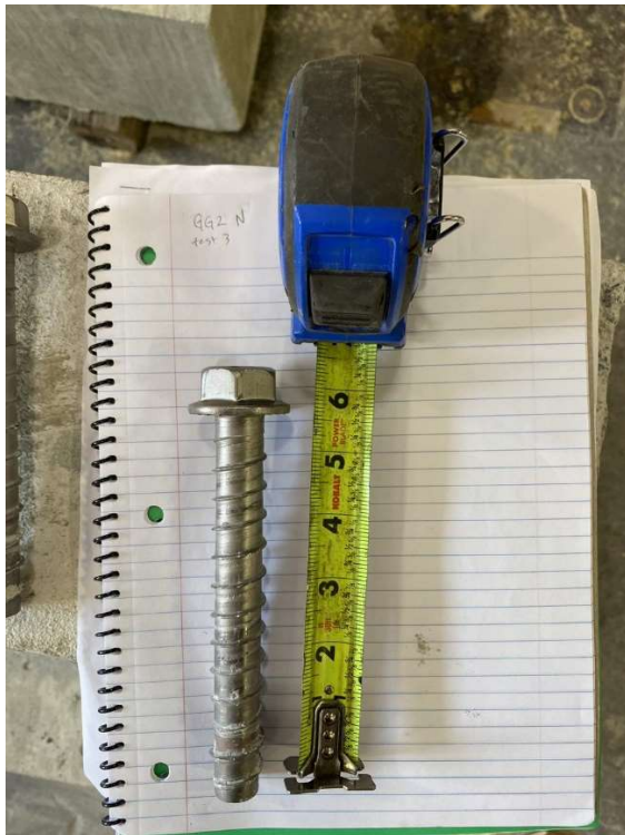
Figure A-78: G-G-2 specimen north screw after breakout
