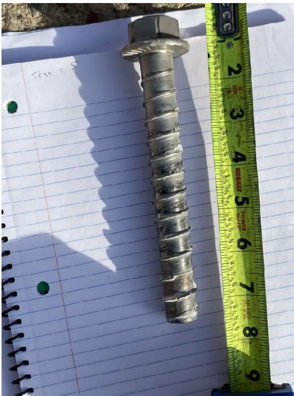
Figure A-76: G-G-1 specimen south screw after breakout
