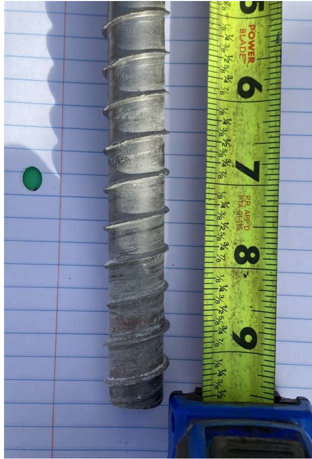
Figure A-81: G-G-3 specimen north screw after breakout
