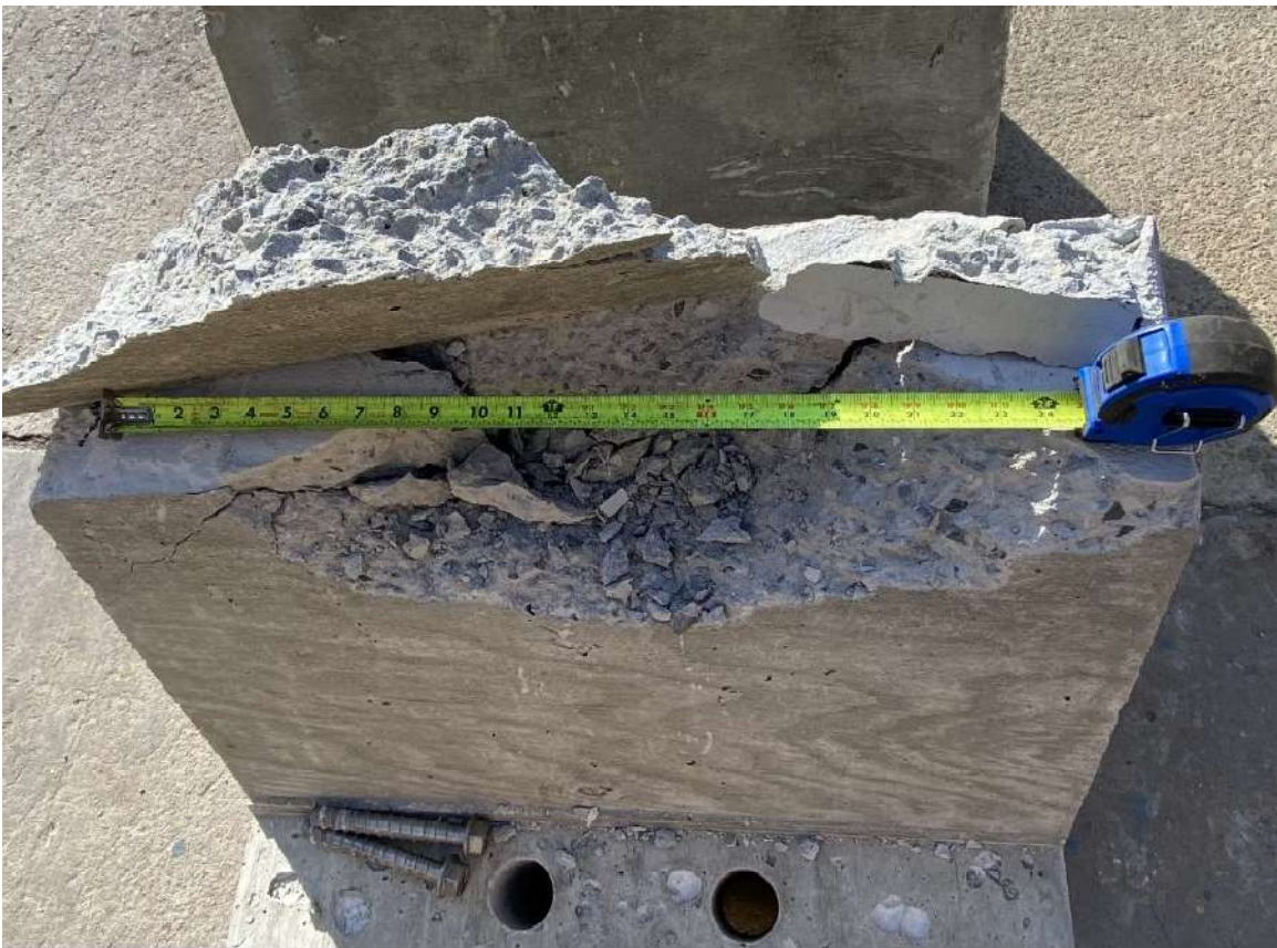
Figure A-80: G-G-2 specimen concrete after screw anchor breakout
