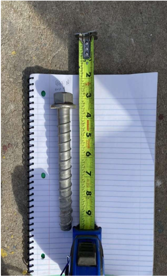
Figure A-81: G-G-3 specimen north screw after breakout
