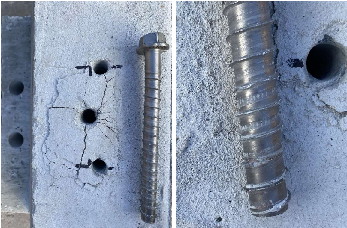
Figure A-29: P-G1-1 specimen screw after breakout
