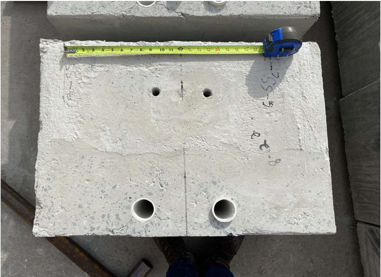
Figure A-64: G-SSc-3 specimen concrete after cyclic loading
