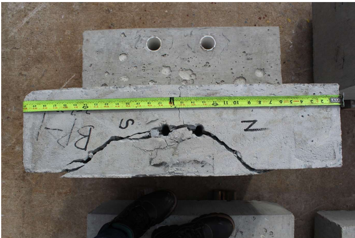
Figure A-97: B-P-1 specimen concrete after breakout
