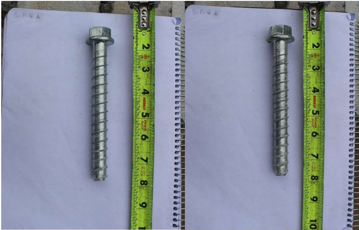
Figure A-102: B-P-4 specimen north and south screw anchor after breakout
