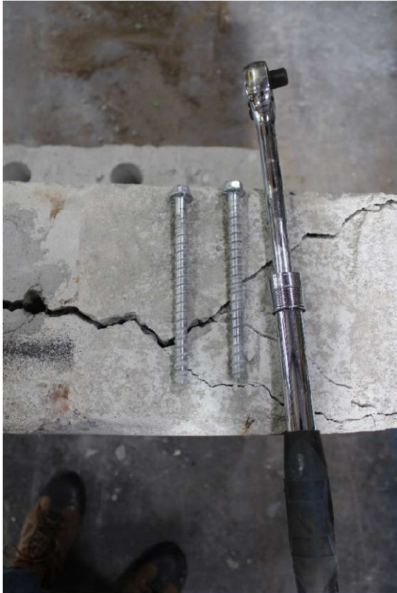
Figure A-121: G-G-38 specimen north and south screw anchor after breakout
