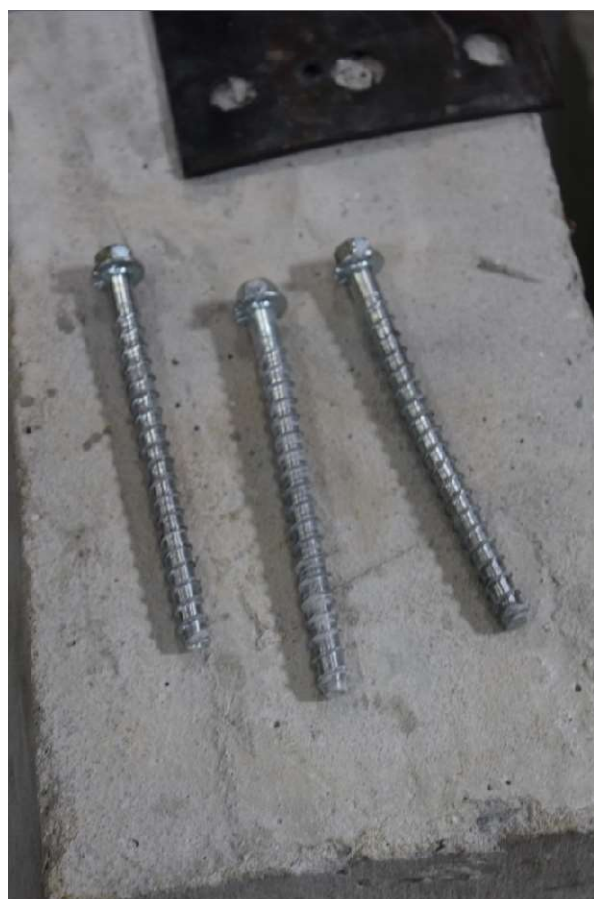
Figure A-123: G-G-310 specimen screw anchors after breakout
