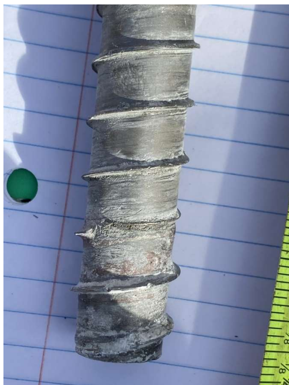
Figure A-82: G-G-3 specimen south screw after breakout
