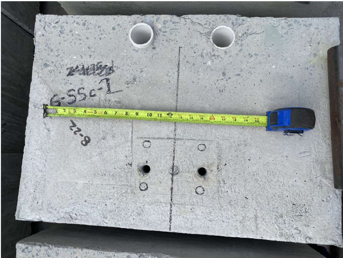
Figure A-61: G-SSc-2 specimen concrete after cyclic loading
