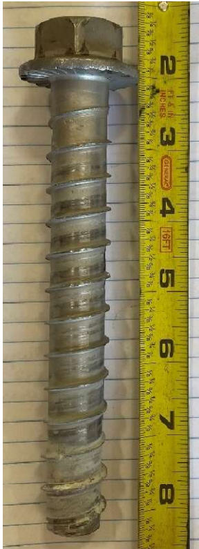
Figure A-47: G-SS-2 specimen south screw after loading
