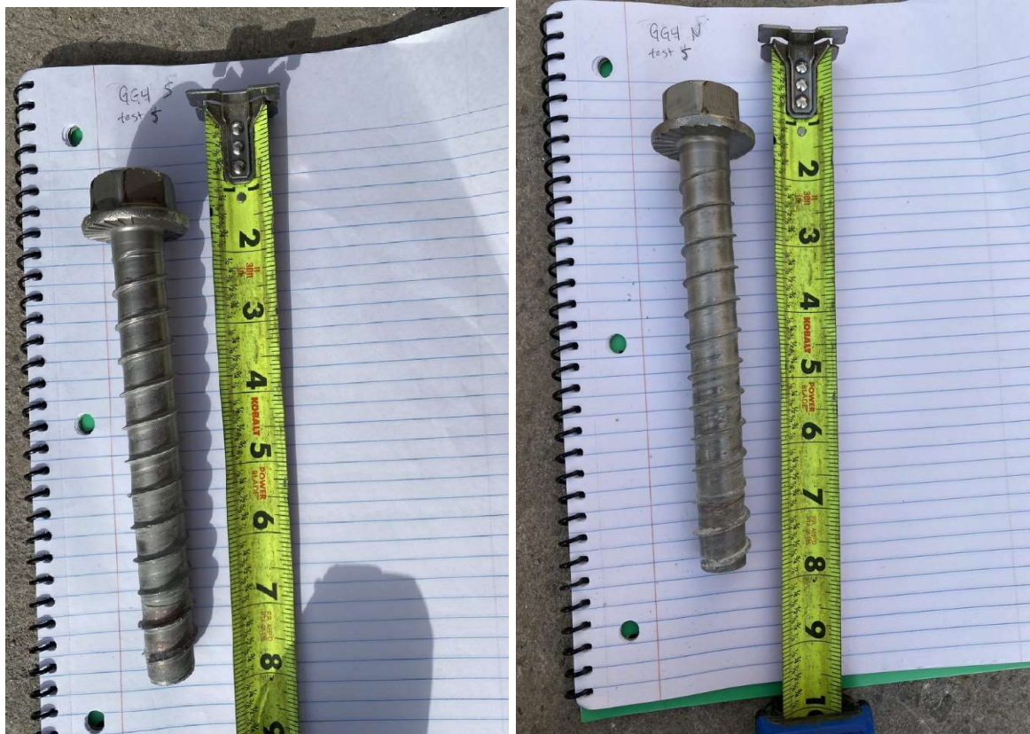
Figure A-84: G-G-4 specimen south and north screw after breakout
