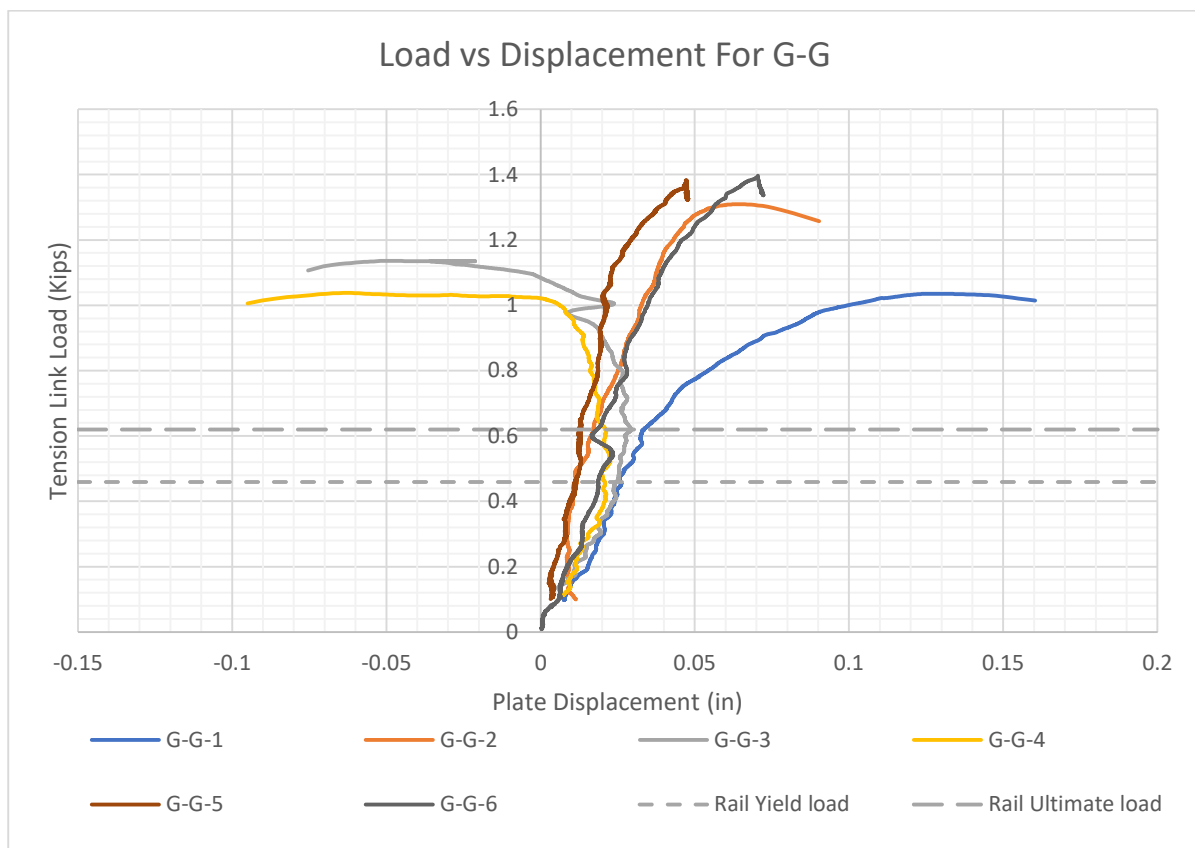
Figure A-68: Relation between load and displacement for G-G
