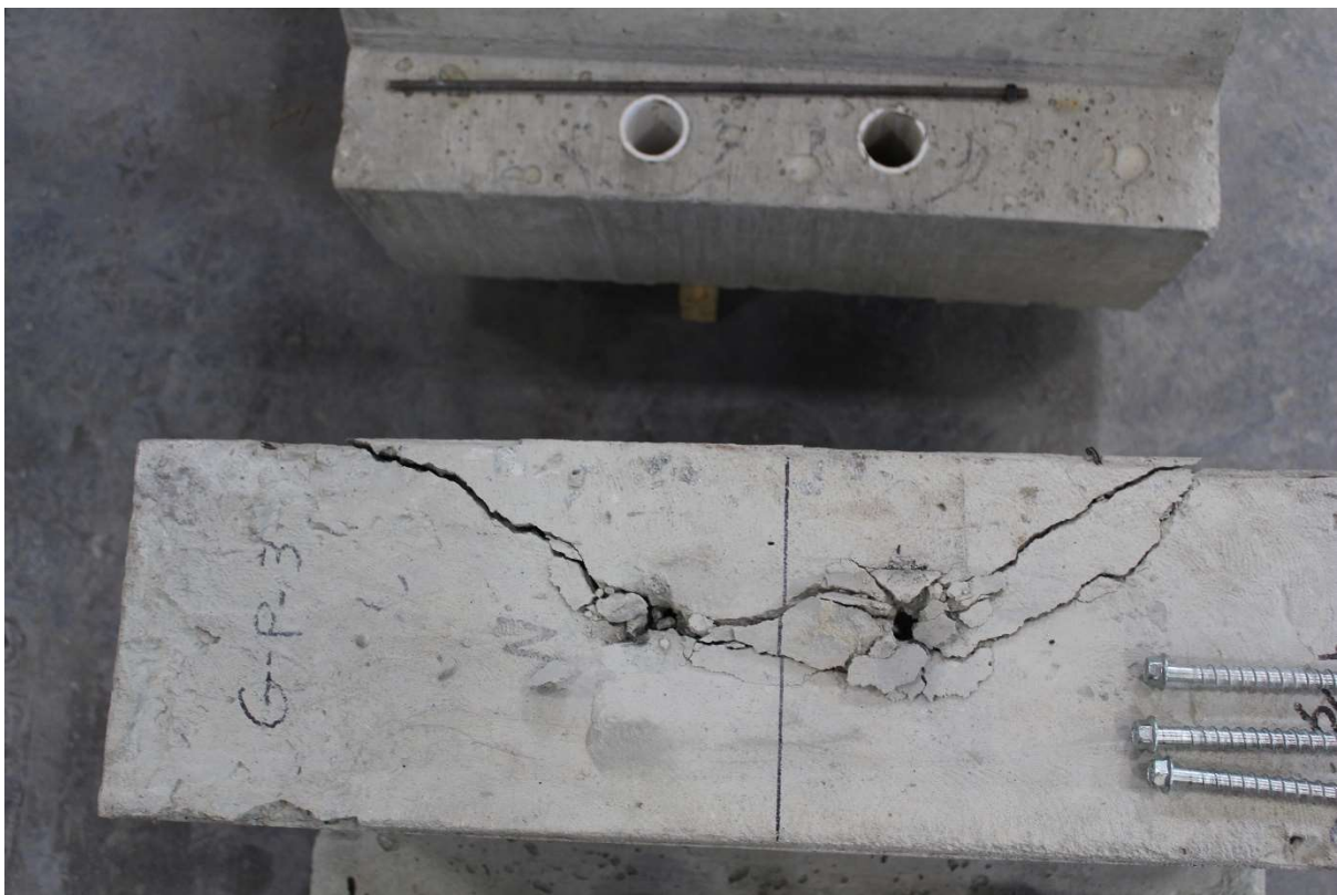
Figure A-126: G-G-312 specimen concrete after breakout
