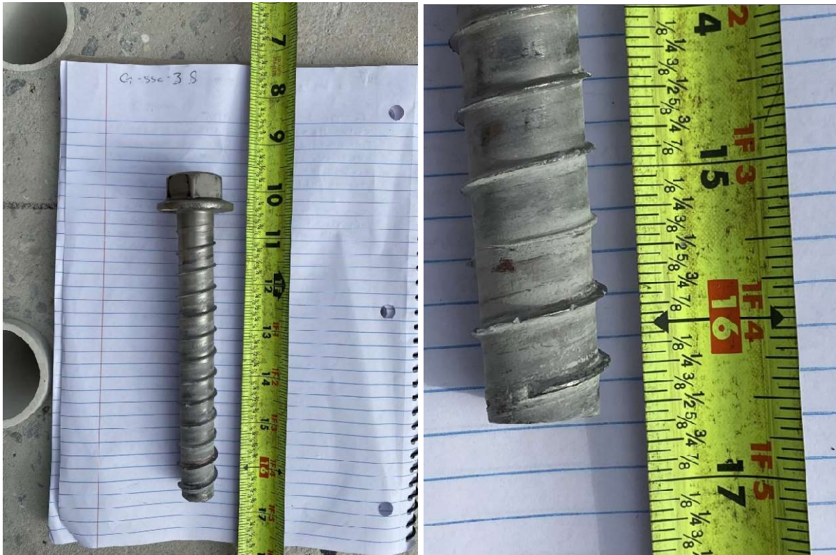
Figure A-63: G-SSc-3 specimen south screw after cyclic loading
