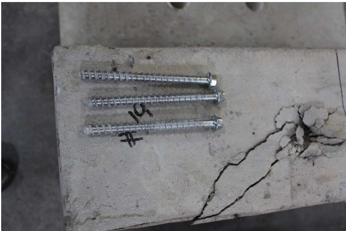
Figure A-127: G-G-312 specimen screw anchor breakout
