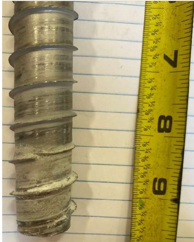
Figure A-47: G-SS-2 specimen south screw after loading
