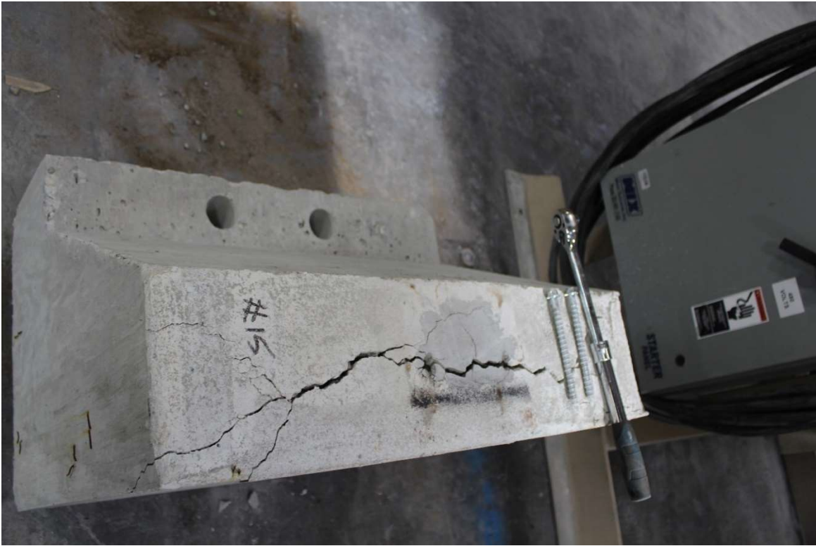
Figure A-120: G-G-38 specimen concrete after breakout
