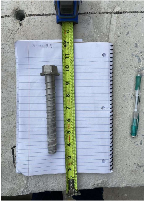
Figure A-65: G-SSc-4 specimen north screw after cyclic loading
