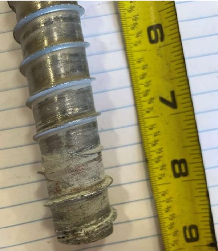
Figure A-48: G-SS-2 specimen north screw after loading
