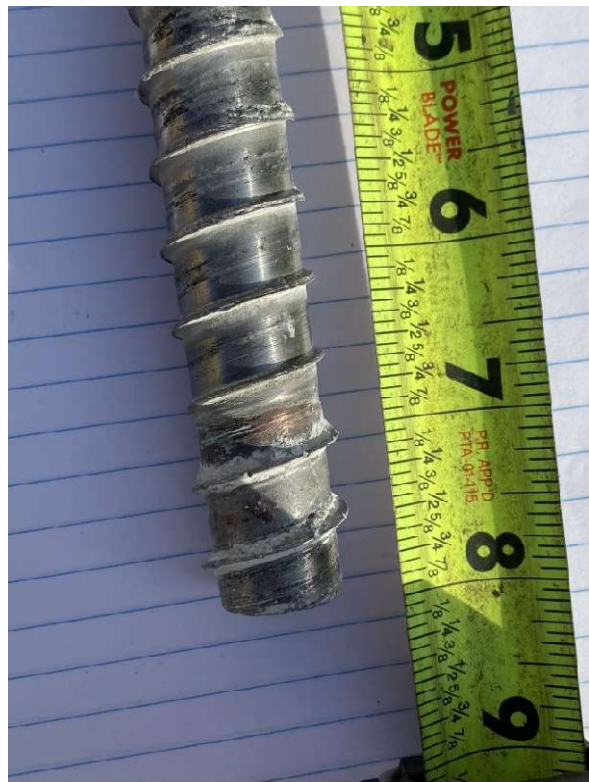
Figure A-76: G-G-1 specimen south screw after breakout
