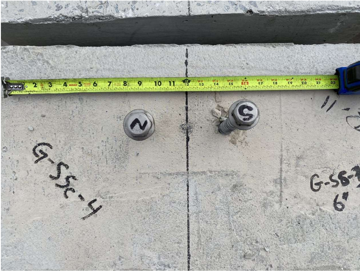
Figure A-67: G-SSc-4 specimen concrete after cyclic loading
