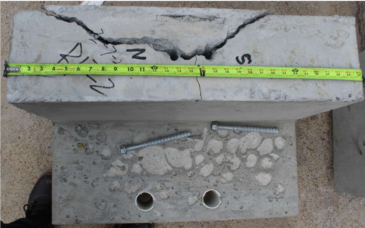
Figure A-99: B-P-2 specimen concrete after breakout
