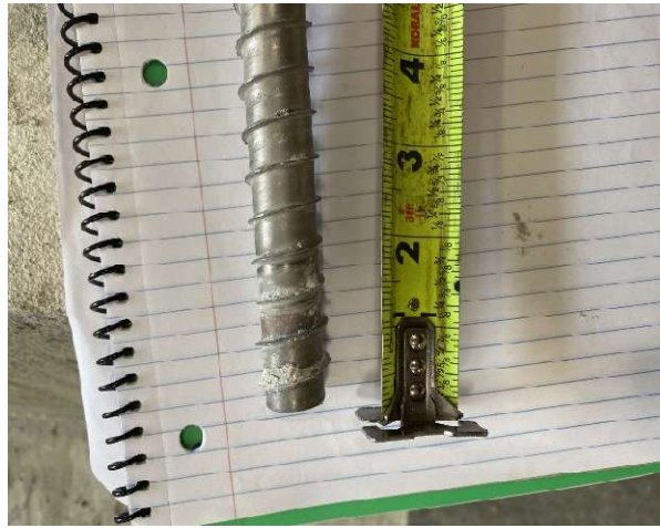
Figure A-79: G-G-2 specimen south screw after breakout
