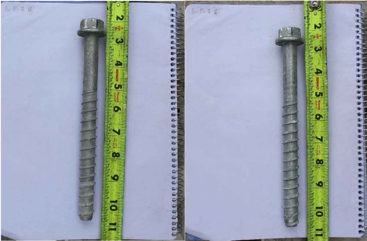
Figure A-98: B-P-2 specimens north and south screw anchors after breakout
