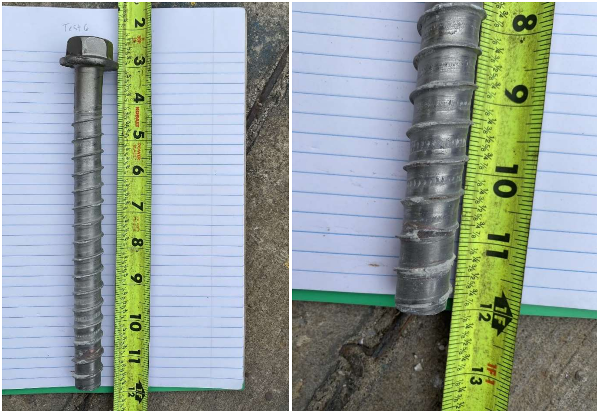
Figure A-19: P-SE1c-1 specimen screw after cyclic loading
