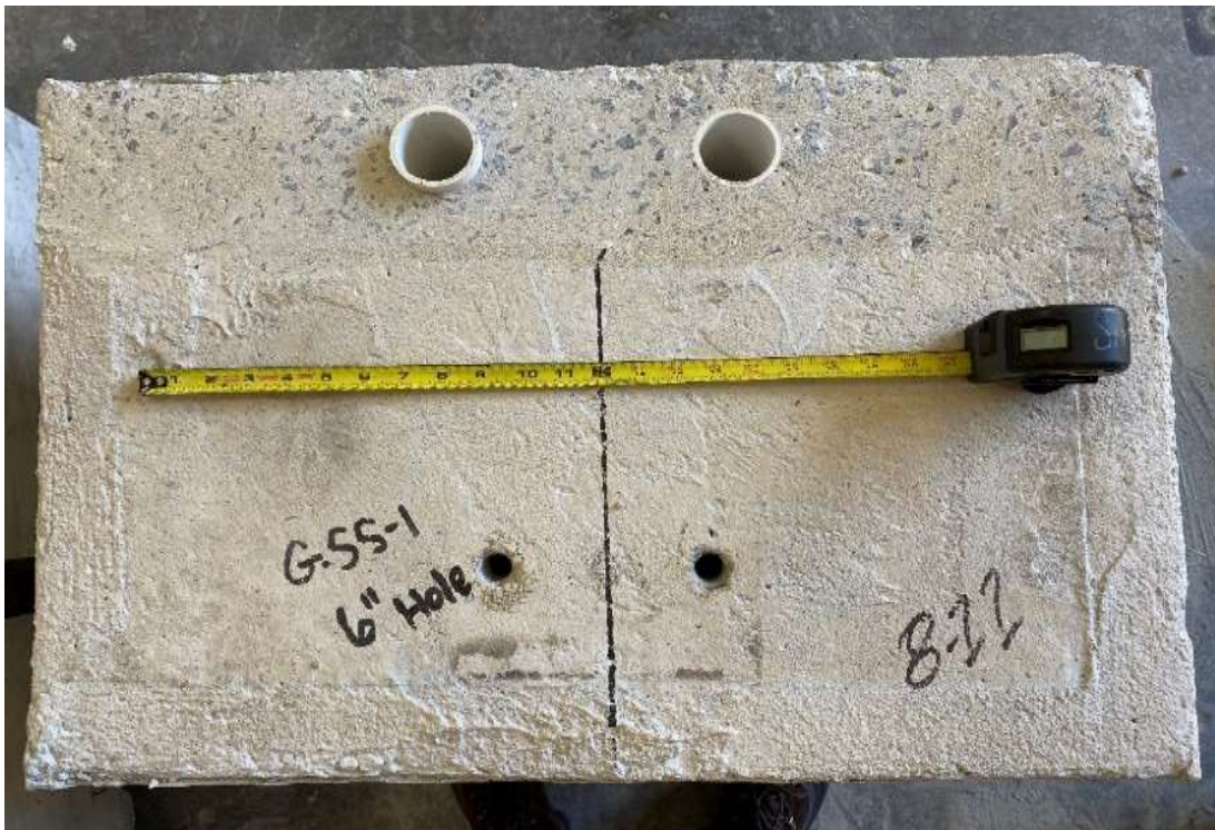
Figure A-46: G-SS-1 specimen concrete after loading
