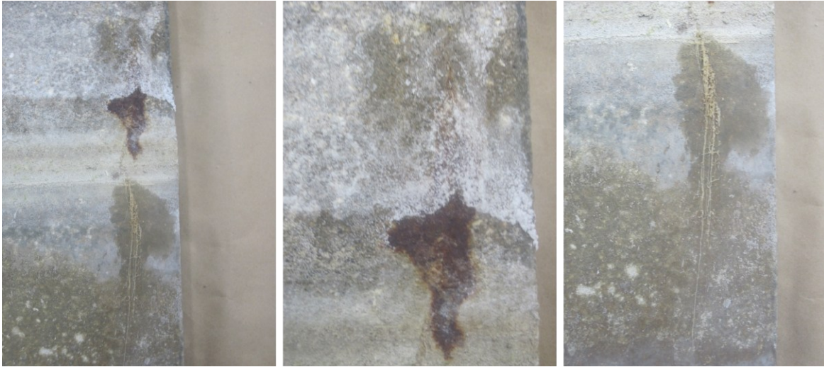
Figure 8-7. Front side of sample STD3-SMI-D before termination.
