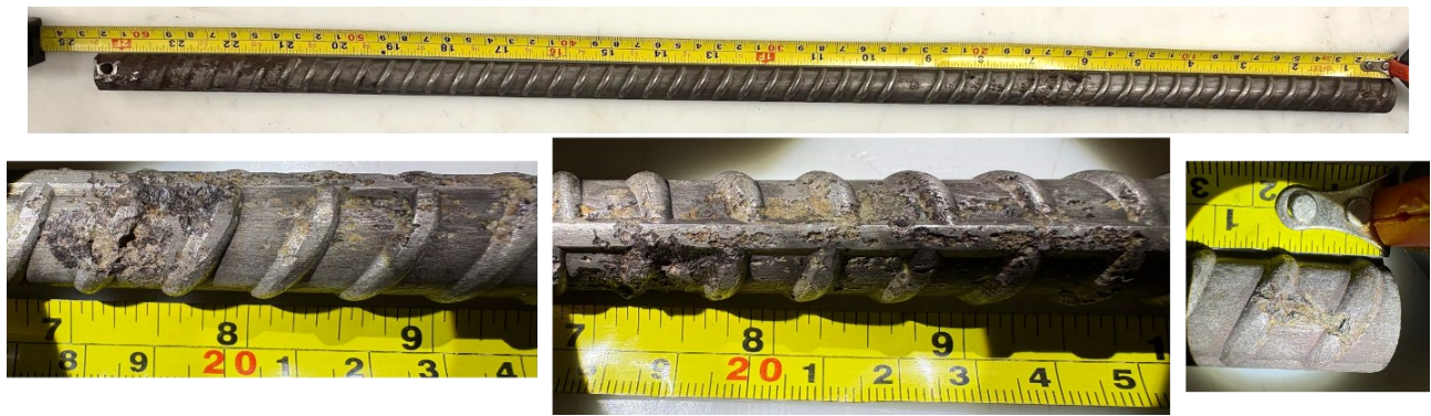
Figure 8-50. STD3-MMFX-B - full length of rebar 1 and notable areas of corrosion damage.
