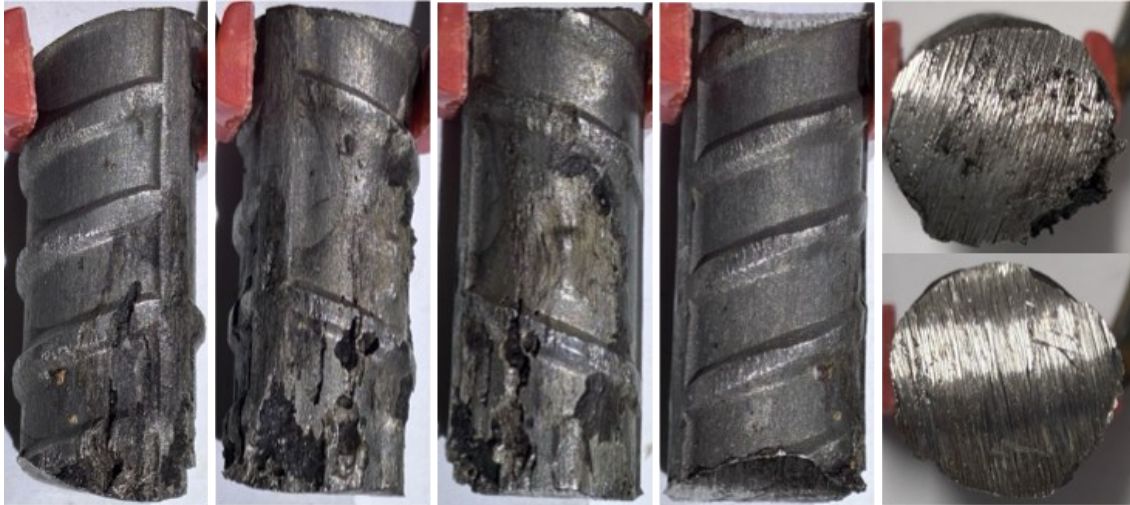
Figure 5-47. 2101 rebar section (Column A) after additional immersion in cleaning solution.
