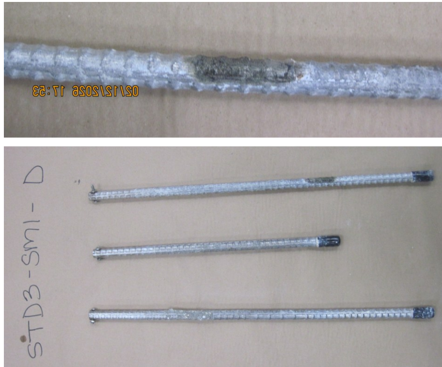
Figure 8-25. All rebars and close up image of corrosion spot on rebar 3 of sample STD3-SMI-D.
