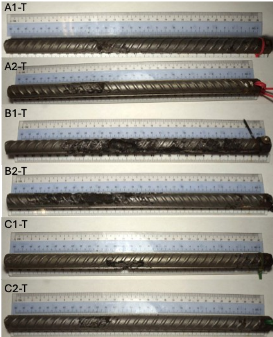
Figure 7-23. 4-CCRV-3CR12-2 top row, top-facing rebars after cleaning.
