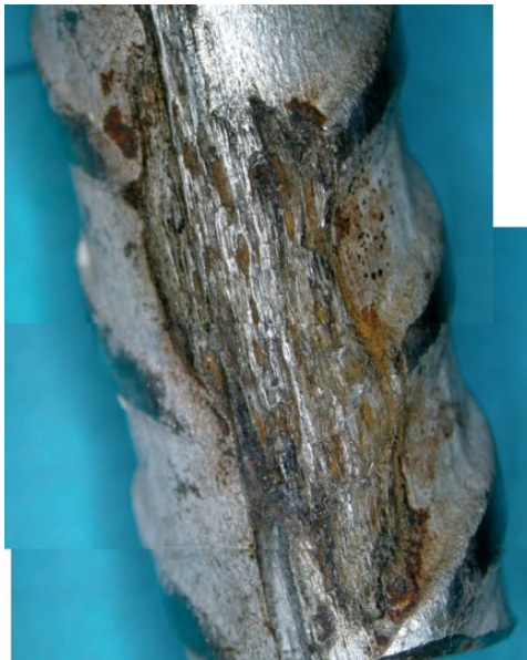
Figure 8-42. Corrosion spot observed on rebar 2 of sample STD3-2304-B.
