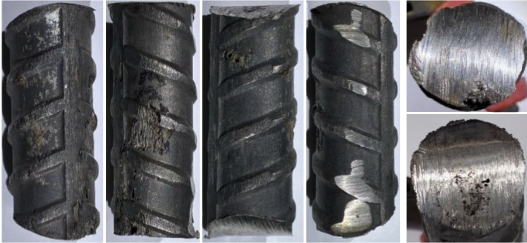
Figure 5-49. 2101 rebar section (Column B) after additional immersion in cleaning solution.
