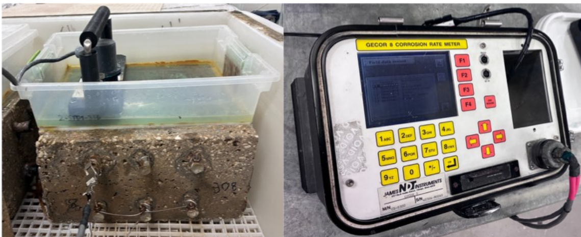
Figure 2-2. Gecor 8 Sensor C measuring Rebar A of an SDS sample (left); Gecor 8 device (right).
