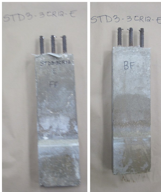
Figure 8-8. Front and back side of sample STD3-3CR12-E before termination.
