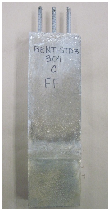
Figure 8-5. Front side of sample BENT-STD3-304-C before termination.
