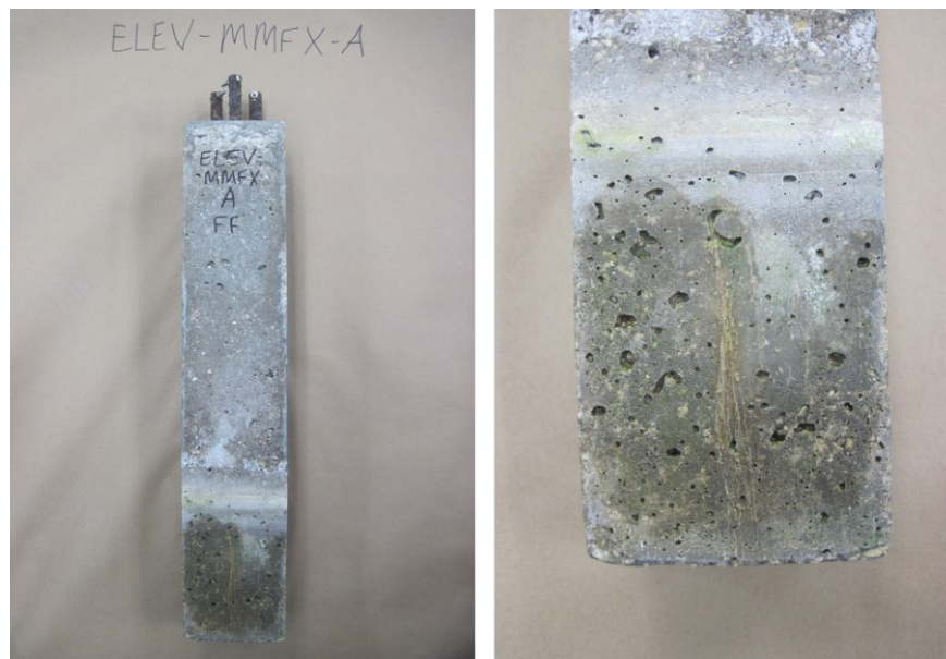
Figure 8-12. Front side of sample ELEV-MMFX-A before termination.
