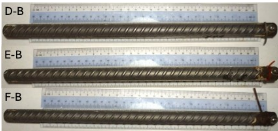
Figure 7-26. 4-CCRV-3CR12-2 bottom row, bottom-facing rebars after cleaning.
