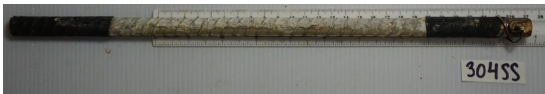
Figure 7-20. Bottom-facing side of 304SS rebar before cleaning, showing some corrosion.
