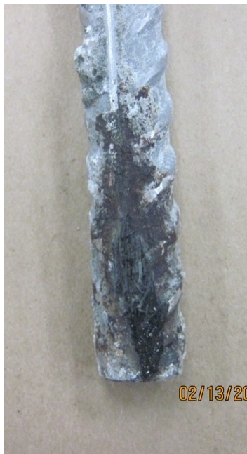
Figure 8-20. Close up corrosion spot on rebar 2 of sample STD-2304-B.
