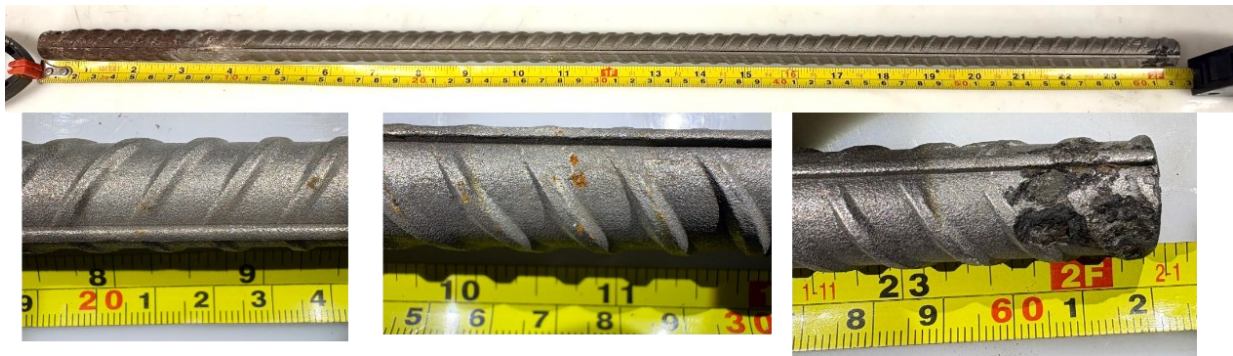
Figure 8-48. STD3-3CR12-E - full length of rebar 1 and notable areas of corrosion damage.
