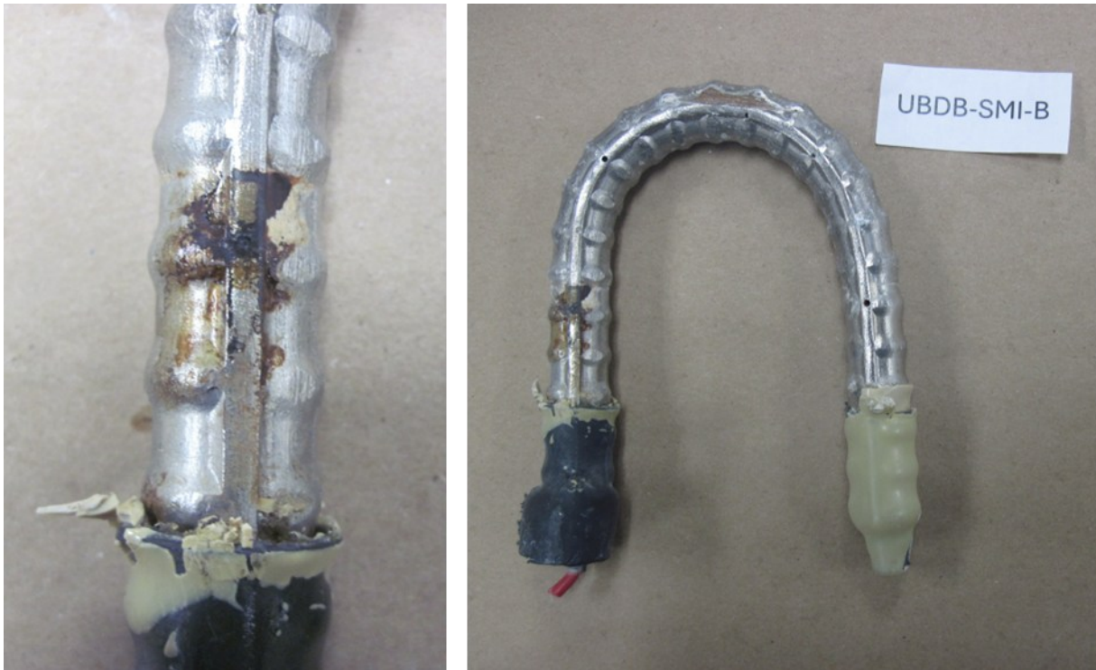
Figure 8-38. Corrosion spots on bottom side of sample UBDB-SMI-B (G109).
