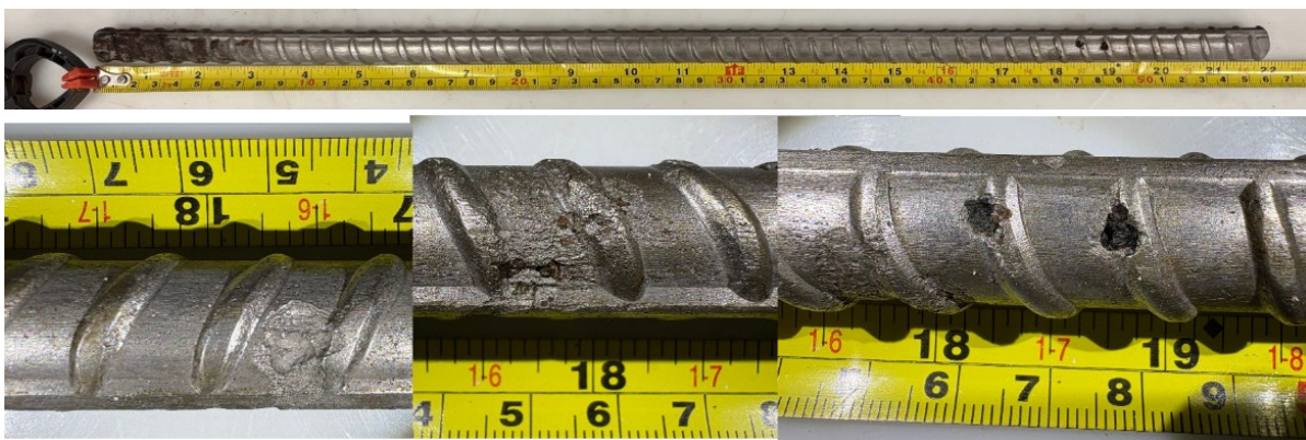
Figure 8-54. ELEV-MMFX-A - full length of rebar 2 and notable areas of corrosion damage.
