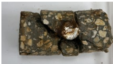
Figure 5-31. Image shows the core obtained from column 2101-B (~6 inches below WL).
