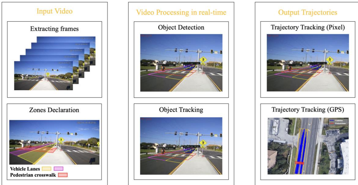
Figure 4 Overall video processing stages for trajectories extraction
