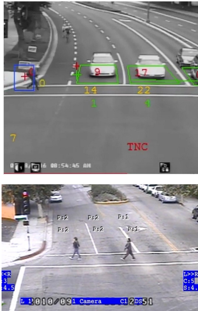
Figure 3-2. Sample display of an automated pedestrian detection system
