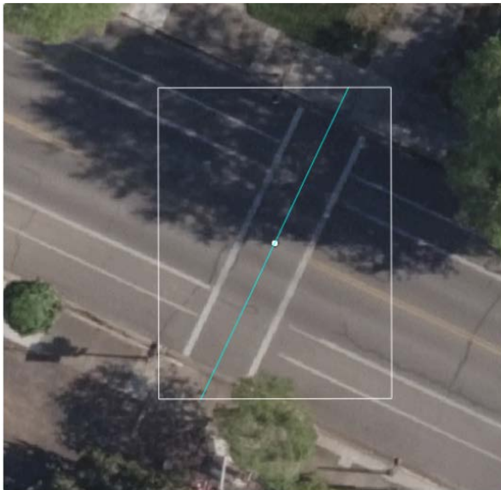
Figure 4-8. Crosswalk element displaying bounding box polygon, bounding box centroid point, and crossing distance (line string)
