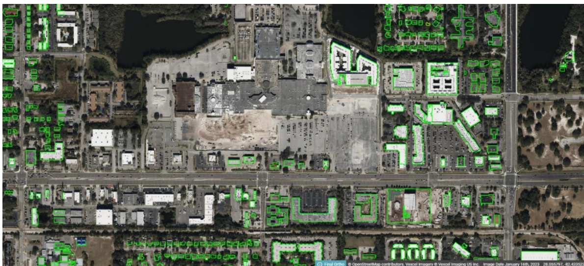
Figure 7-4. High-resolution aerial imagery with object detection and land use analysis from Vexcel platform
