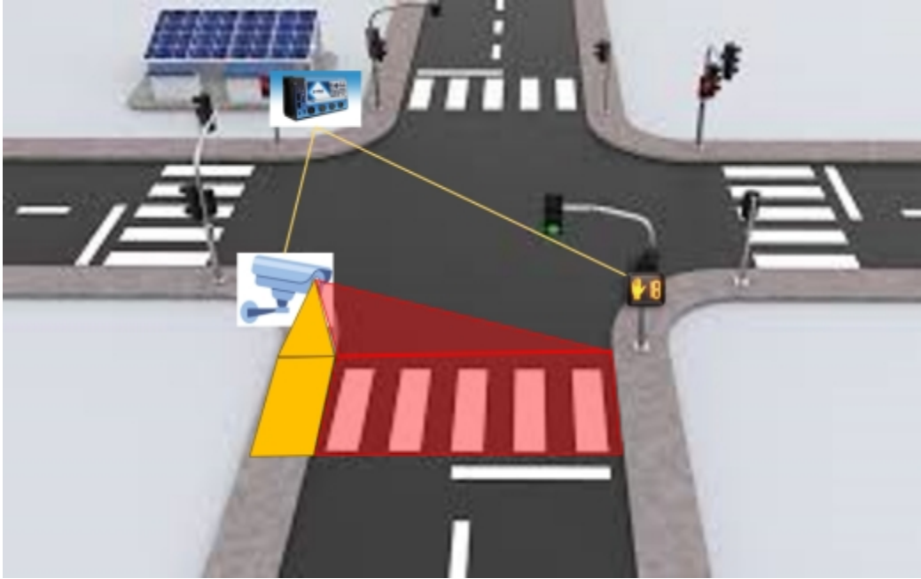
Figure 3-1. Schematic of the automated pedestrian detection system
