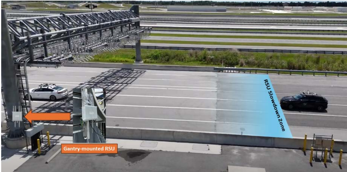
Figure 4-16: RSU slowdown zone marked onto east straight of test location.
