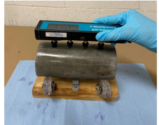
A concrete sample surface resistivity is measured according to AASHTO T 358. In this method, the probe is placed on the sample surface at 0 degrees to measure the concrete surface resistivity then rotated with the probe being placed on the line 90 degrees to the initial line.
