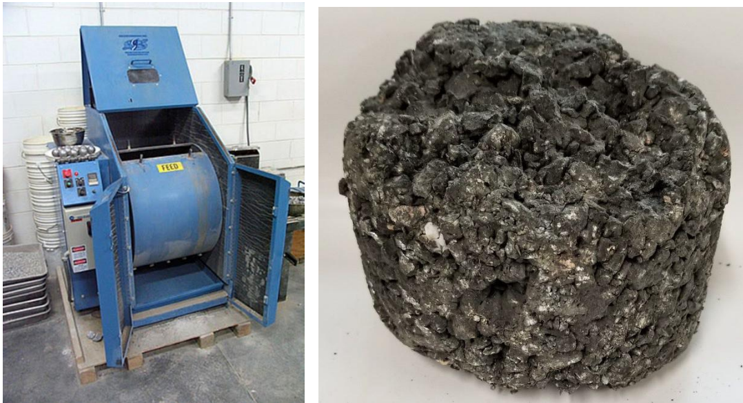
Figure 15. Los Angeles Abrasion Machine Used for Cantabro Testing (left) and FC-5 Specimen after Cantabro Testing (right)
