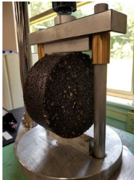
Figure 13. High-Temperature Indirect Tensile Strength Test (HT-IDT)
