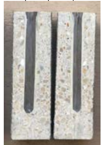
The spike anchor (cross-section shown) is the most common type of CFRP anchor used in Florida.
