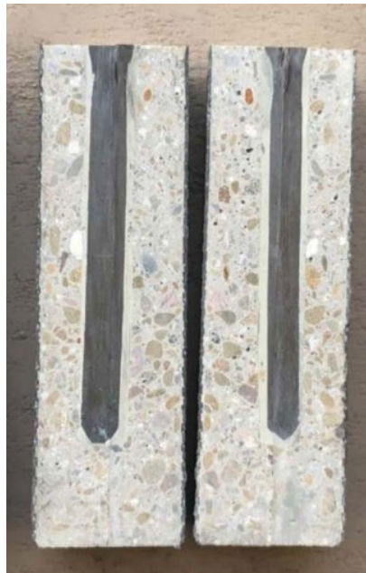
Figure 2: Spike anchor cross-section (Castillo and Kanitkar, 2021)
